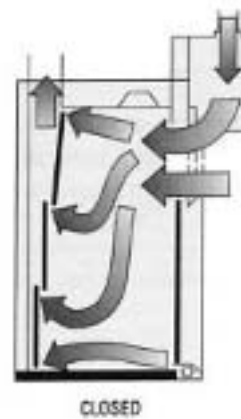
▼ Auxiliary air fume hood with constant volume exhaust systems. Courtesy Fisher Hamilton.
