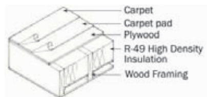
Figure 4-11. (EN12) Floors, wood frame.
