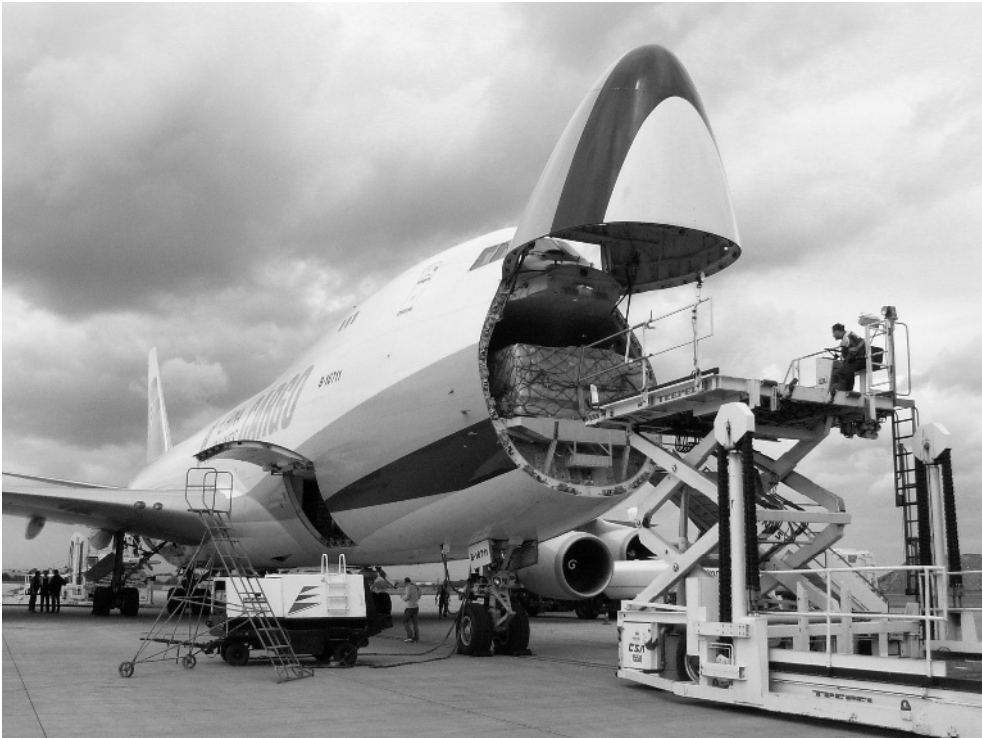
Figure 11-1 Front loading reduces the handling costs (Photo: Courtesy CSA Cargo)
