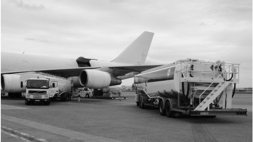
Figure 10-4 B-747 refuelling requires sometimes more than one tanker (Photo: A. Kazda)
