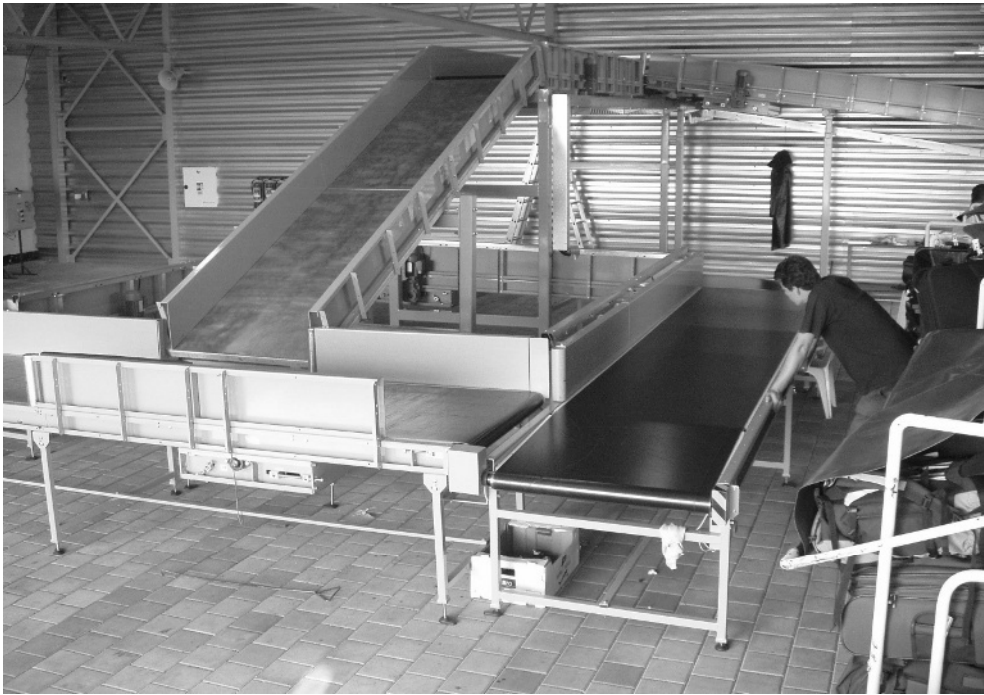
Figure 12-8 For small airports simple manual sorting system is sufficient – Brno Airport (Photo: A. Kazda)
