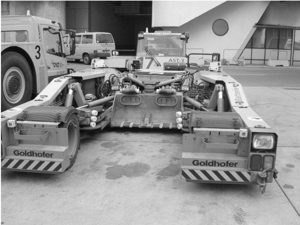
Figure 9-8 Heavy Goldhofer towbarless tractor (Photo: A. Kazda)
