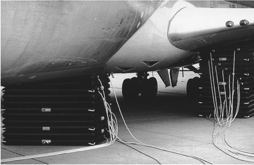
Figure 19-10 Lifting of aircraft by special air bags (Source: Vepro company)
