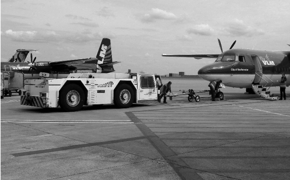
Figure 9-6 A towbar tractor being connected to an aircraft (Photo: A. Kazda)
