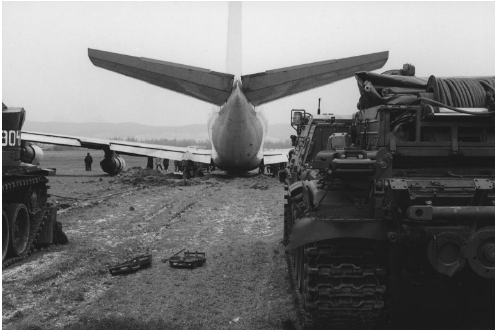
Figure 19-8 The airplane recovery after runway end overrun (Photo J. Mach)
