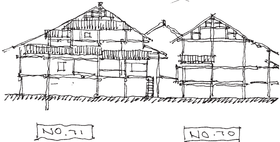
Figure 4.15 Dong house elevation showing the use of short queen posts. Source: Fieldwork sketch by Xing Ruan, 1993.
