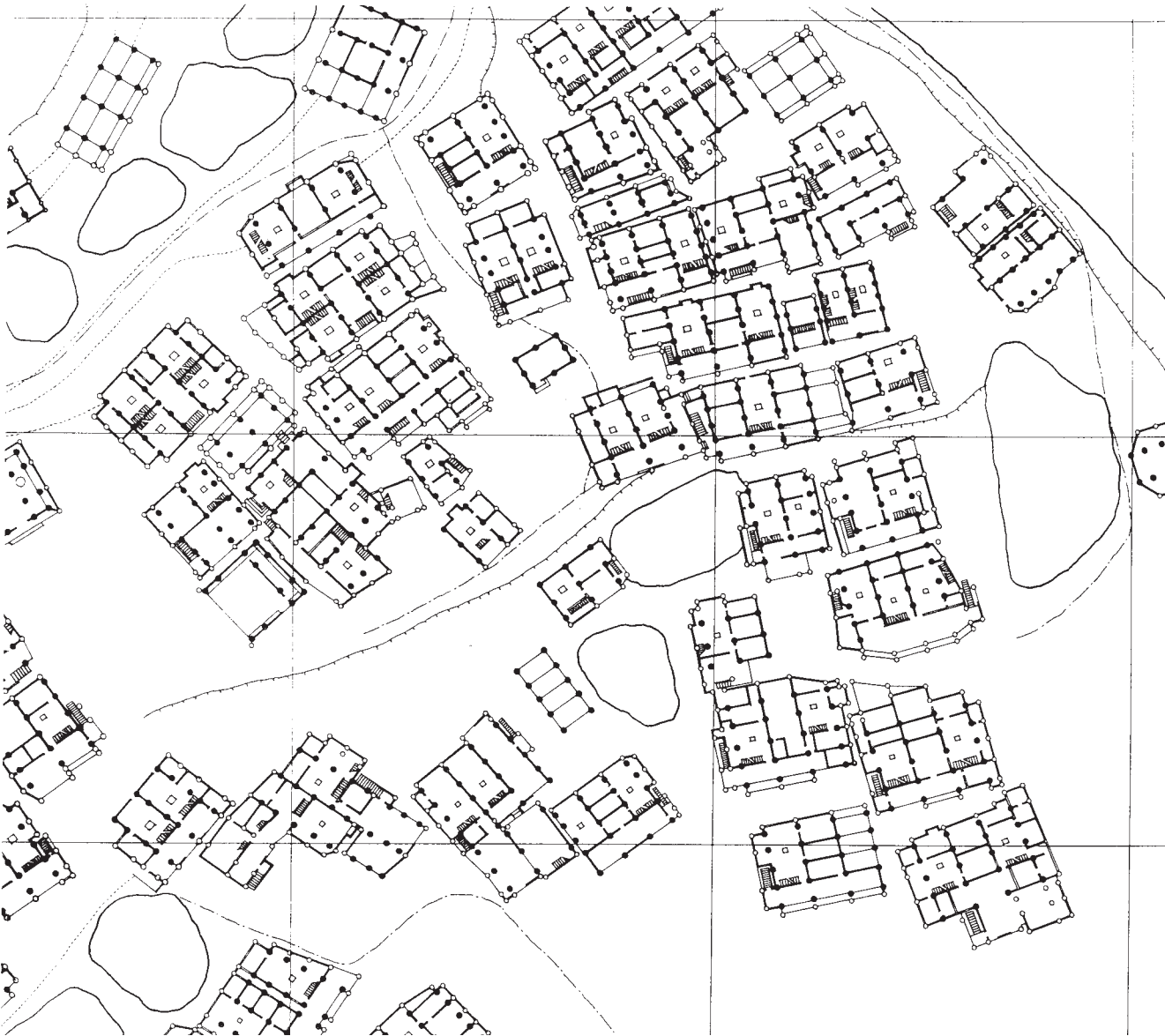
Figure 4.16 Plan fraction of Dong dwellings in Ma'an village, Sanjiang region, Guangxi province, showing the flexible additions attached to the main structural frame. Source: Drawn by Dongmin Zhao and Xing Ruan.
