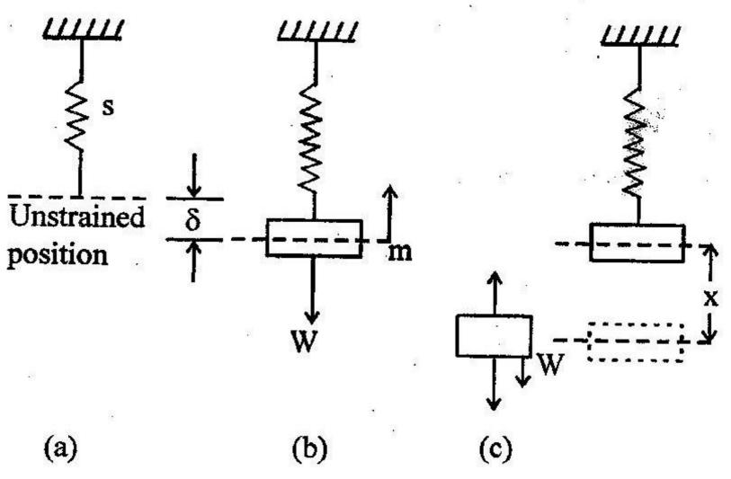
Show that the natural frequency of longitudinal vibration of the system is:
