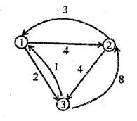
(e) Consider the graph shown below and find the shortest path using the Floyd-Warshall algorithm.
