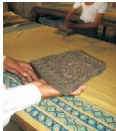
Figure 2.25 Block printing process
