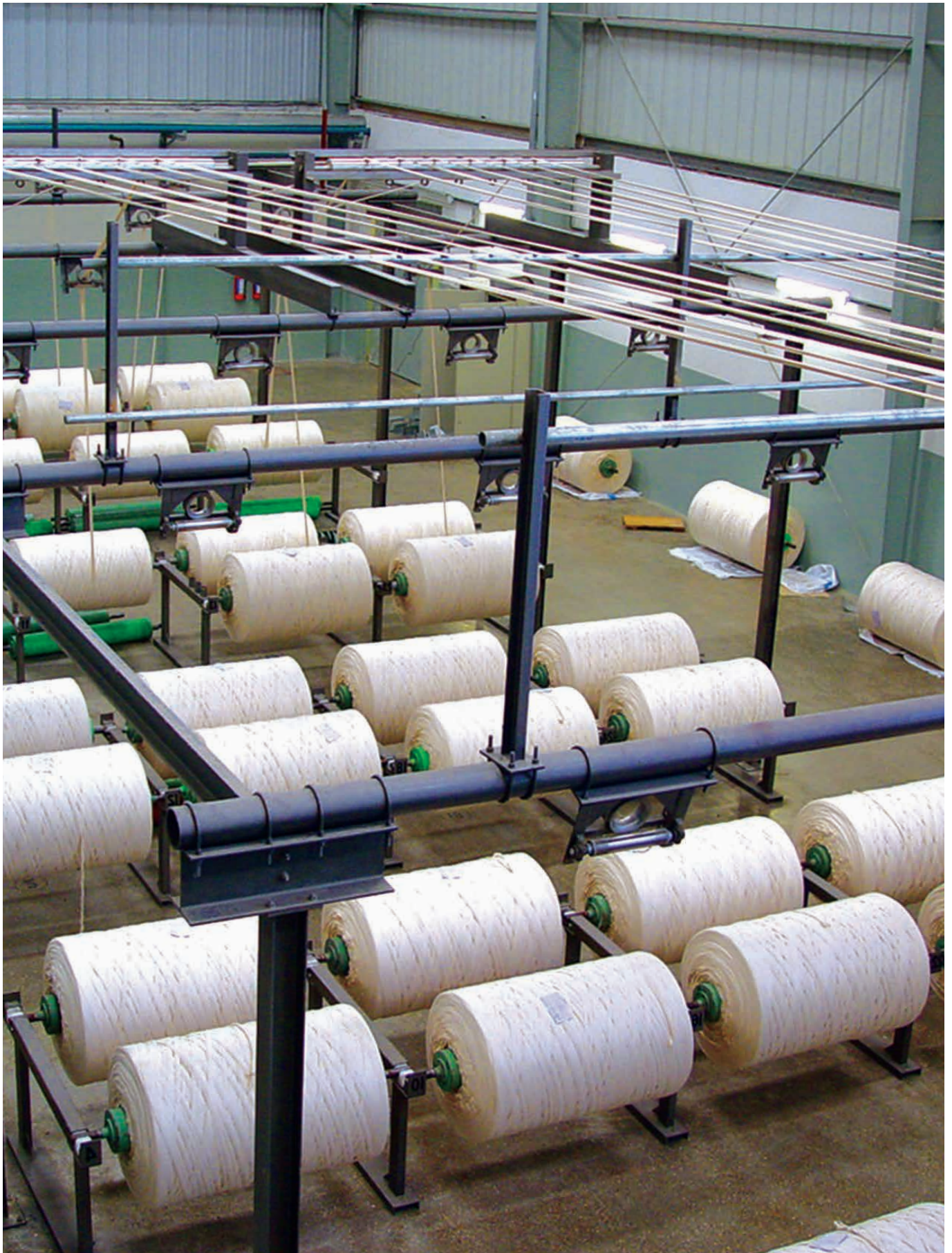
Ball warp in rope form ready to dye
