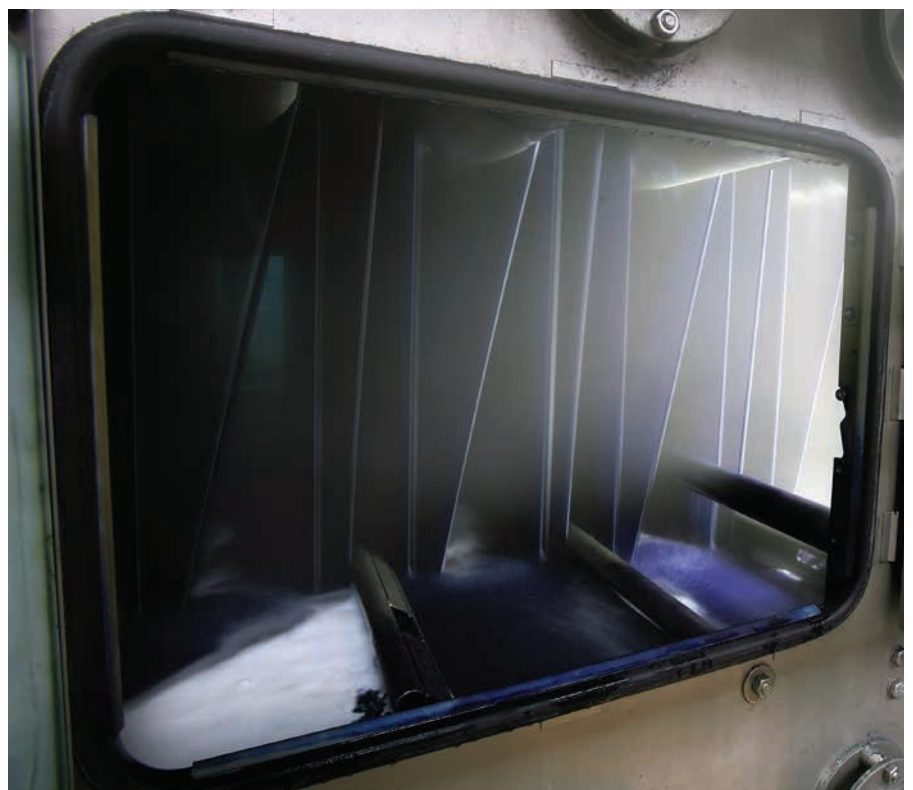
Washing vat after desizing. The fabric circulates thanks to a series of submerged cylinders
