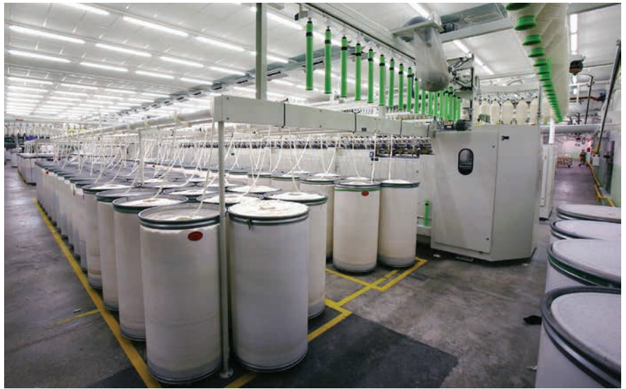
Accumulation of tufts or ropes after coming out of speed frames
