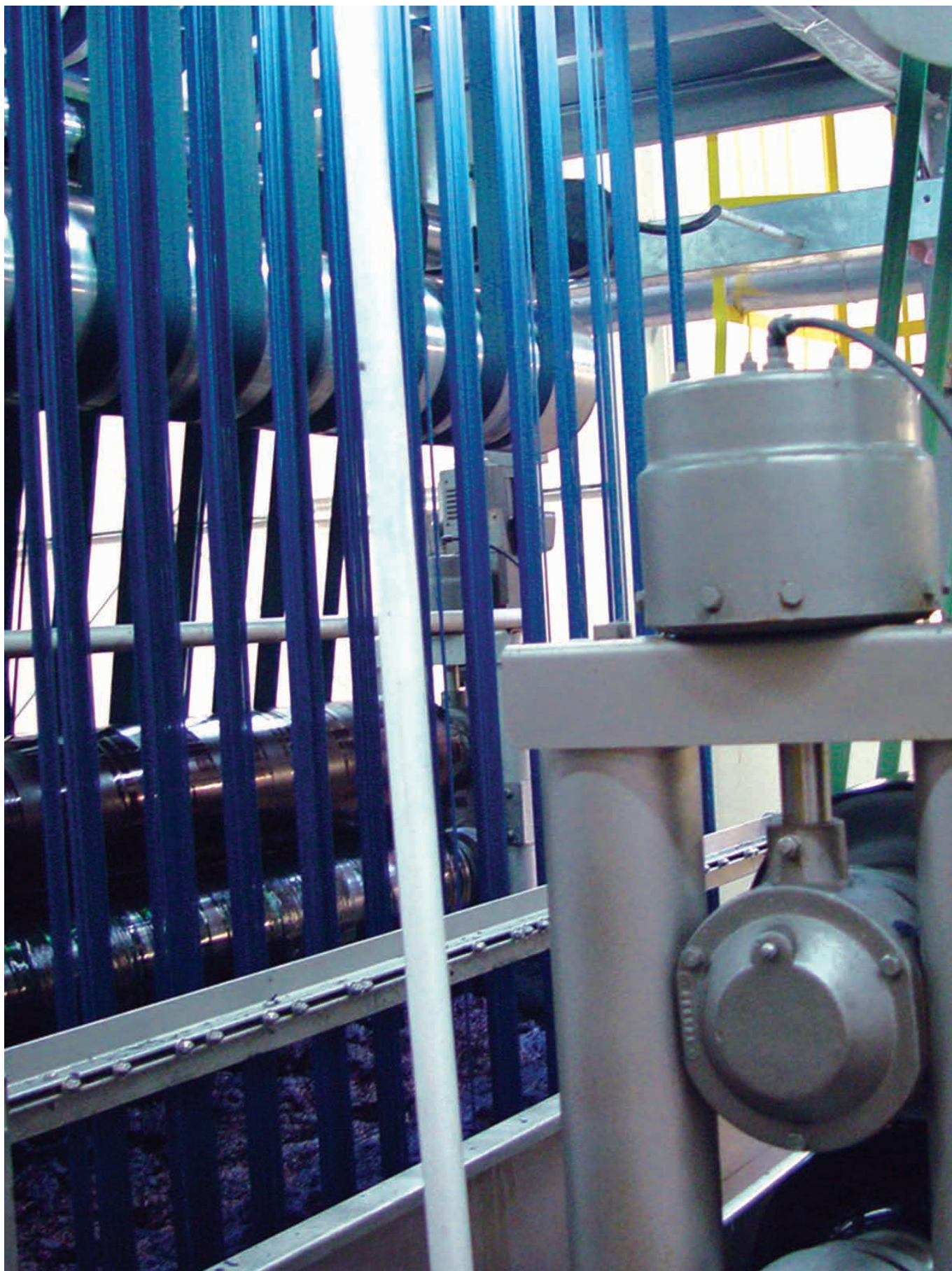
Detail of the colored ropes coming out of an indigo dye vat
