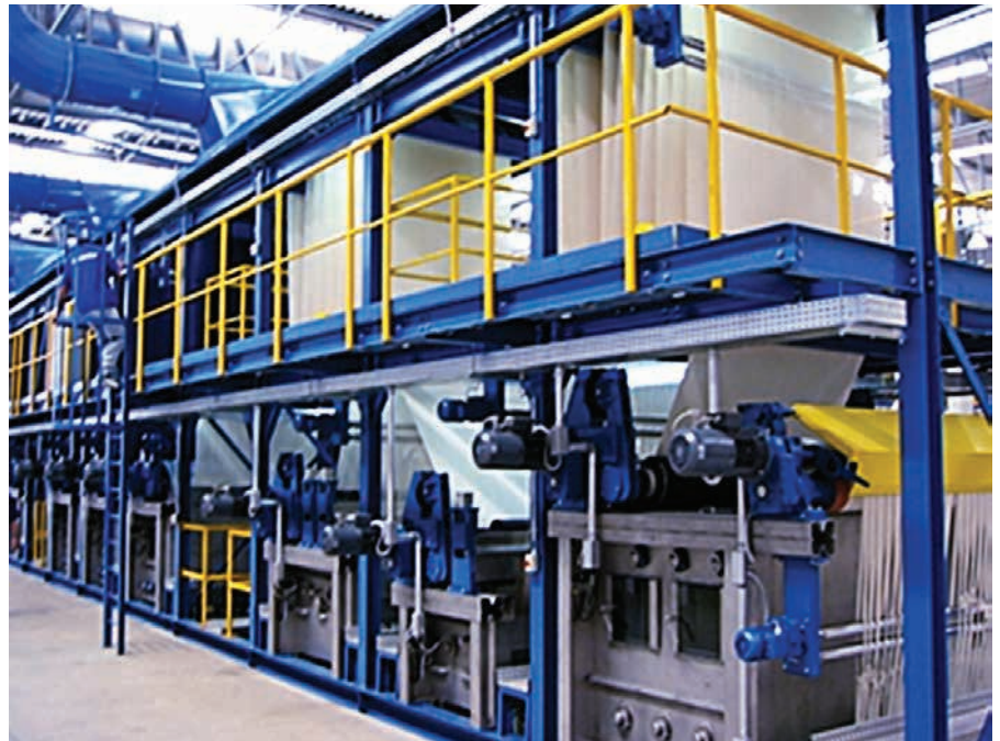
Dyeing range with different vats where both bottoming as well as topping processes are carried out
