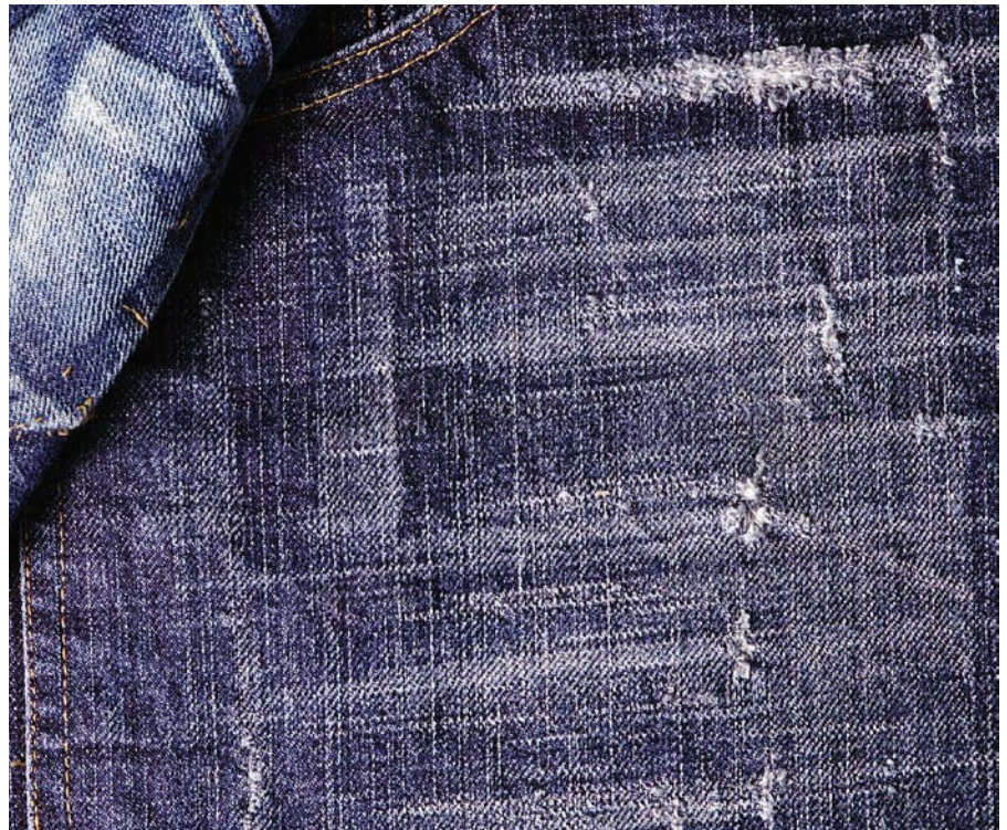
Denim fabric after a bottoming-type application. The initial dyeing performed with a sulfur dye and later with indigo
