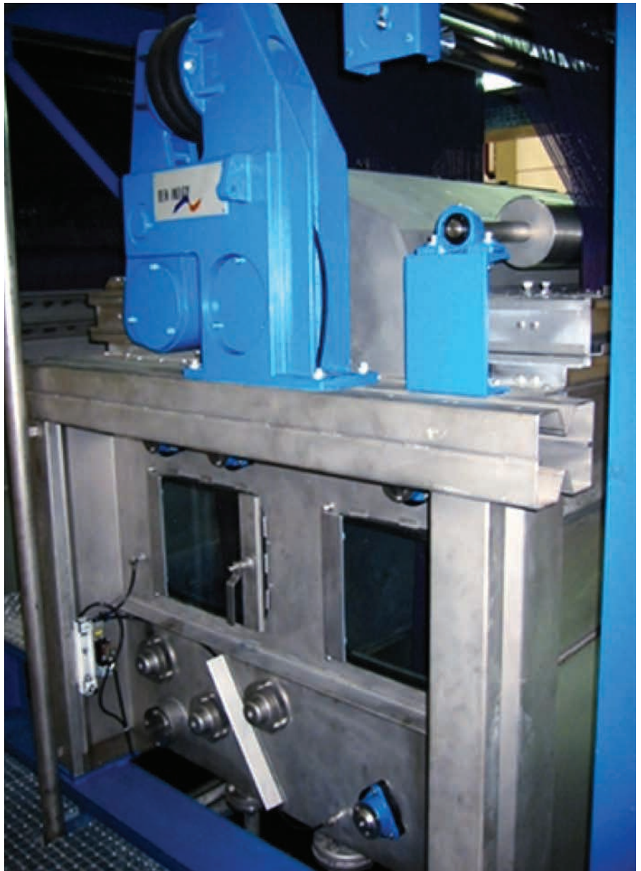
Closed dye vat which can be used for both indigo as well as for sulfur dyes
