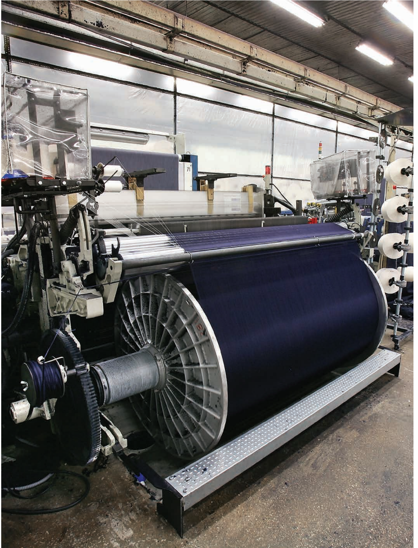
Detail of a beam of colored thread placed in the loom, prepared for the weaving of a plane fabric
