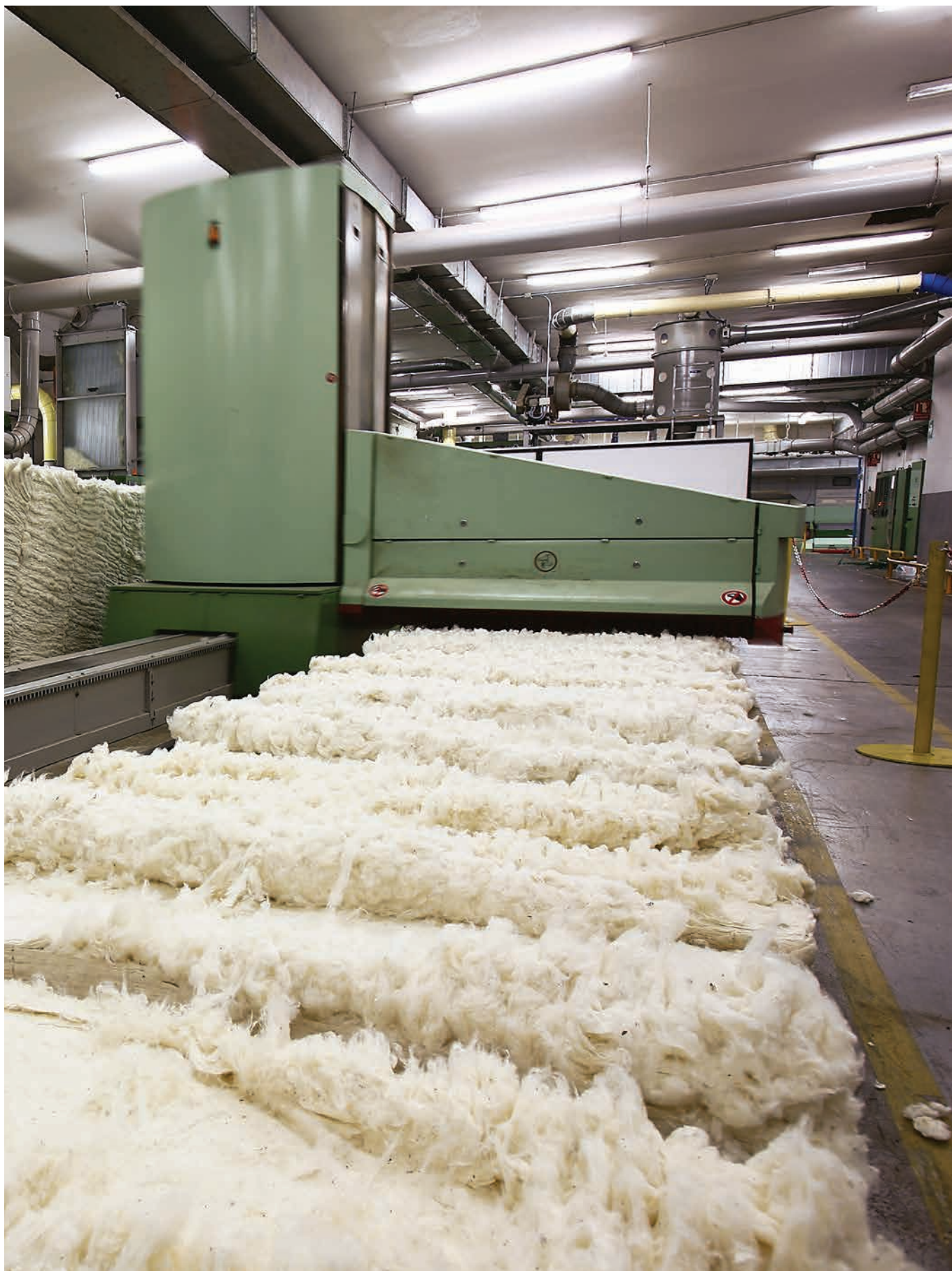
Cotton fibers are mixed in the first phase of yarn formation
