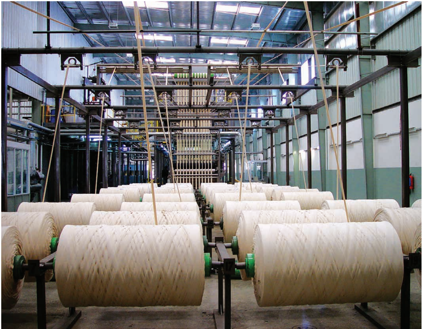
Ropes entering the range from ball warp
