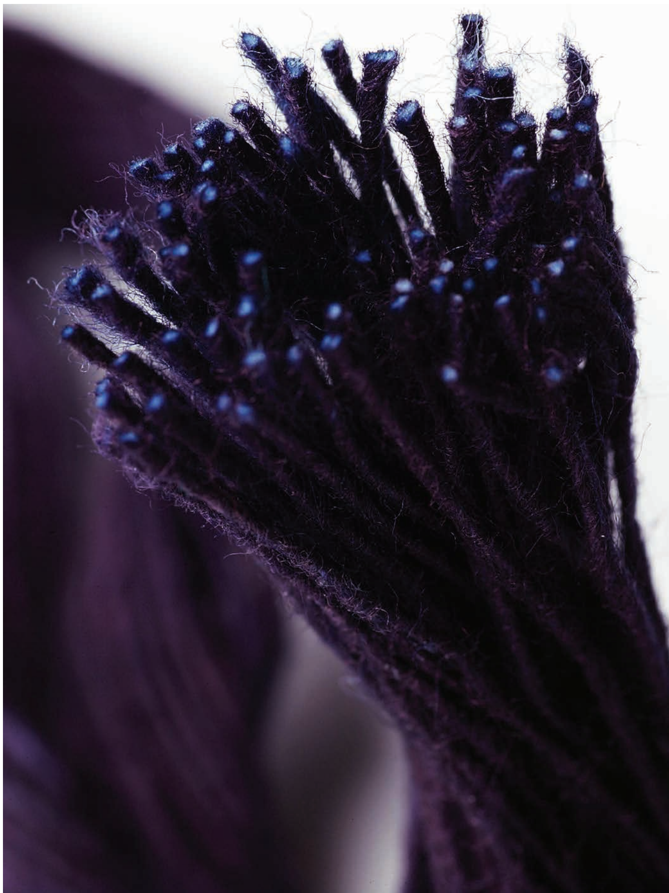
Yarn dyed by using bottoming process
