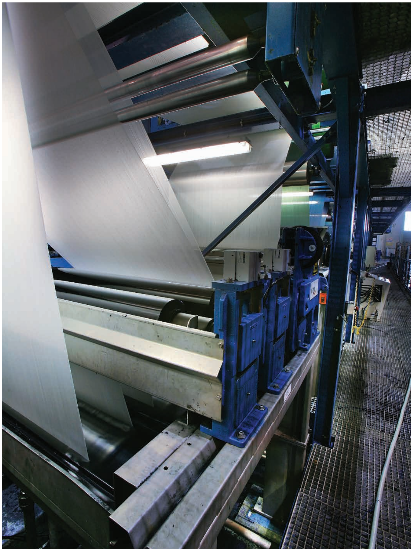
Details of a preparation vat in a slasher type range
