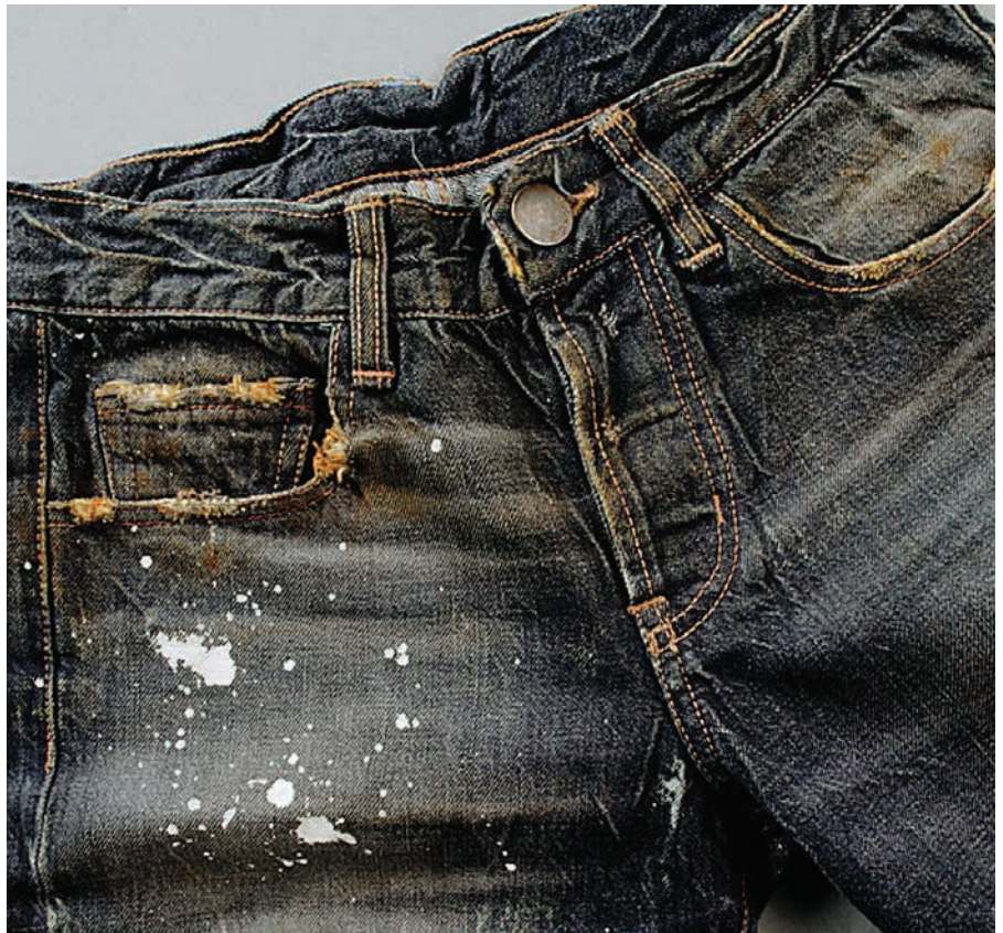
Pigments with resin can be used for local application on jeans in the same way, by being sprayed on or applied with a sponge
