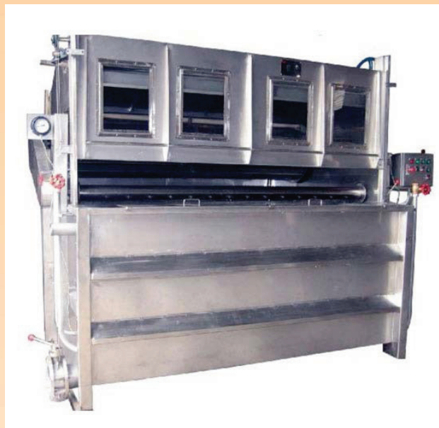
Pic.2.17 Winch Dyeing Machine
