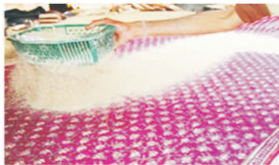
Fig. 49 Saw Dust Sprinkled Over the Resist Paste
