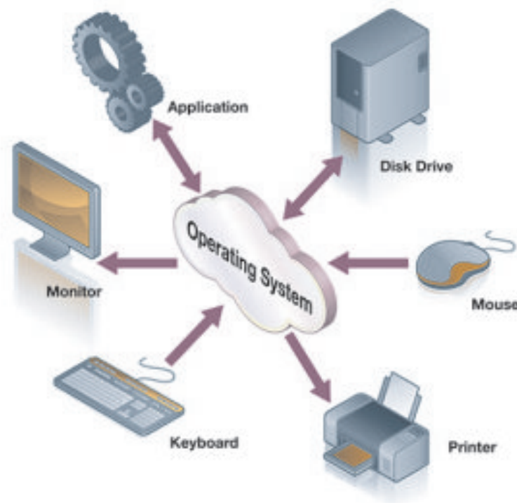
Figure 2.5 Components controlled by an Operating System
