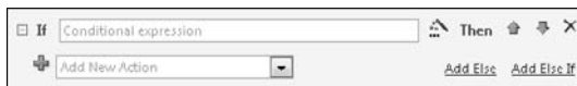
Figure 1-11: The If block is where you type in a condition that controls whether Access performs a set of actions.
