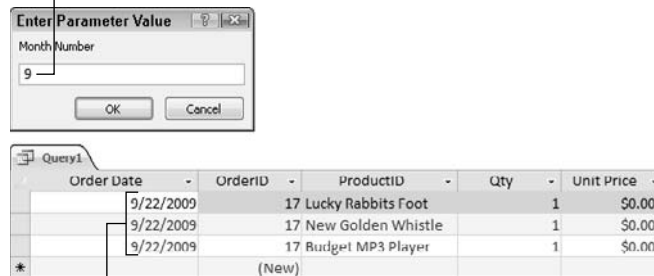
Figure 2-15: The result of opening a parameter query and specifying 9 as the Month Number.
