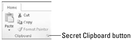
Figure 4-1: The Cut, Copy, and Paste buttons are found in the Clipboard group on the Home tab of the Ribbon.
