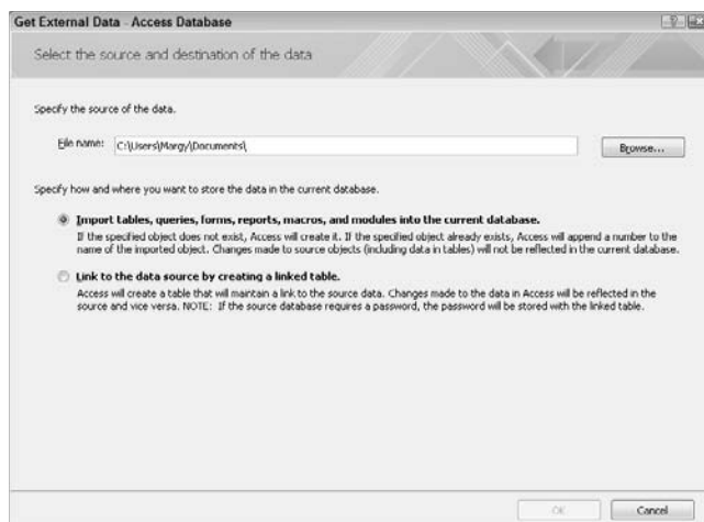
Figure 2-2: Use the Get External Data dialog box to split a database or link to tables in another database.
