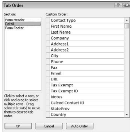
Figure 2-13: Controlling the order in which your cursor moves from field to field on a form.
