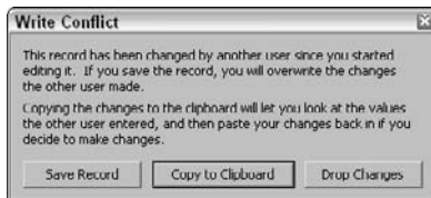
Figure 2-5: Two people are trying to change this record at the same time.
