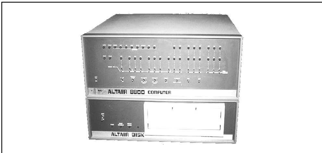
Figure 1-6. The Altair MITS is thought to have been the first personal computer
