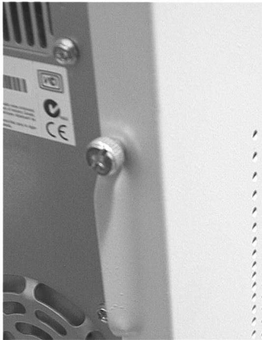
Figure 15-4. A single screw holds on the cover on a single screw case design
