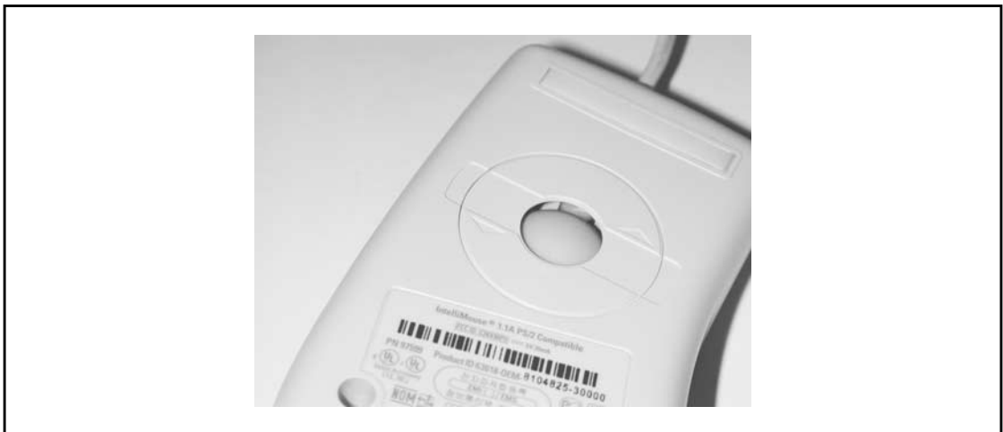
Figure 22-5. A mouse ball is held inside the mouse by a locking cap that can be rotated to release the ball
