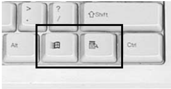
Figure 18-10. The two Windows-specific keys to the right of the SPACEBAR are used to display the Windows Start menu and the current context menu
