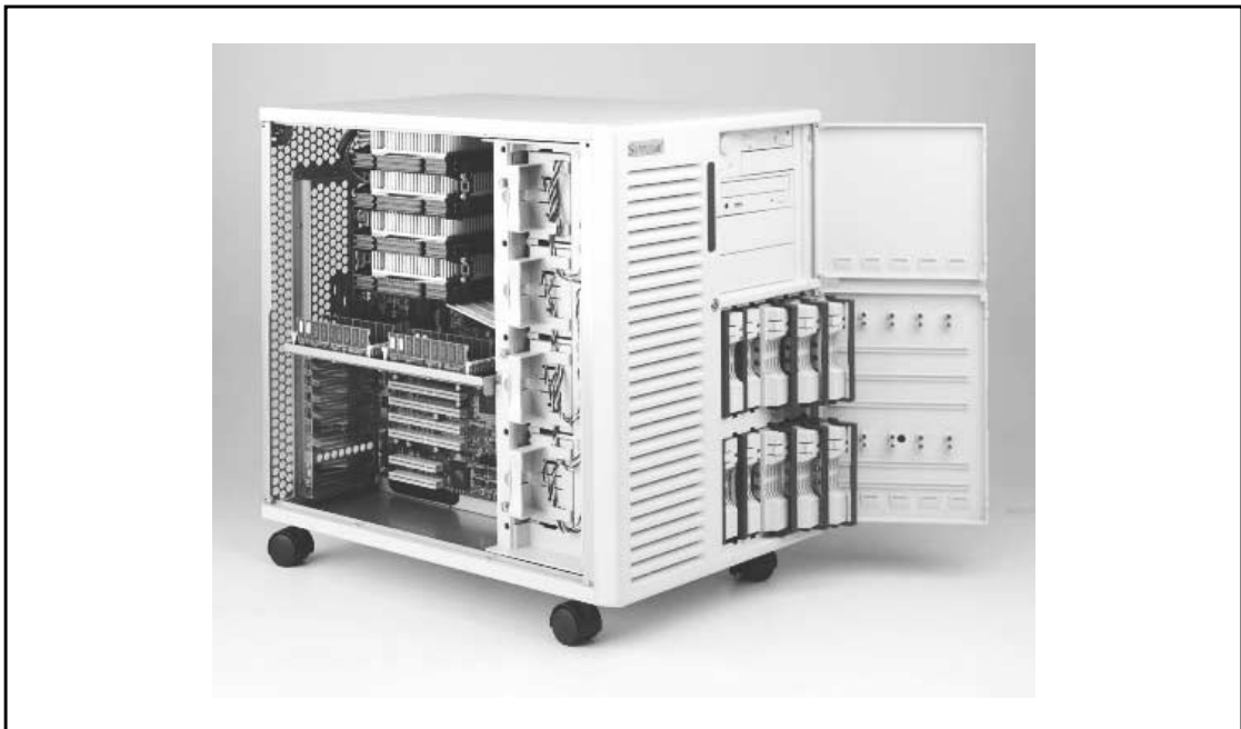
Figure 15-6. A WTX form factor computer with two front-panel doors. Photo courtesy of Super Micro Computer
