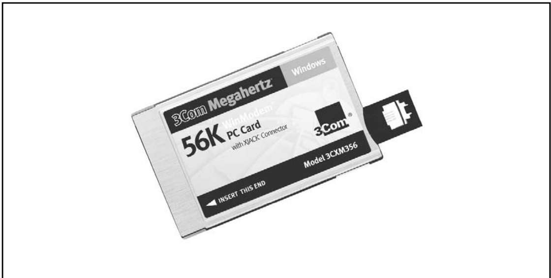
Figure 11-17. A PC Card modem for a portable computer with an X-jack. Photo courtesy of 3Com/U.S. Robotics
