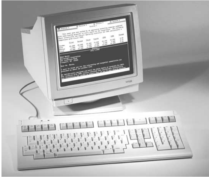
Figure 1-3. Terminals, like the VT 520, are one way to connect to a mainframe. Photo courtesy of Boundless Technologies
