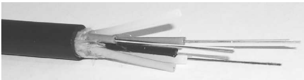
Figure 20-7. The makeup of a fiber optic cable
