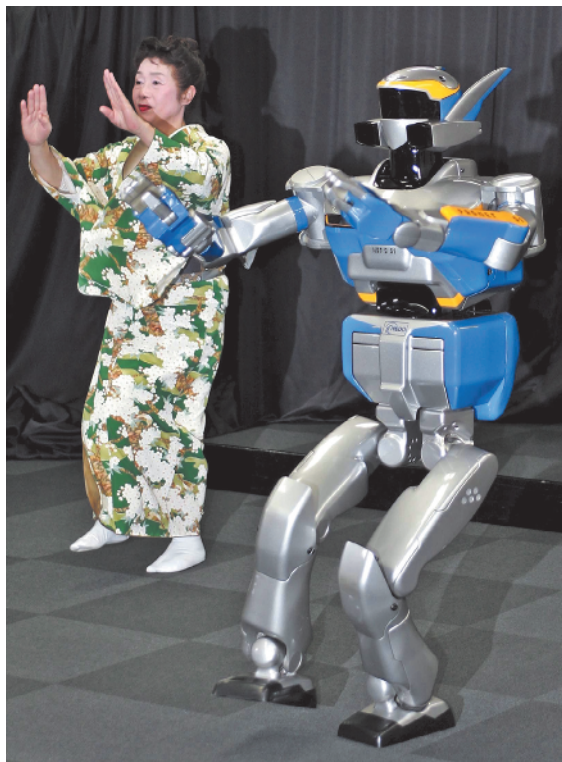
Robots. (Left) A new humanoid robot, HRP-2 Promet, developed by the National Institute of Advanced Industrial Science and Technology and Kawada Industries, Inc. Five feet tall, it performs traditional Japanese dancing. Priced at $365,000, the robot can help workers at construction sites and also drive a car. (Right) This sea bream is about 5½ pounds and can swim up to 38 minutes—before recharging. The robot fish, created by Mitsubishi, looks and swims exactly like the real thing.
