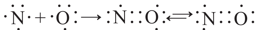
Figure 3.10. Formation of NO. The uneven number of electrons cannot accommodate complete octets around both atoms simultaneously, so the structure is a hybrid resonance structure of the two forms shown.
