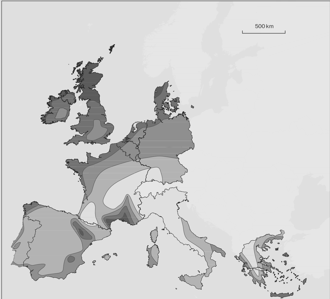
Wind resources at 50 metres above ground level for five different topographic conditions
