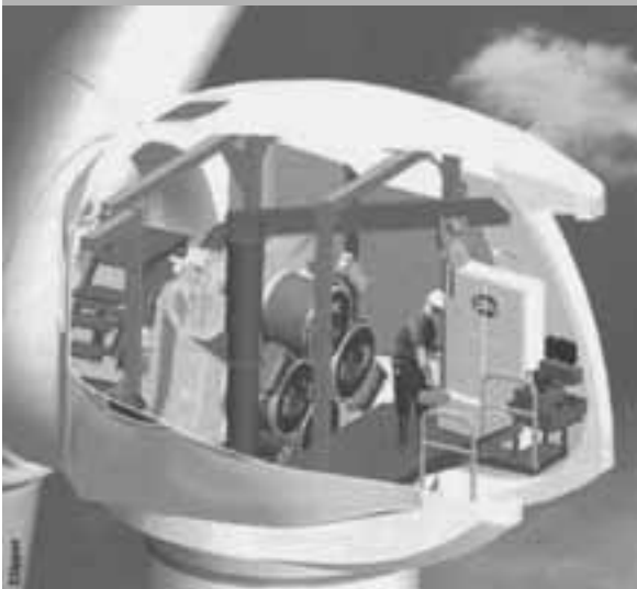
Figure I.3.32: Clipper Windpower Liberty wind turbine with Multi-PMG system
