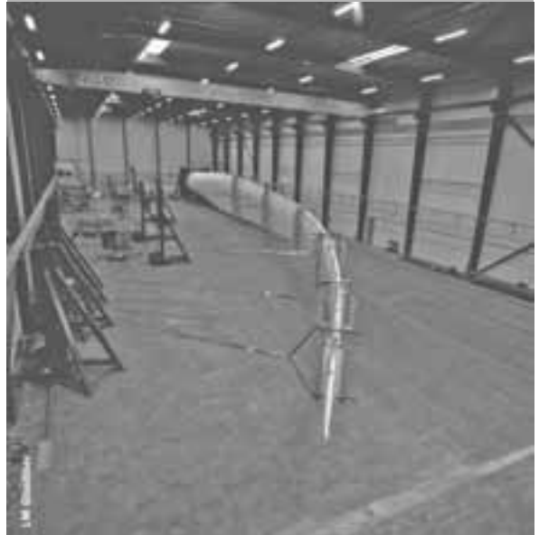
Figure I.3.28: LM Glasfiber blade test (LM 61.5 m blade for 126 m rotor diameter)
