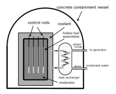
Ideally fission should proceed at the rate of one fission for one neutron produced. The trouble is that in the process two and sometimes three neutrons are produced. To limit the numbers of neutrons in the reactor **control rods** are used. These are rods of <u>boron-coated</u> <u>steel</u> which absorb neutrons. When the rods are raised from the reactor, neutron numbers increase. When they are lowered, neutron numbers decrease. In this way the rate of fission is controlled.
