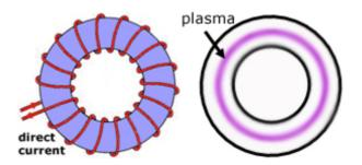
Because the particles are charged they corkscrew around the magnetic field lines. The most effective shape is a doughnut or toroid. This produces a powerful magnetic field within it, much like a linear electromagnet, but closed into a loop.
