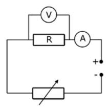
The current through a resistor is varied, while the p.d. across it is measured. The graph of V against I is a straight line through the origin.
