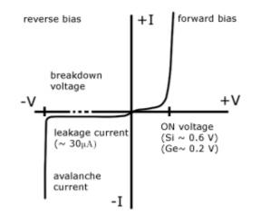
On a V-I graph the top right quadrant shows how a very small forward p.d. causes the diode to conduct. Notice the high current for a small p.d. increase.
