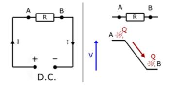
Charge loses potential energy(PE) as it moves through the resistor. This electrical PE is transformed mostly into heat energy dissipated in the resistor.
