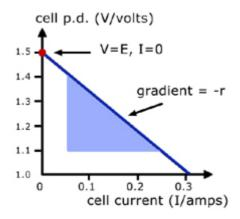
Information can be obtained from the graph by manipulating the equation obtained for E and r:
