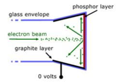
A layer of graphite is painted on the inside of the vacuum tube close to the fluorescent screen. As a result of impacting electrons, the screen acquires a negative charge. To reduce this effect, the graphite is electrically connected to 'earth' (zero volts). This allows excess charge to drain away.
