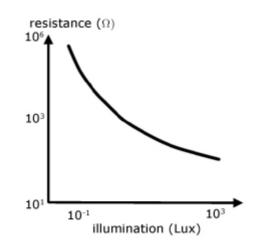
Typically effect of light on a LDR is to reduce its resistance from ~  $10^6 \Omega$  to ~  $10^2 \Omega$ .
