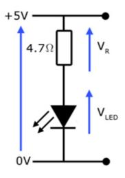
Example: Find the limiting resistor for an LED, where:
