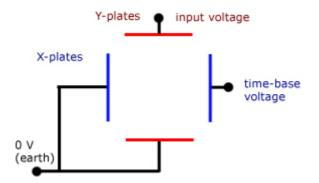
To display a waveform, a repetitive reversing voltage is applied to the X-plates. This causes the electron beam to be slowly repelled from the left-hand plate and attracted towards the right-hand plate. On the CRO screen this translates as an illuminated dot moving from left to right.
