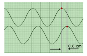
Example: The phase difference is 0.6 cm and the wavelength is 3.1 cm. therefore : phase difference ( $\phi$  phi) =( 2  $\pi$  x 0.6)/3.1 = <u>1.2 rads</u>.
