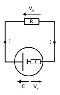
The total resistance  $R_{\text{total}}$  is the sum of the series resistor and the internal resistance of the cell.
