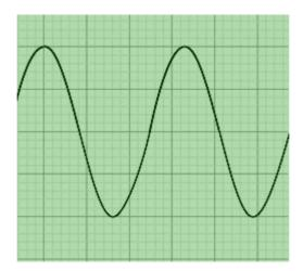
Example: In the example above, measuring from the first crest to the second horizontally, the distance is 3.3 cm.
