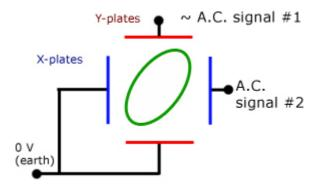
Different ratios of frequency give different images. In this way an unknown frequency can be identified, provided it is in a simple ratio with the first frequency.
