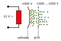
This beam current is controlled by having a grid over the cathode. The p.d. of the grid can then be varied to accelerate electrons through it or repel some back to the cathode.
