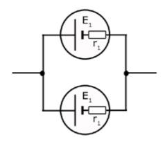
For similar cells the EMF's are equal and the internal resistances are also equal.
