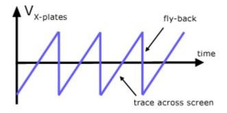
The voltage is then reversed and increased rapidly. The effect is to move the dot very quickly from right to left (fly-back).
