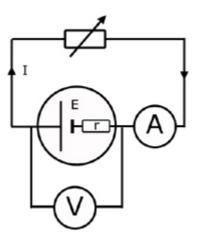
After taking readings of terminal p.d.  $(V_R)$  and current (I), a graph is drawn.
