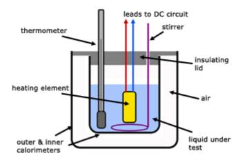
The heat energy supplied by the electrical element is given to the liquid and its container, producing a temperature rise  $\Delta \theta$ .
