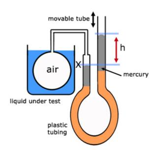
In its original state the glass bulb is full of air and the mercury levels are the same. A mark(X) is made against the glass to record this.
