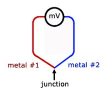
Thermocouples work on a principle called the **thermoelectric**or **Seebeck Effect**.
