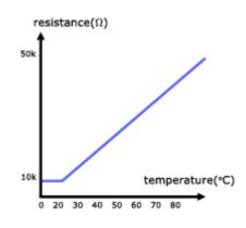
The property of metals that their resistance is temperature-dependent makes them ideal as thermometers. The metal of choice is platinum as a result of its high melting point(1773°C) and large resistance temperature coefficient\*.
