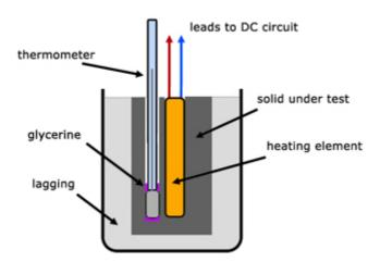
The method is very similar to that for a liquid except that there is no container. The solid under test is a lagged cylinder with holes drilled for the thermometer and the heater element. A little **glycerine** is added to the thermometer hole to improve thermal contact.
