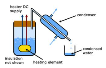
Water is heated electrically until it boils. The condensed water (m) is collected over time (t). Heating element readings of voltage (V) and current (I) are recorded.
