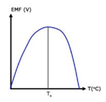
On the graph, the value of T where the EMF is maximum is called the **'neutral temperature**'. The gradient (d(EMF)/dT) anywhere on the curve is called the **thermoelectric power**.
