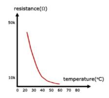
Semiconductors like metals have resistance that is temperature-dependent. So they too make ideal thermometers.
