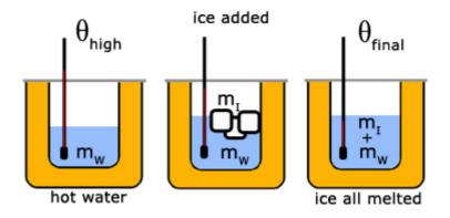
Ice cubes are added to hot water of known temperature in a copper calorimeter. The mixture is stirred until all the ice has melted and a final reading of temperature taken.
