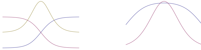
Figure 8.6: The initial data is \phi_0 = 0 and bump function \dot{\phi}_0 = 2 \cosh^{-2} x shown on the left. Also shown are f(x) = \tanh(x) and g(x) = \tanh(-x) . On the right you see the initial data \phi(0) again, and the wave \phi(x) at time 2. This is supposed to illustrate that wave lingers near the origin forever and the failure of Huygens principle in one dimension.
