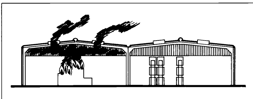
2 With vents & smoke reservoirs fire can be quickly contained & controlled
