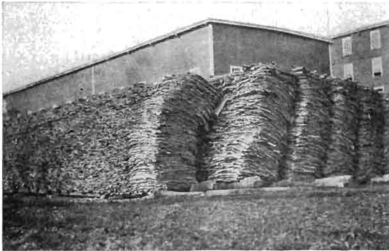
FIG. 56.—Hemlock bark ready for use, stacked at a Maine tannery. (Photo by U.S. Forest Service.)
