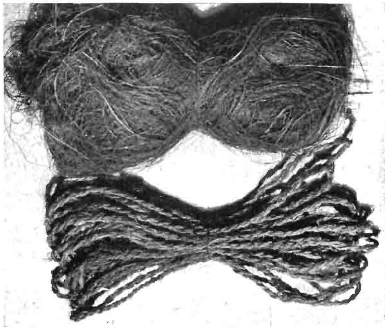
FIG. 17.—Above, coir, the coarse fibers from the husk of the coconut ( Cocos nucifera ); below, sennit, the rope that is made from it. Sennit is the most universally used type of cordage in the South Seas. (Courtesy of the Botanical Museum of Harvard University.)
