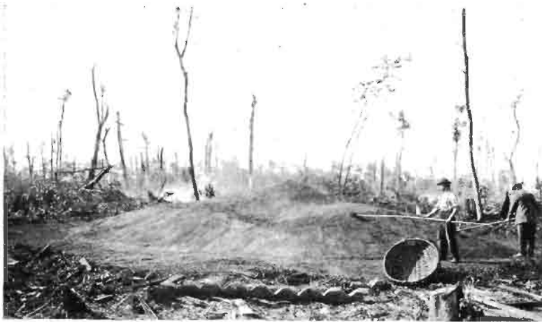
FIG. 35.—Cleaning the dust in a charcoal pit in Pennsylvania. (Courtesy of S. J. Record.)
