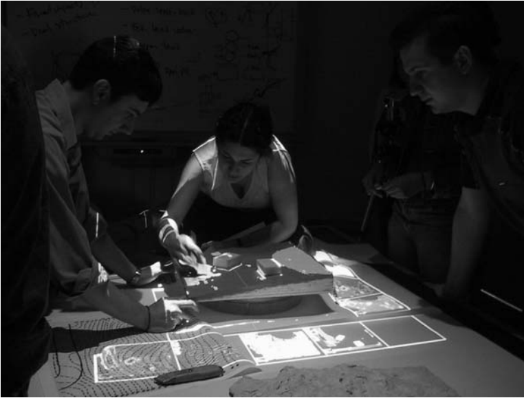
Figure 20.3 Illuminating Clay combines physical models and digital information. Source: © Eran Ben-Joseph. Note: Illuminating clay is an example of Tangible User Interfaces (TUIs), which allow for design and simulations that are comfortable, intuitive and collaborative.
