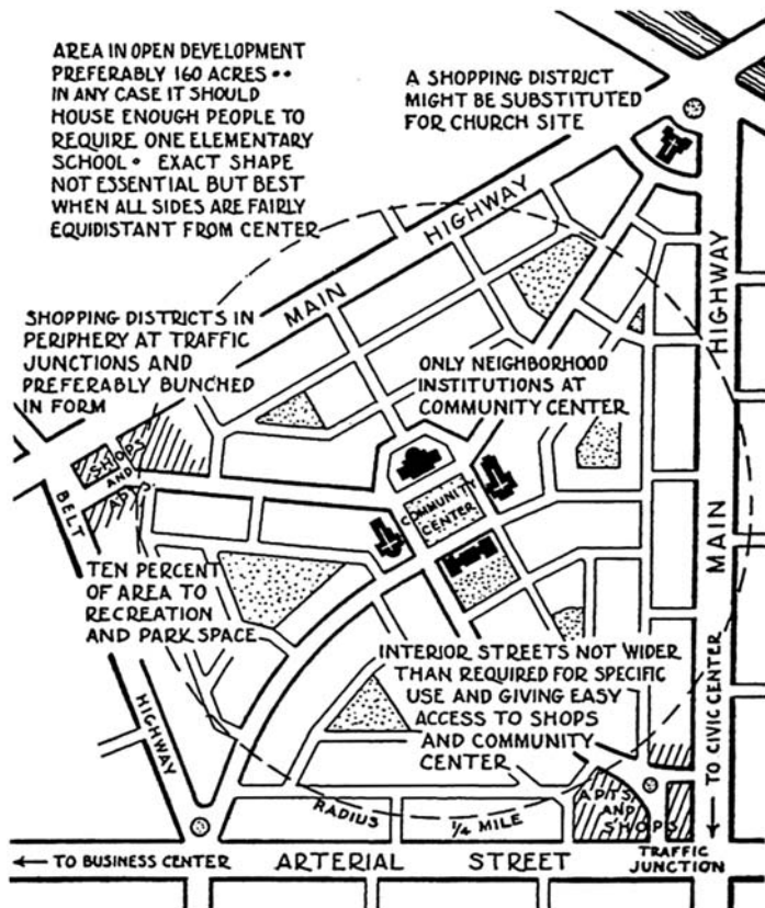
Figure 29.1 Neighborhood unit diagram. Source: Committee on Regional Plan of New York and Its Environs. Regional Survey of New York and Its Environs (Vol. 7). New York (1929) – used by permission. Note: Conceptual diagram of the neighborhood unit as originally conceived for the New York Regional Plan.
