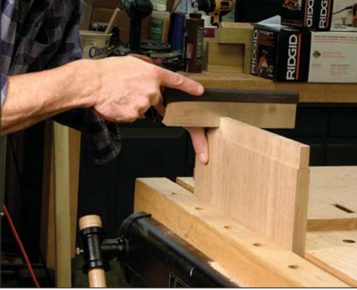
Begin at the end. Cut the ends of the tenons first with a backsaw, then use the same saw to cut away the outside corners.
