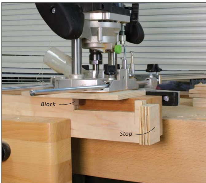
The block is lined up with the bit so that the template can be made to the exact size and location of the mortises.
