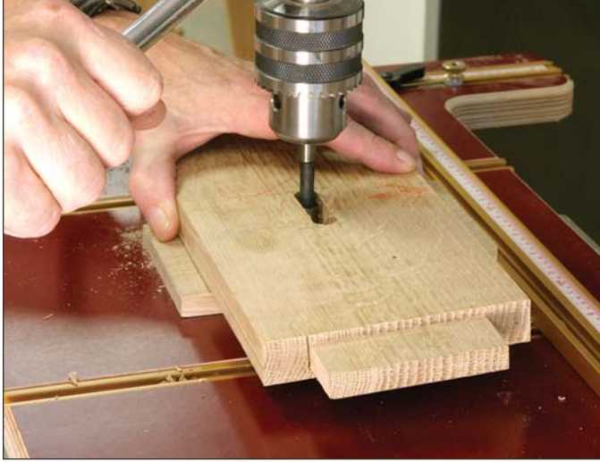
The angled mortises on the lower rails were roughed out with a Forstner bit on the drill press. A tapered block under the workpiece makes the holes at the correct angle.
