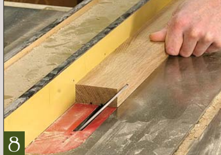
8 After the grooves are cut, the saw is again tilted to 45° and the waste is removed. Leave about 1/4" of flat on the edge to ride against the router table fence.
