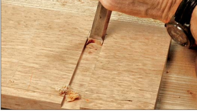
Finish by hand. A few cuts with a chisel complete the end of the dado for the top and bottom shelves. The front edge of the shelf is notched and ends 1/2" past the end of the dado. The notch is cut by hand with a dovetail saw.
