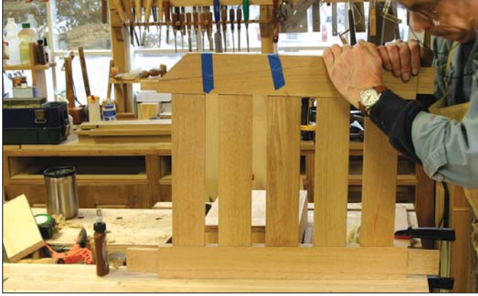
Don't throw that away. The offcuts from tapering the upper rails are taped back in place to keep the clamps from sliding during assembly.
