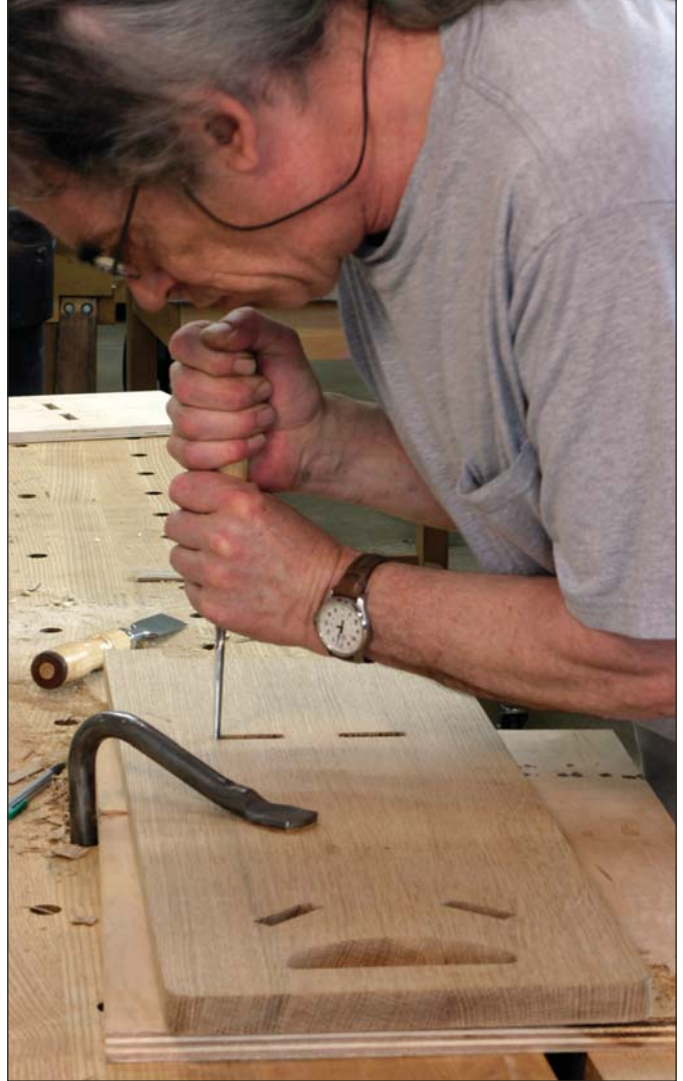
On top. Positioning your shoulder over the chisel allows you to use your body weight to pare the end of the mortise.
