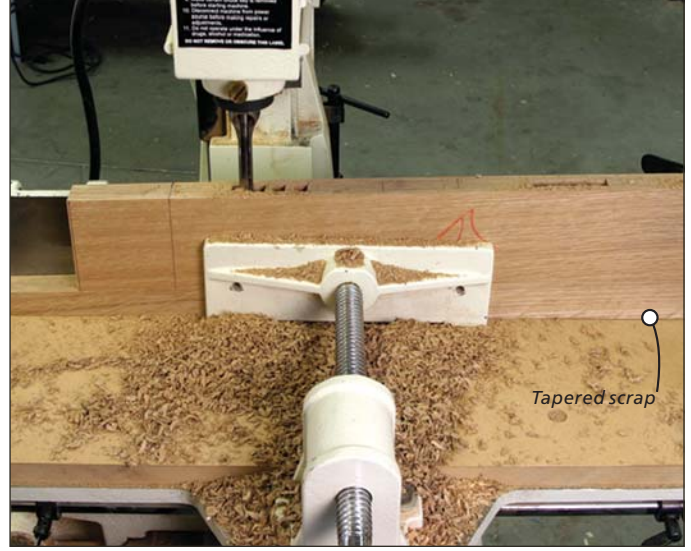
Keep your head straight. A tapered piece of scrap below the workpiece keeps the mortises oriented vertically.
