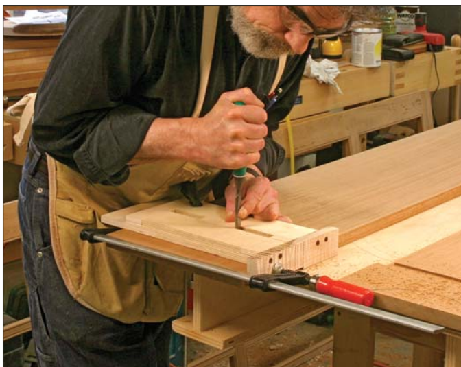
Double duty. After routing, the mortising jig also serves as a guide for the chisel to square the corners of the through-mortises.
