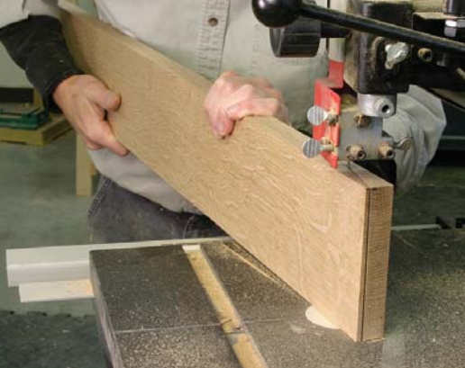
A little off the top. An angled wedge sliced off the end of the arm forms the bend.
