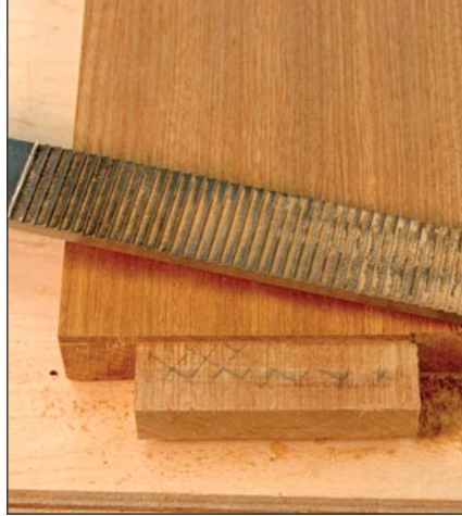
A little off the top. The pencil lines smear where material needs to be removed. A planemaker's float gives good control and leaves a smooth surface.
