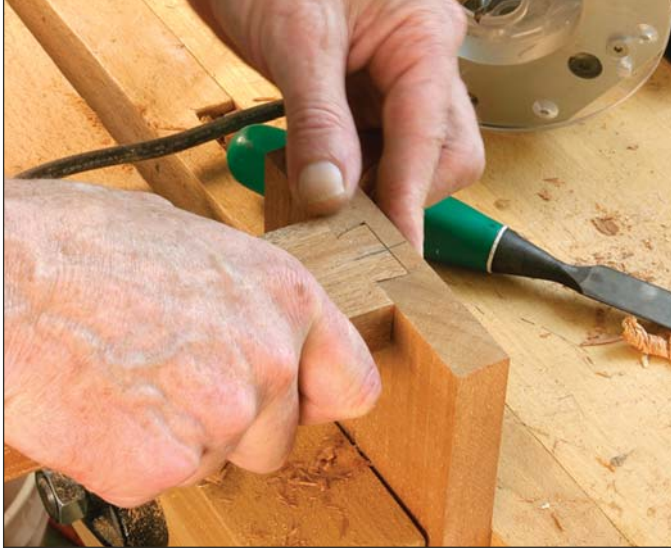
Never to be seen. These joints won't show in the finished table, but they must be strong. The sockets in the legs were wasted with a small router; the sockets in the hub with wasted with a Forstner bit. I then pared them all to size with a chisel.
