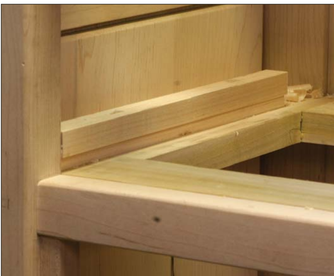
Adjustable guide. The drawer guides are glued to the web frame. The short length and rabbeted bottom edge provide room to adjust the width with a block plane.
