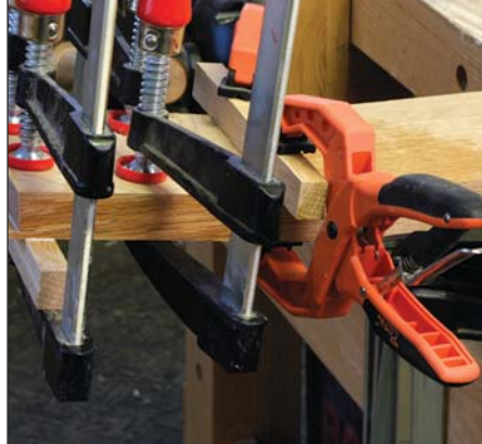
Get to the bottom. The wedge is glued to the underside of the arm, smooth face to smooth face.
