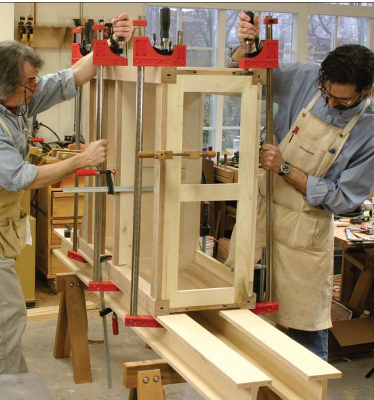
Several joints must be fit at one time as the second panel and leg assembly is put in place. Get some help so both sides can be fit and clamped at the same time.
