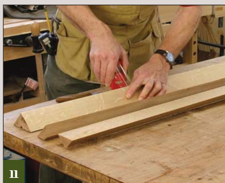
11 After all the parts are milled, I assemble the corners and hold them together with packing tape. All but the last corner is taped before gluing. I then flip the taped parts over, put glue on the edges, then fold the parts back together, taping the last corner.
