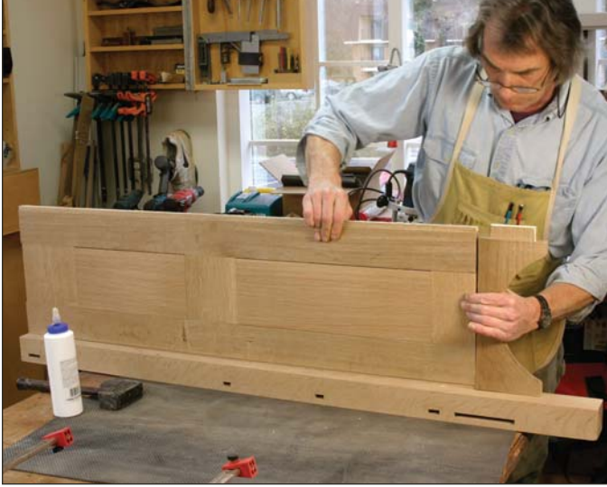
The side panels are assembled as a unit, then fit in a groove in the leg, and butted at the bottom to the thicker arched rail.
