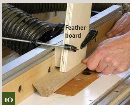
10 After making some test cuts and fine tuning the router table setup, the edges are beveled. The block behind the featherboard holds it away from the fence, so it is pushing down on the narrow flat left between the two bevels.
