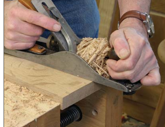
Smooth it over. Planing out the band saw marks leaves a smooth surface on the top and bottom of the arm.
