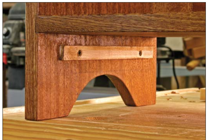
Simple enough. Maple runners below the bottom shelf support and guide the hidden drawer.
