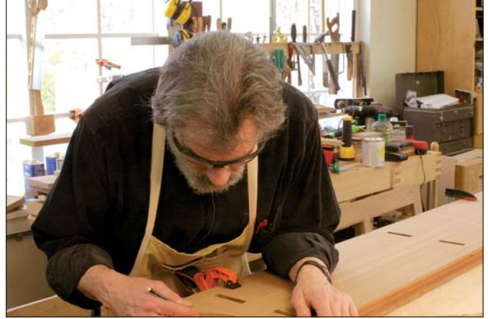
One side makes another. After the curves on one side are completed, the first side is used as a template to make the second side.
