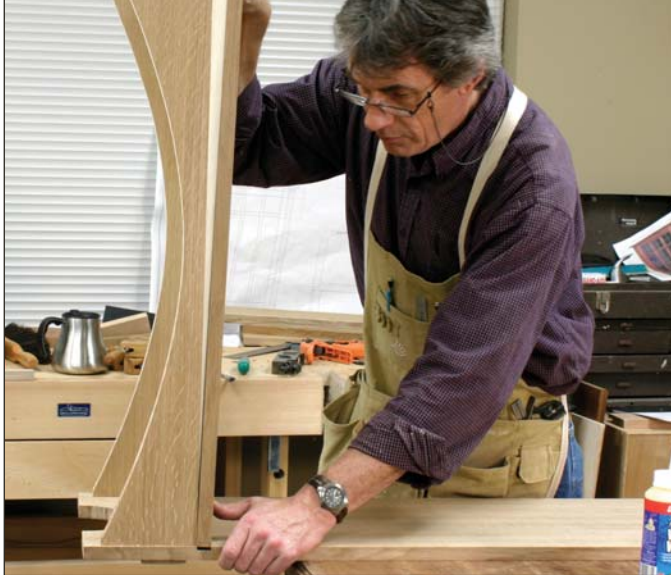
With the two bottom rails in place, I spread glue on the top edges of the rails and in the dado before tipping the bottom in to place.
