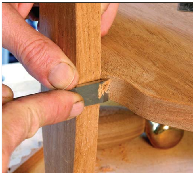
Final cut. After shaping the legs and the shelf, the intersection is blended with a #1 straight carving chisel. Leaving these small areas oversized until almost the end of the project resulted in crisp detail in a highly visible place.
