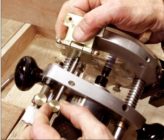
Better than measuring. Use a leaf of the hinge to set the depth stop on the plunge router. Set the bottom of the bit flush with the router base, then set the depth stop to the hinge. Plunge the router to the stop and you're set.
