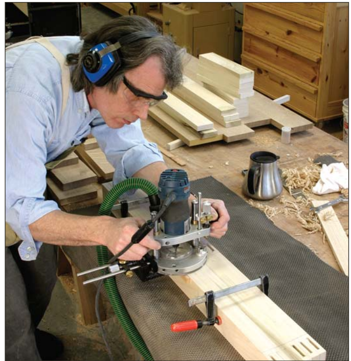
A group of stiles for the web frame is clamped together to lay out the joints. Leaving the stack clamped together provides a stable base for the router used to cut the mortises.
