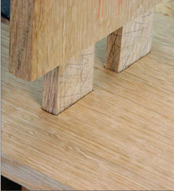
Ease in. Bevel both the ends of the tenons and the edges of the mortises for fitting.
