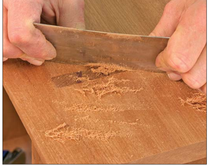
At the same level. Following the plane, a scraper is used to smooth the exposed tenon ends and the cabinet sides.
