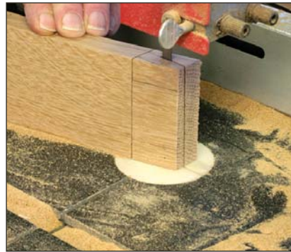
Quick cheeks. A band saw is an efficient way to cut the tenon cheeks, or you can cut them by hand. Either way, cut a little wide and make the tenons fit with a shoulder plane or a float.
