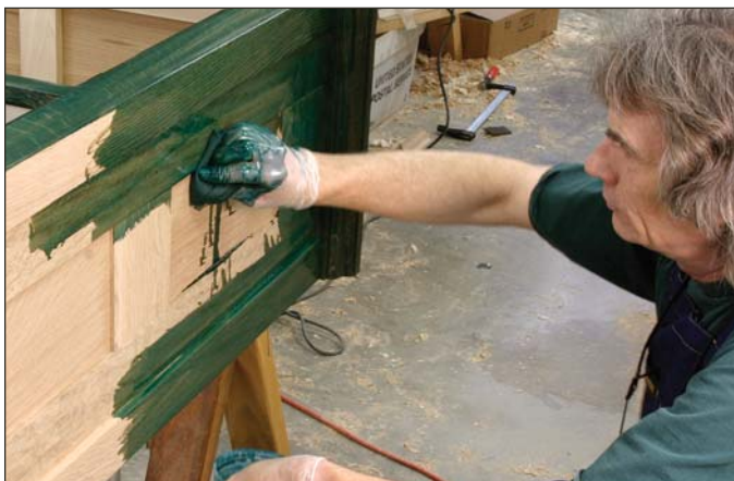
The stain, a mixture of artist's oil colors and Watco Danish Oil is liberally applied. After letting it soak into the surface for 15 minutes the surface is wiped dry.
