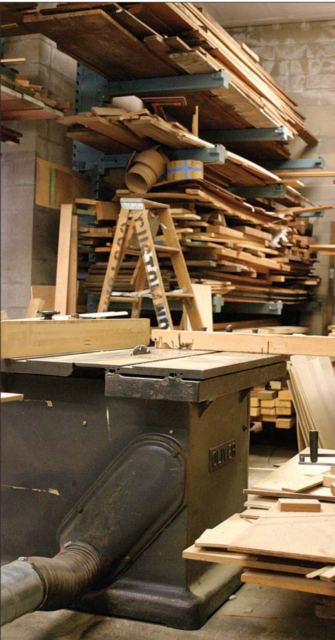
An ancient, but accurate Oliver sliding table saw and floor-to-ceiling stacks of lumber occupy the back half of the shop.
