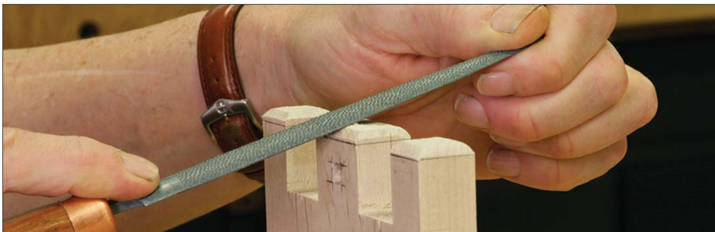
Cutting corners. Mark where the end of the drawer side intersects the fingers on the drawer front. Round over the edges to the pencil line.
