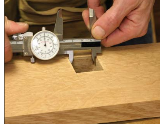
Careful comparison. Check the size frequently with calipers as you work on the mortise, and compare it to the tenon.
