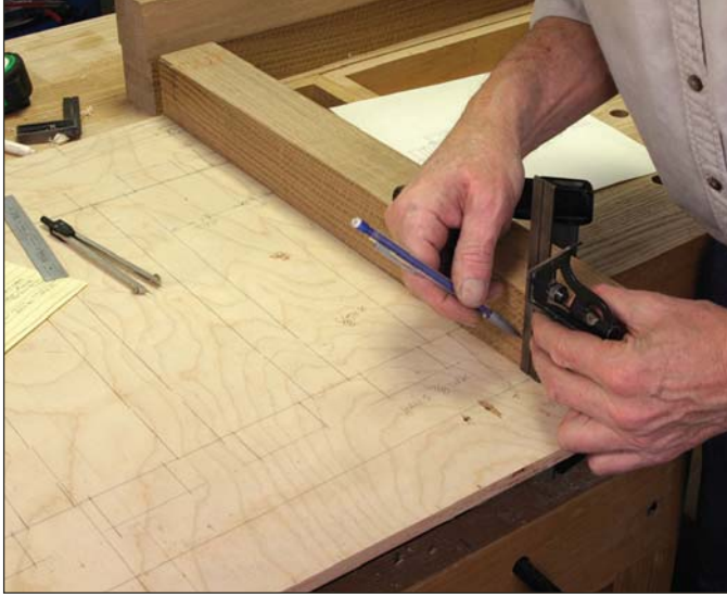
Measure once. A full-scale drawing provides a reference for most parts of the project. It saves time, and prevents measurement and layout errors.
