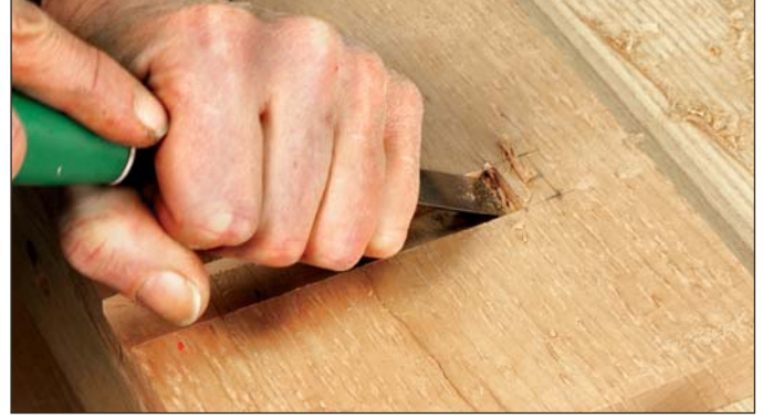
Finish by hand. A few cuts with a chisel complete the end of the dado for the top and bottom shelves. The front edge of the shelf is notched and ends 1/2" past the end of the dado. The notch is cut by hand with a dovetail saw.
