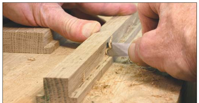
Run in reverse. The back of a chisel makes a great scraper, just the ticket for cleaning out the corner of rabbets.
