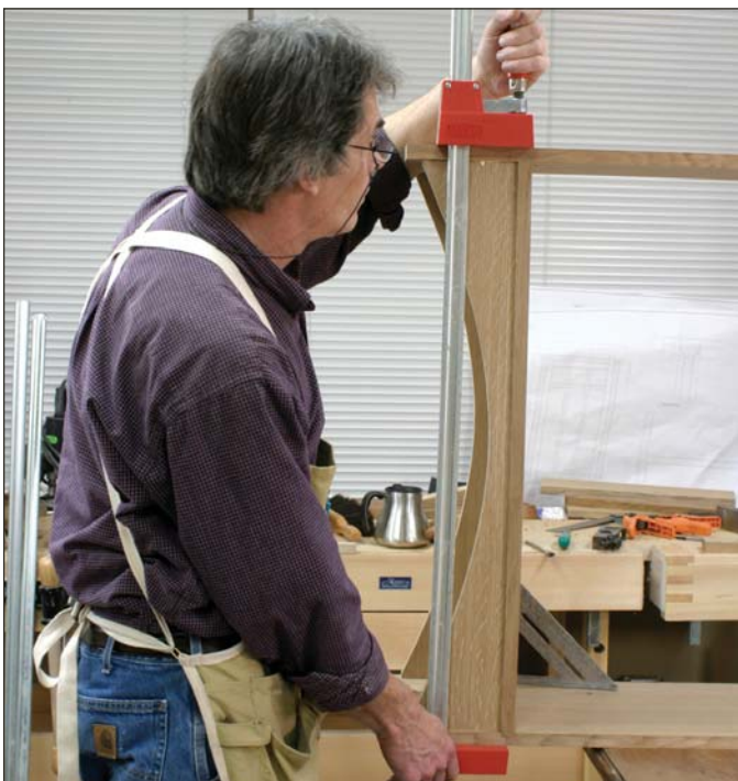
Because of the mechanical fit of the rails and bottom, it only take a couple clamps to secure the bottom of the case assembly.
