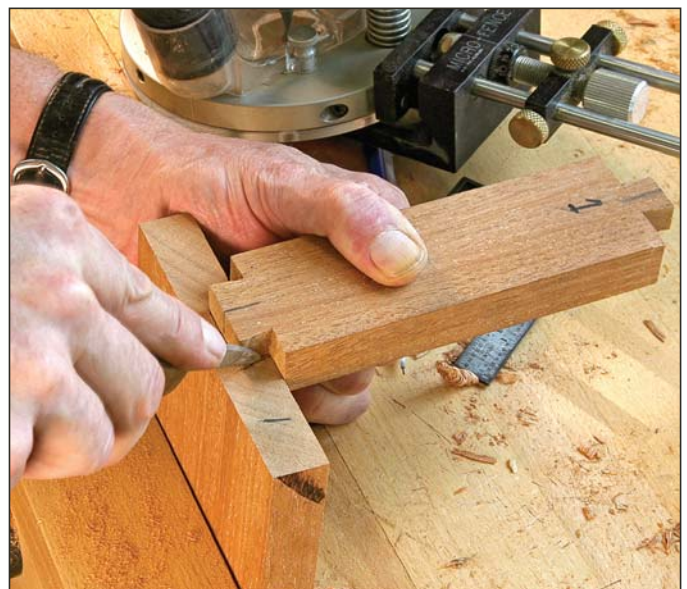
Hidden lapped dovetails. The stretchers connect to the hub and the leg with \frac{1}{2} "-thick lapped dovetails. They are \frac{3}{4} " wide at the hub end and 1" wide at the leg.
