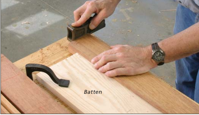
Each of the tenons is planed to fit snugly in its mortise. A batten across the bench eliminates the need to clamp the parts while fitting.
