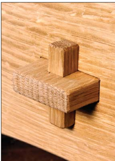
After cutting the key to length, I round the edges above and below the completed joint.
