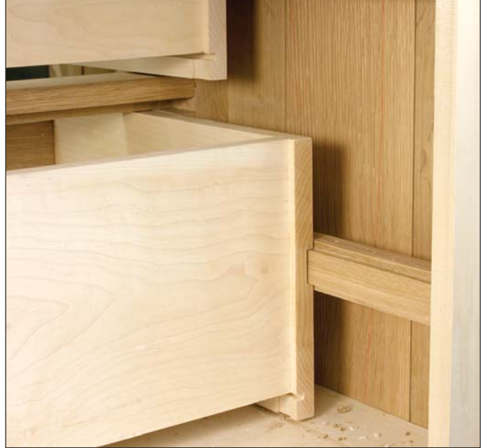
The back of the drawer runner is screwed to the back leg after being squared to the front of the cabinet. A groove in the side of the drawer box lets the drawers slide nicely.
