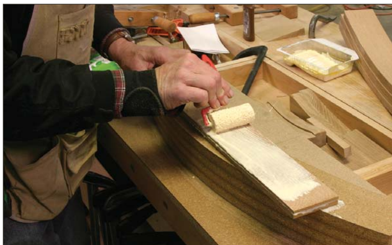
Work fast. Use a roller to spread glue on one side only of the laminations for the back. Keep the pieces in order and the edges will match.
