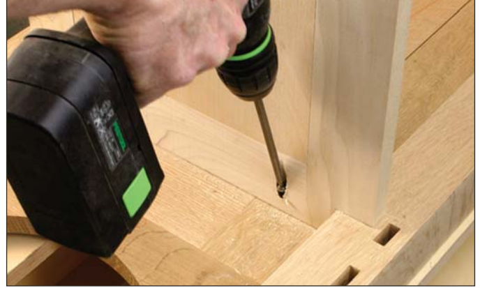
The web frames are notched around the legs and attached to the side rails with pocket screws. The front and back edges will be glued to the rails as they are assembled.
