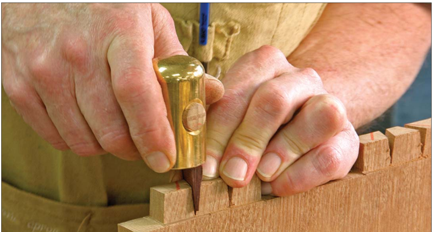
One size fits all. In theory, the tapered wedges will fit anywhere. In reality, I fit each one and kept them in order.
