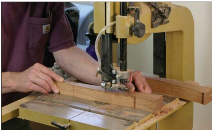
A stack of four blanks held together with double-sided tape yields eight matching corbels.
