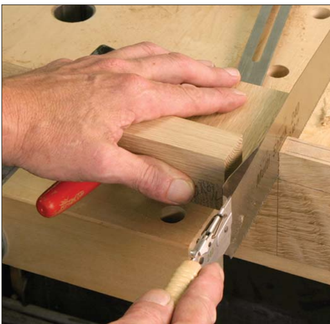
The quick and easy way to make the angled cuts for the through tenons is with a handsaw, guided by an angled block of wood.
