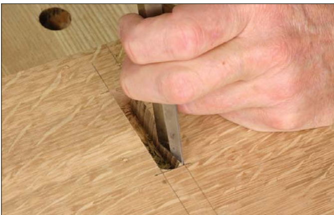
And swing it. Keep the back of the chisel pressed against the routed edge of the mortise and carefully rotate the edge into the corner.
