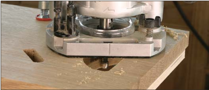
Saw first, then trim. Cut close to the lines with a jigsaw and use the router to trim the opening at the top.
