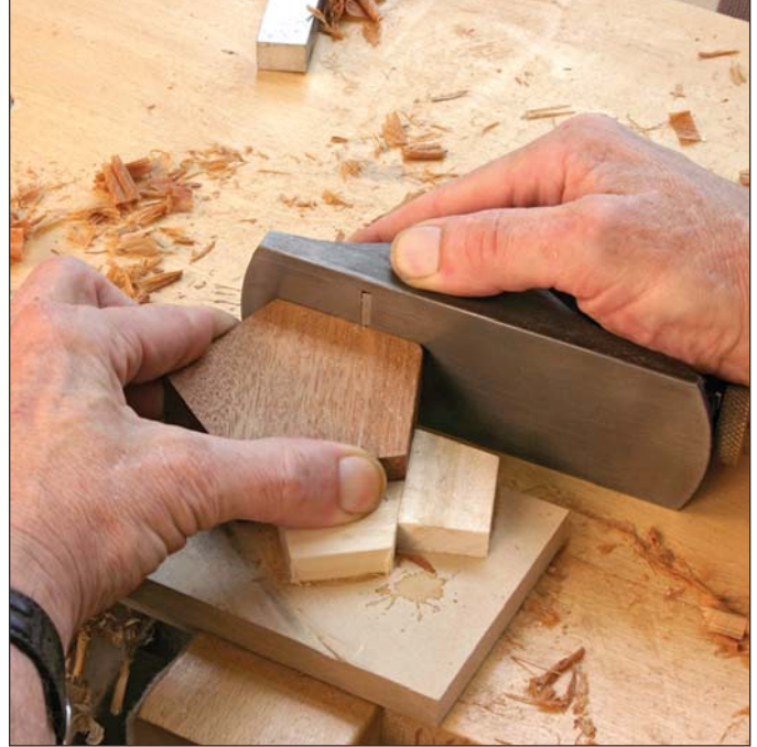
The hub is the keystone. All of the structural parts of the table radiate from this small piece, so it needs to be precise. This shooting jig lets me trim it down in tiny increments.
