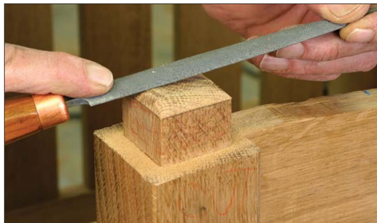
After the fit. Mark the intersection of the arm and the tenon with a pencil line and round the end of the tenon down to the edge. Stop just outside the line to maintain the fit between the two parts.
