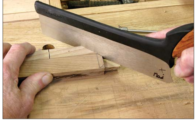
Miters, too. 45° cuts in the fence guide the saw to cut the short miters. Preserve the line at this point, and work down to it while fitting.
