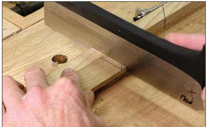
Use the fence. Saw cuts in the fence of the bench hook guide the saw to make clean and accurate cuts.
