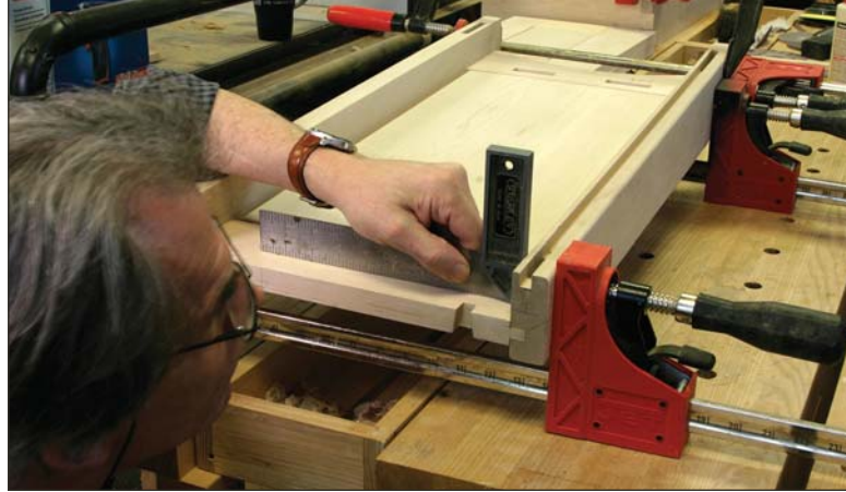
E pluribus unum. Subassemblies minimize the number of pieces to contend with during the final assembly. After clamping, check to see that they are square.
