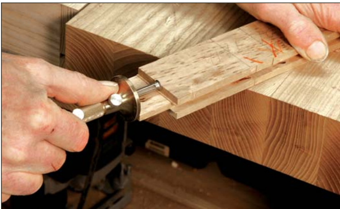
Dual-purpose tool. The cutter on the gauge removes the remaining material where the tenon cheek and shoulder meet. After scoring it with the gauge, pare with a chisel.
