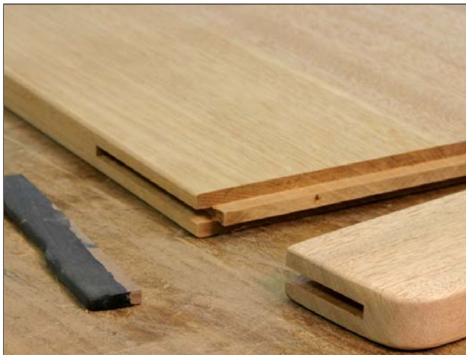
The breadboard end is attached to the tabletop with screws and the ebonized walnut spline is glued in the slot in the table only.
