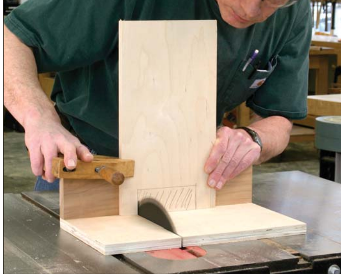
Guided by the kerf. One precise cut establishes the size of the tenon. This L-shaped jig attached to the miter gauge is simple and safe.
