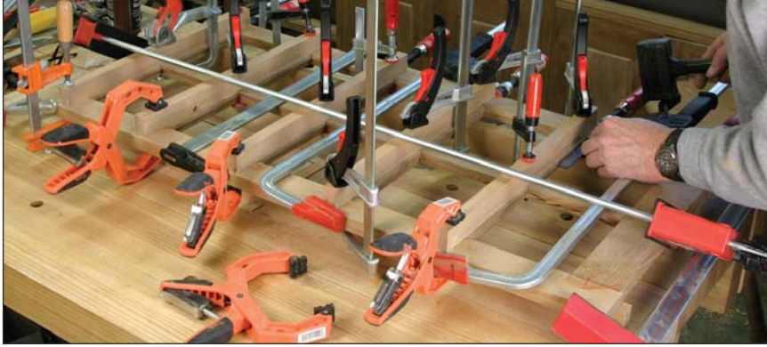
Payday. Flush the surfaces of the completed joints with a sharp block plane, and take a moment to feel proud. Then get back to work; there are a bunch of these.
