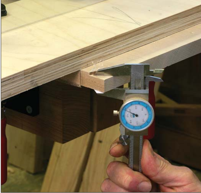
Knowledge is power. Measuring with calipers reveals the exact thickness of the tenon and how far to set the depth of the router bit.
