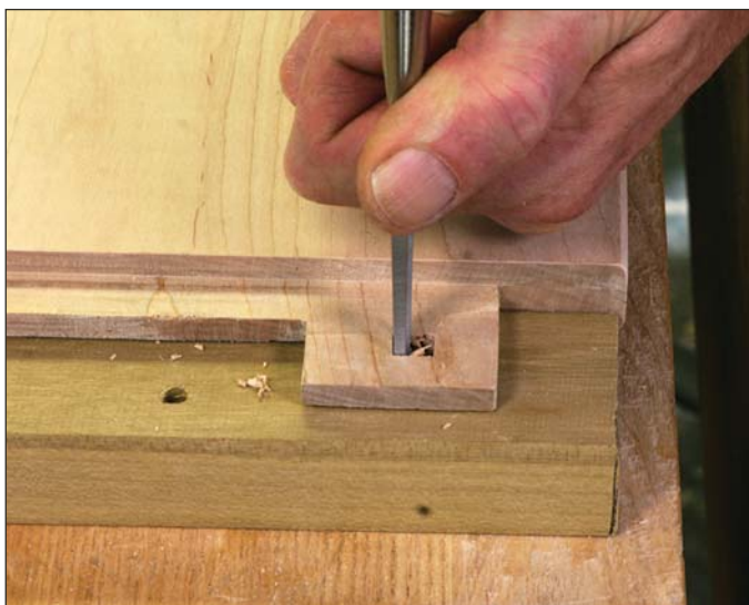
Room to move. Elongate the sides of the holes that pass through the tenons. This will allow the top to expand and contract against the breadboard ends.
