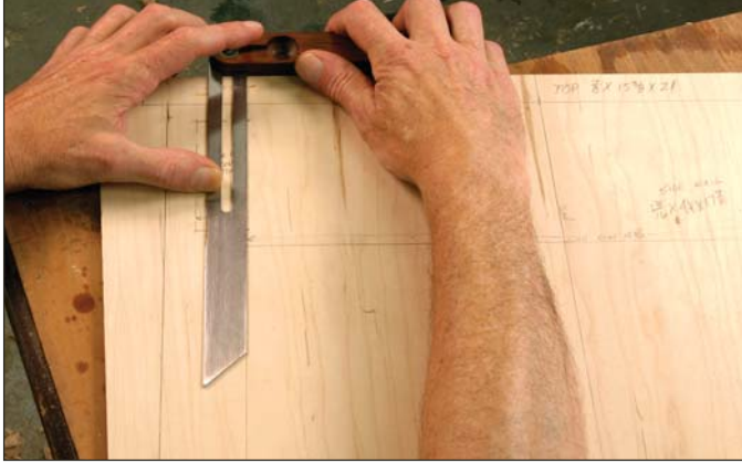
Using a full-size section drawing is essential; it lets me set angles and shows the exact sizes of parts without any of the risks of measuring.
