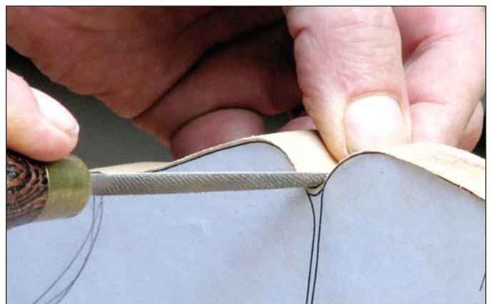
Rasp to the rescue. The flat side of this rasp removes the band-saw marks on most of the edge. The round side gets into places the flat side can't reach. Many of the finished tight curves are defined by the shape of the tool.
