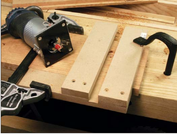
Quick custom jig. The dado-routing jig is made by clamping the two guide rails on either side of a shelf. The top-mounted bearing on the router bit then cuts the proper-width dado without measuring or fussing.
