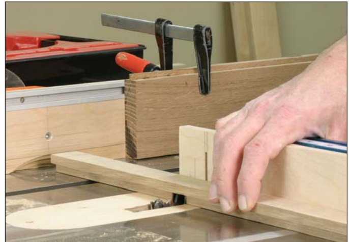
The half-lap joints, as well as all of the tenons for the door were cut with the dado head on the table saw as you can see here. The block clamped to the saw's fence locates the cuts without trapping the parts between the dado cutter and the fence.
