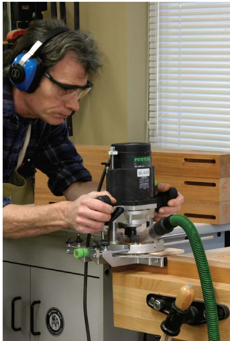
With the template and the leg held in the vise, the fence on the router places the cut laterally, and the block hits the template to locate the ends of the mortises. Using this method allowed me to mill all 32 mortises quickly and precisely, without doing any layout work on the legs.
