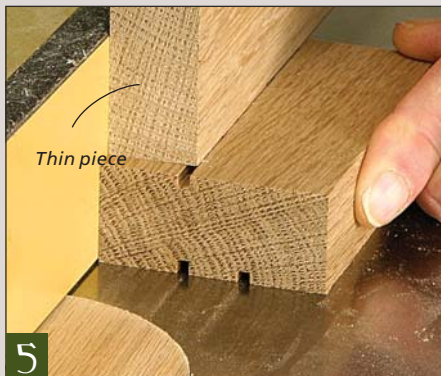
5 Make some test cuts in scrap. Check the width of the groove by placing the edge of the scrap against the fence, and a thin piece of scrap on top. When the corner of the thin piece meets the far edge of the groove, the fence is set correctly.
