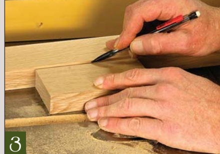
3 Set up to cut the grooves in the bottom of the thick pieces. With a thin piece of scrap against a thicker one, draw a line to indicate the difference in thickness. Flip the thicker piece over and use the pencil line to set the height of the saw blade.
