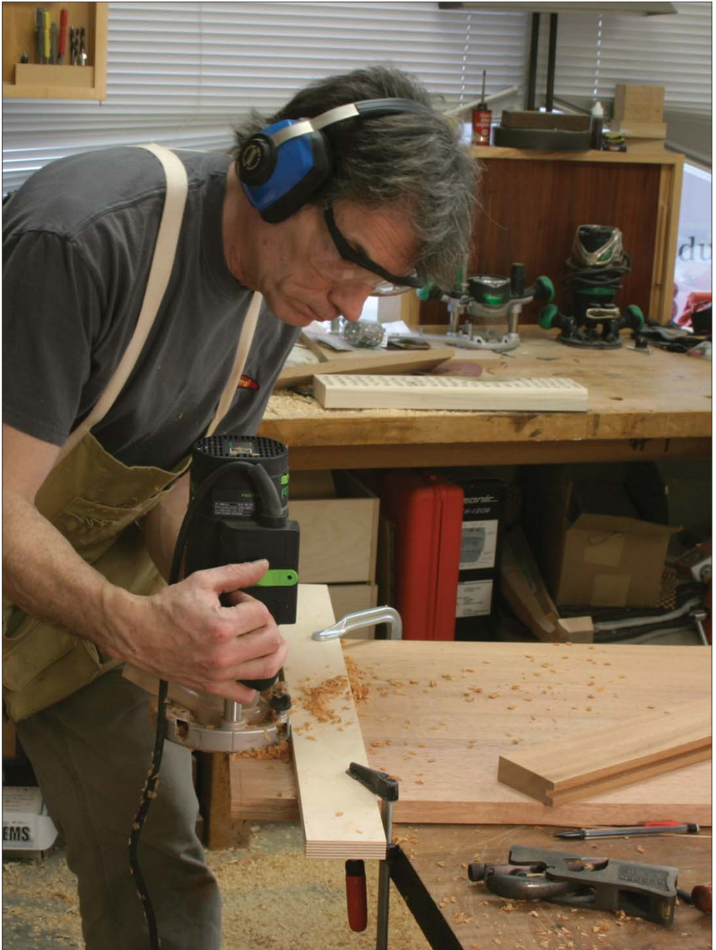
A piece of plywood clamped across the top guides the router to cut the tongue for the breadboard ends.
