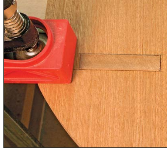
How it ought to be. The ends can be a bit loose because the wedges will expand the tenons.
