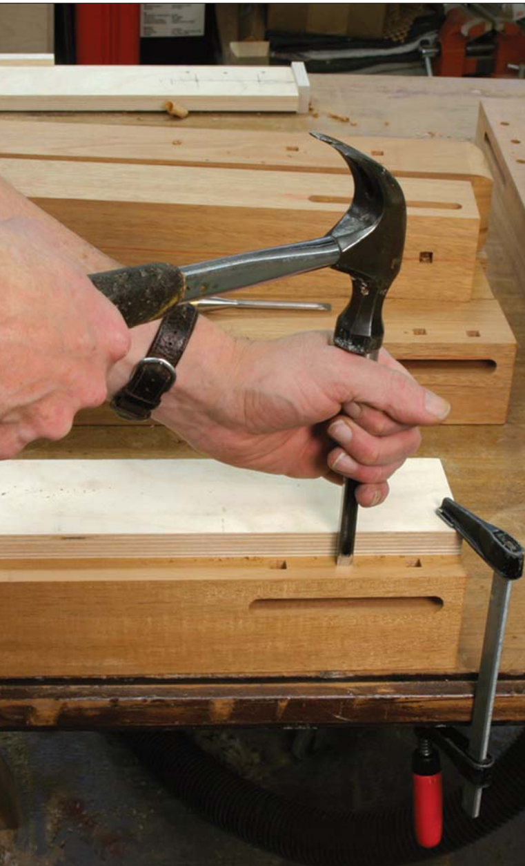
A modified chisel from a hollow chisel mortiser turns round holes square with just a few hammer taps. Plywood clamped to the leg keeps the chisel straight.
