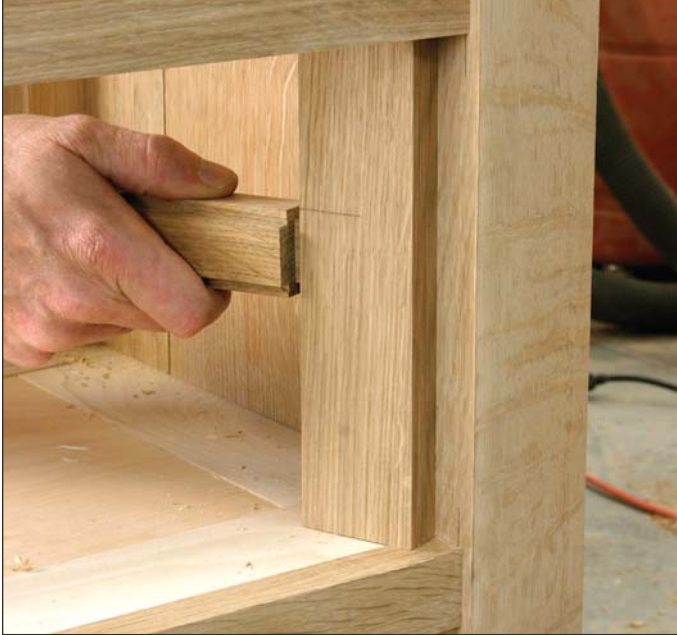
The drawer runners have a tenon on the front end that fits in a mortise in the stile. These are placed in position before the stile is glued in place.
