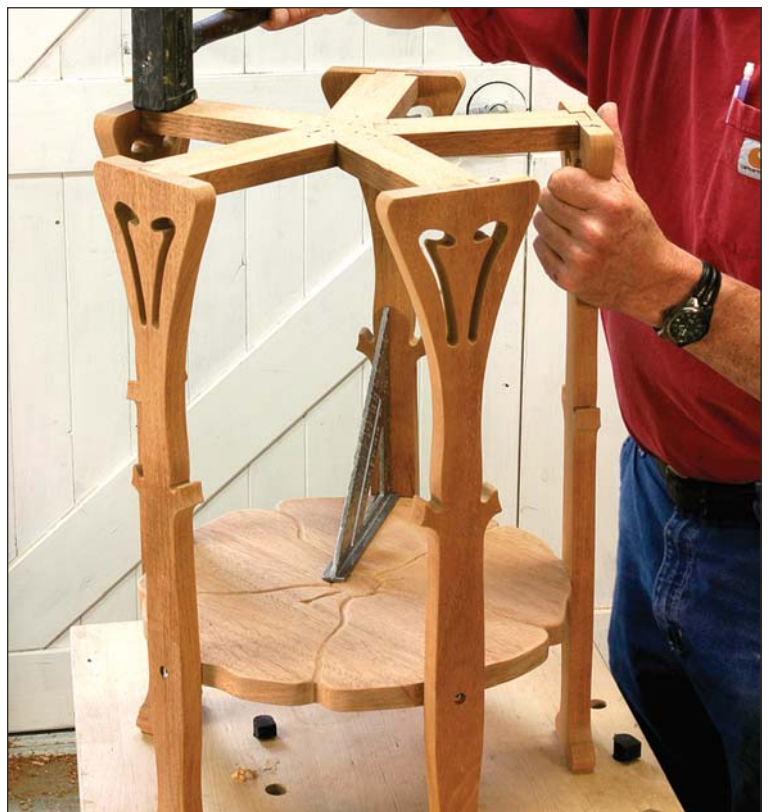
Last tap. The assembled hub and stretchers fit into the dovetail sockets at the top of the legs. When everything is lined up, they are tapped home, completing the assembly without using clamps.
