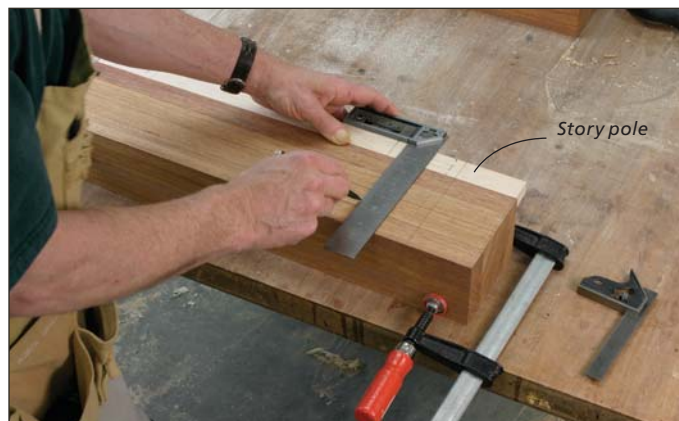
With the dimensions marked on a story pole, the locations for the mortises are marked on the legs as a group.
