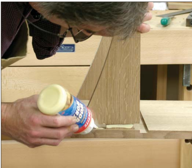
To control glue squeeze-out on the exposed tenons, I get the tenon started in the mortise, then apply glue directly to the tenon.
