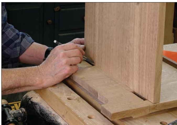
Make your mark. Wait until the mortises are completed to lay out the tenons on the cabinet top and bottom. Mark the locations from existing edges.
