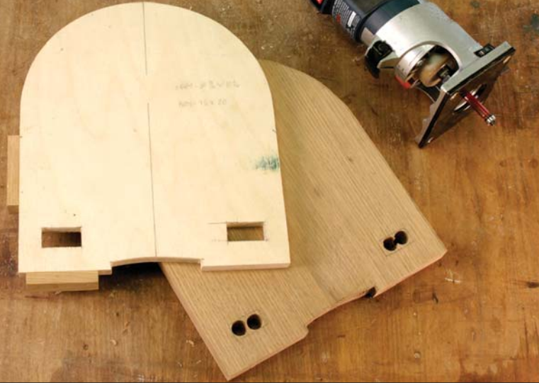
Form and function. The first template generates the shape of the ends and the through mortises. The oak blank below it is cut 1/16" oversize, and the holes minimize the work for the router bit.
