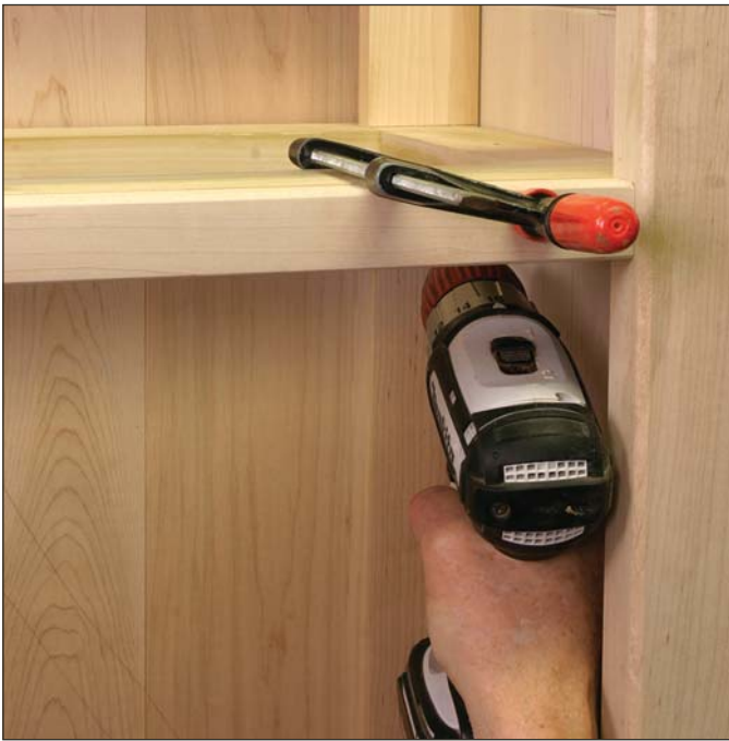
Simple fix. A pocket screw at each end attaches the drawer frame to the inside of the back legs.
