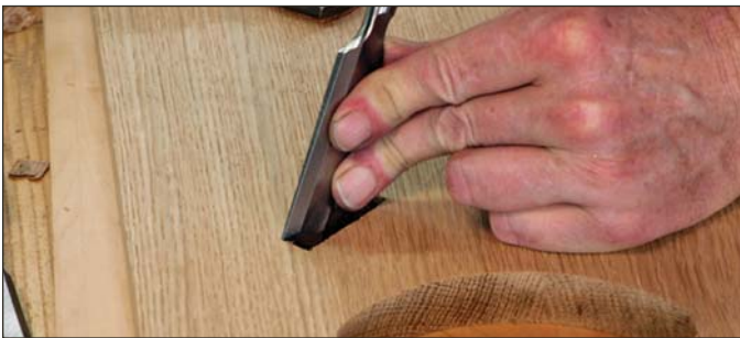
Swing it. Press the back of the chisel against the mortise wall, then rotate the edge down to the corner to maintain a straight edge.
