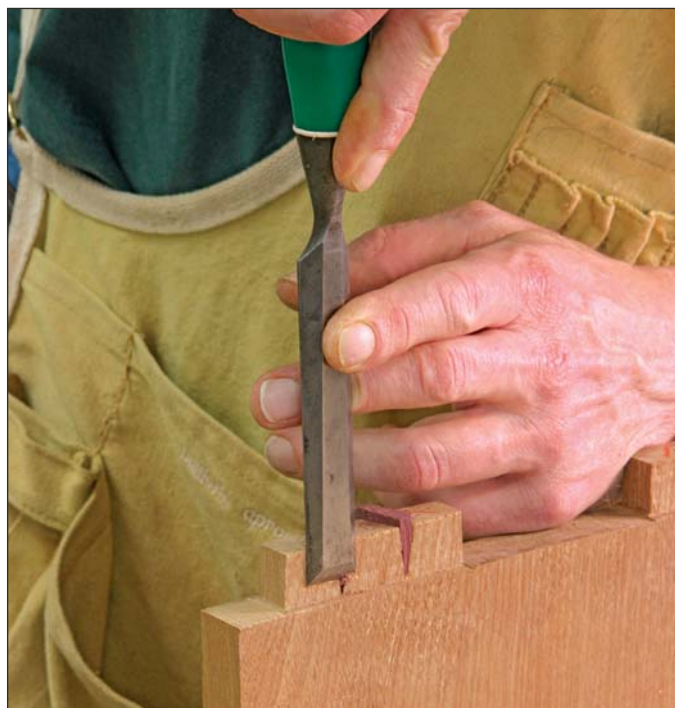
The easy part. Each wedge is pared flush with the surrounding tenon. Then they are removed and stuck to a piece of blue painter's tape.
