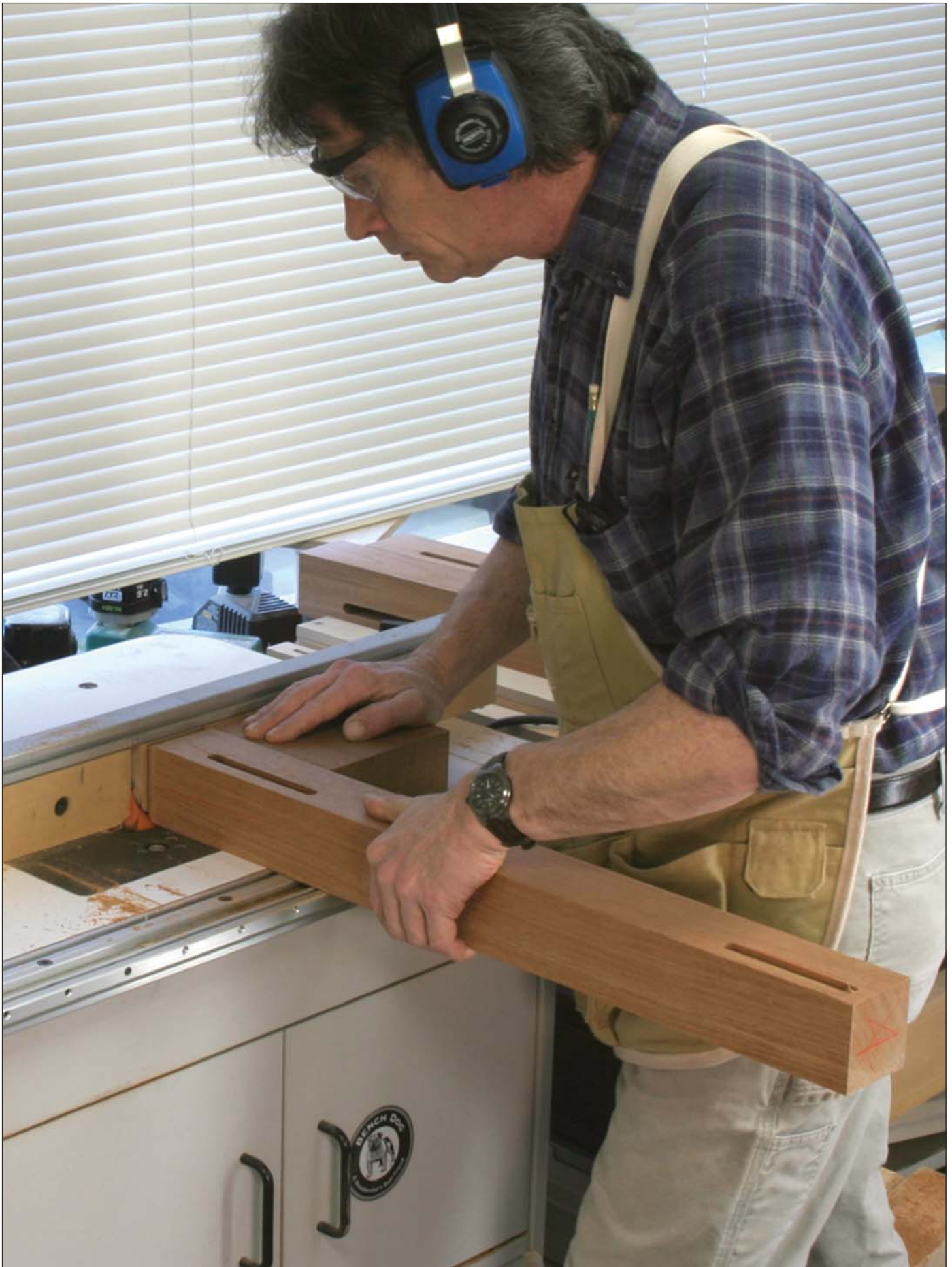
Just a portion of a 2"-radius roundover bit shapes the bottoms of the legs.
