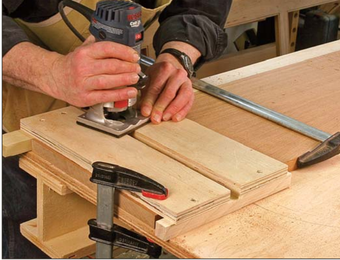
Dedicated jig. This dado jig is made to fit the thickness of the shelves, and utilizes a flush-cutting bit with the bearing on top.
