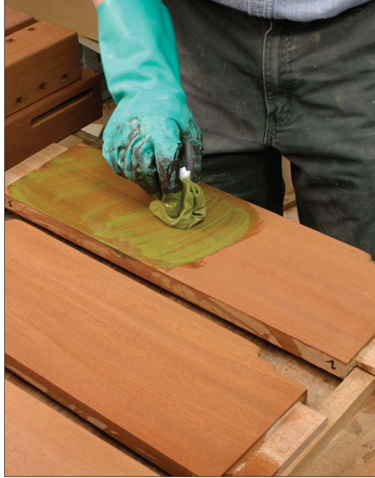
The solution of potassium dichromate oxides the mahogany, turns it a rusty orange color and gives it an aged patina. After this treatment, a green stain made of artist's oils and Danish oil is applied.
