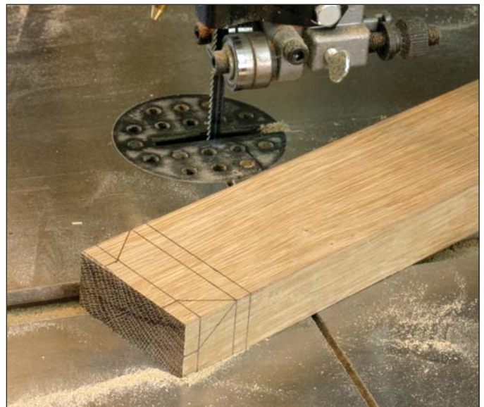
The trapezoid shaped block is laid out on each end of a long piece of wood to make cutting and handling easier.
