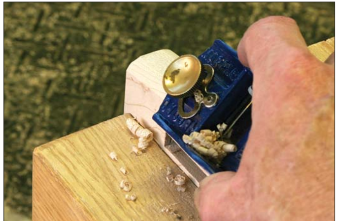
Fine on this side. The other side of the plane takes a small finishing cut. The amount of material removed and the quality of cut is controlled by moving the plane laterally.
