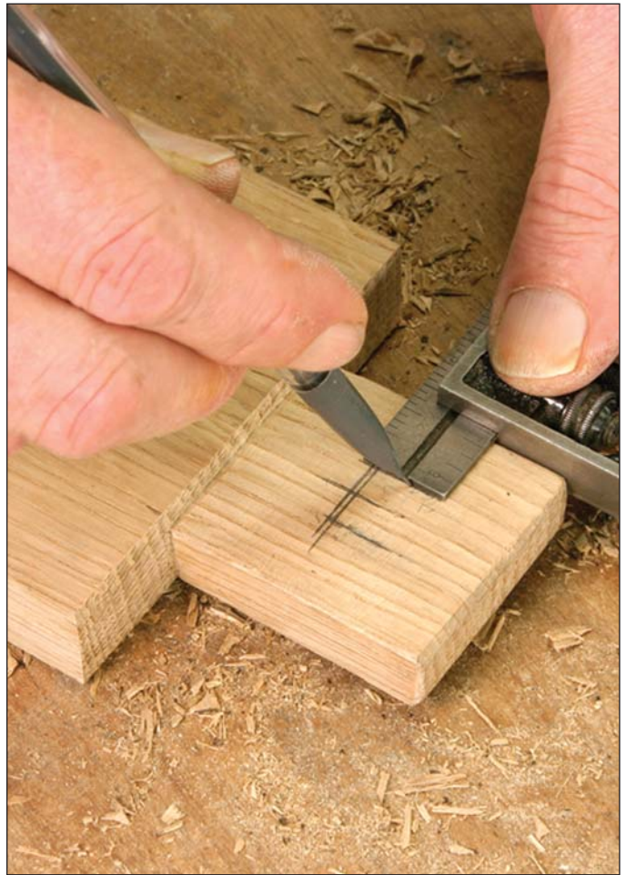
After fitting the through tenon, the location of the second mortise is laid out, keeping the back of the hole just behind the face of the rail.
