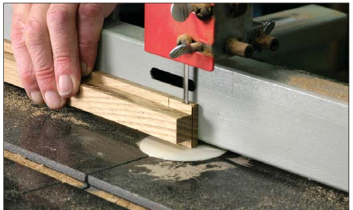
Wasting away. The band saw fence is set to leave just a sliver of material as the tenon cheeks are cut.
