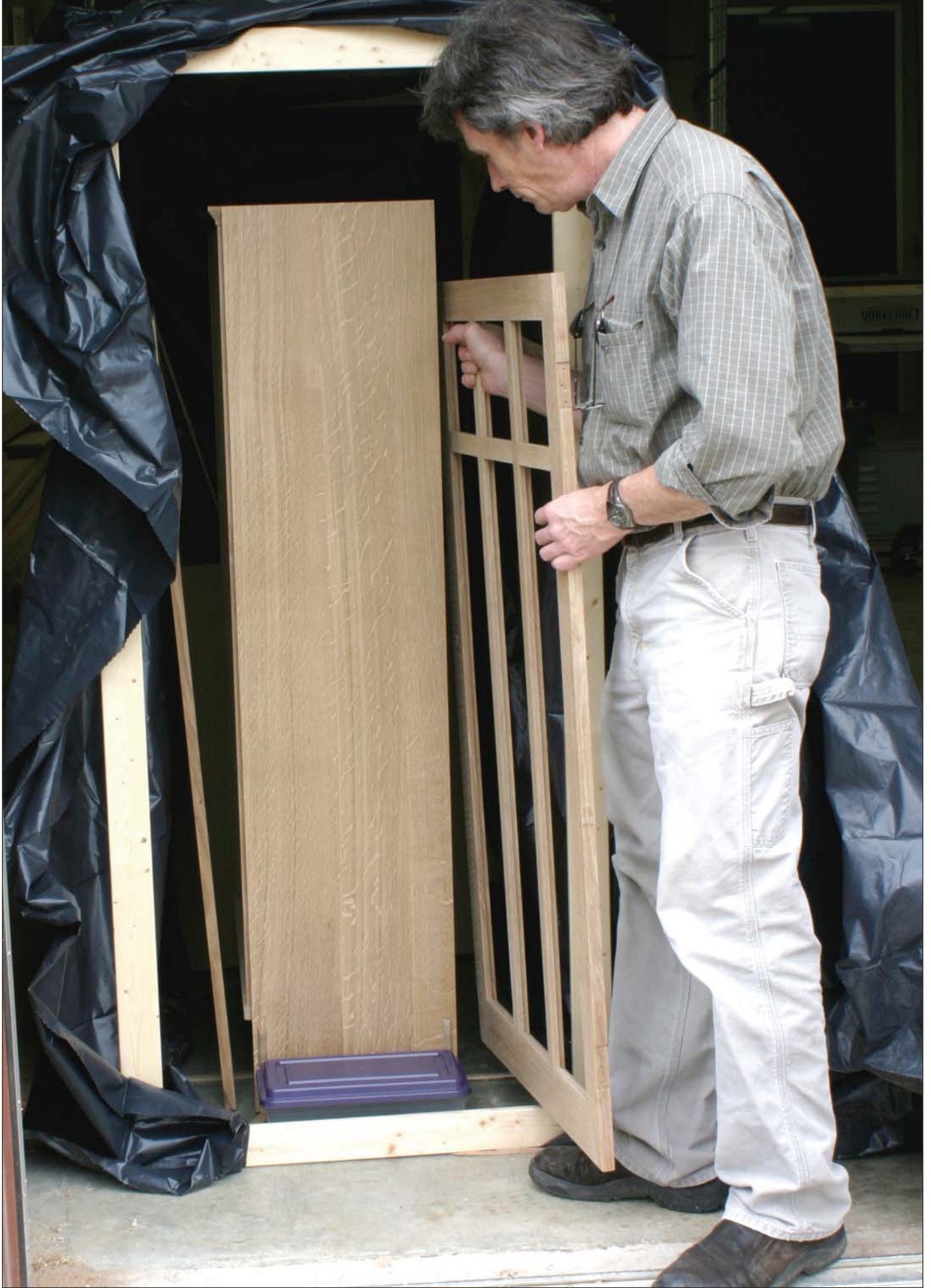
After sanding all of the parts, I placed them in an airtight fuming tent, located by the back door of the shop.
