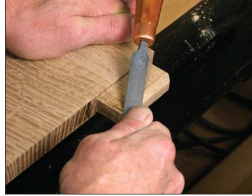
Refined detail. Make a slight bevel on the ends of the tenons before fitting. After a good dry-fit, mark the outside of the case on the tenon, then increase the bevels to end close to the line.
