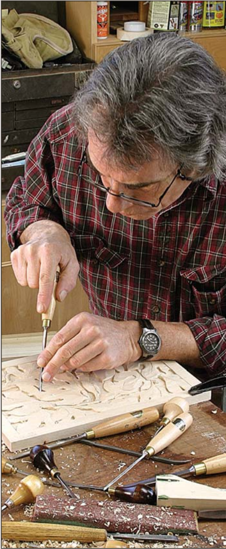
After tracing the pattern on the basswood panels, the design of sassafras leaves is carved.
