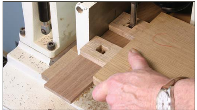
Back it up. A thin piece of scrap under the tenon provides support when making the second mortise.
