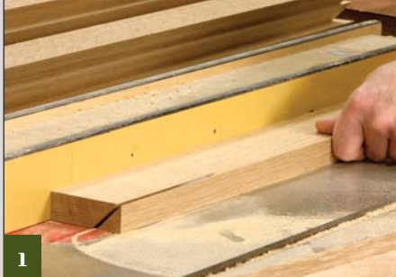
1 After ripping all the parts to finished width, cut a 45° bevel on both long edges of the thinner parts. Cutting the second bevel brings the part to its finished width.
