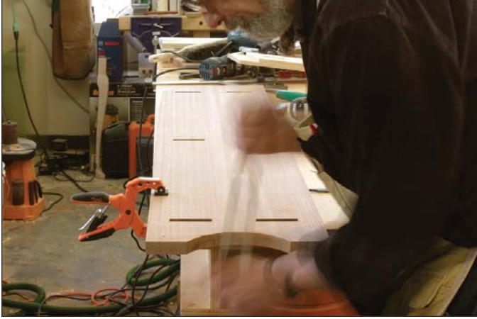
Getting in shape. After cutting the lower arch with a jigsaw, the curve is smoothed with a rasp.
