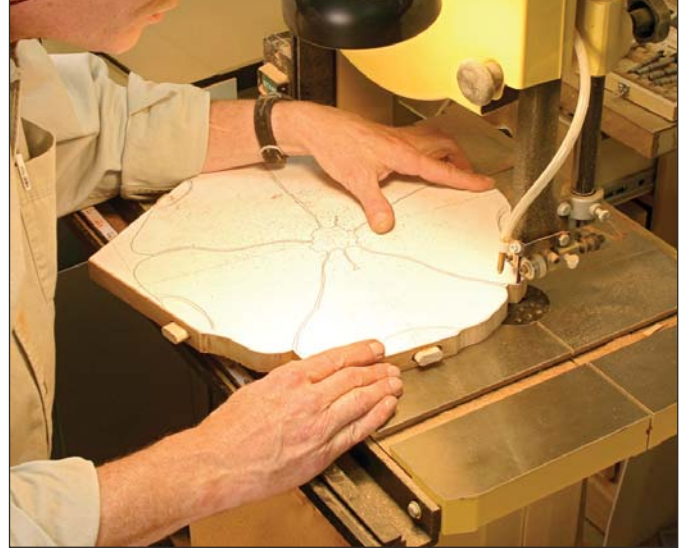
Rapid layout. Gluing a full-size paper pattern to the shelf blank eliminates transferring the pattern. The paper will stay in place through the cutting process.
