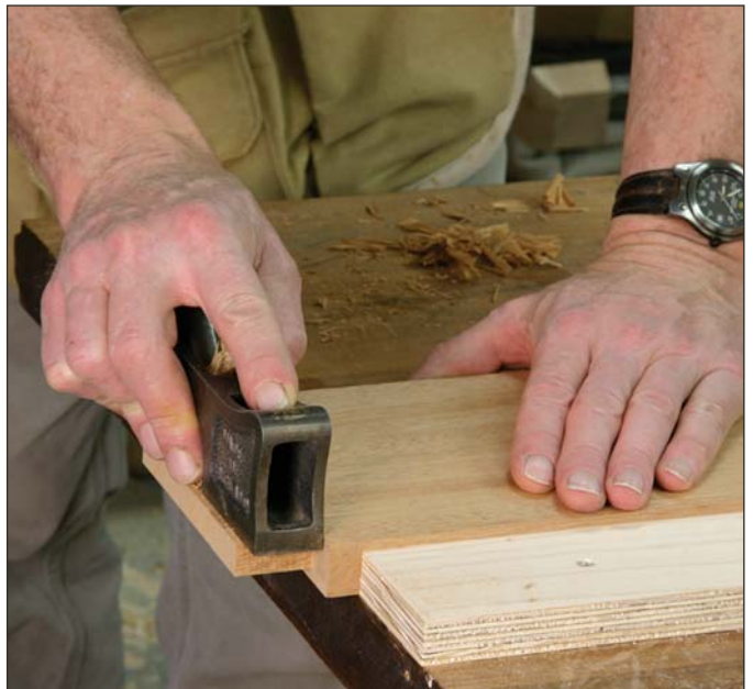
The tenons are adjusted to fit with my shoulder plane. A piece of scrap plywood attached to the bench acts as a bench stop to hold the work.
