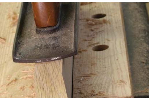
Nothing to see here. The glue line should disappear because the grain and color are the same in both pieces.
