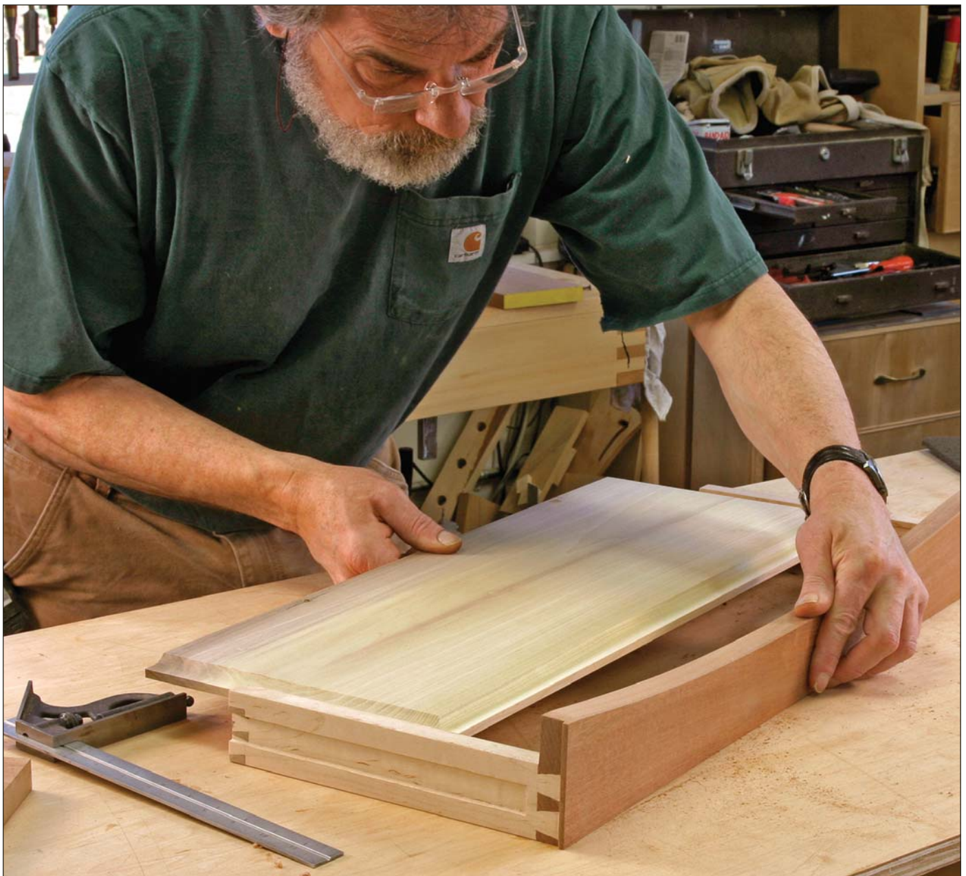
Sliding home. The drawer bottom slides past the drawer back and into grooves in the sides and front. Screws in elongated holes will hold the bottom to the back and allow the bottom to shrink or swell.
