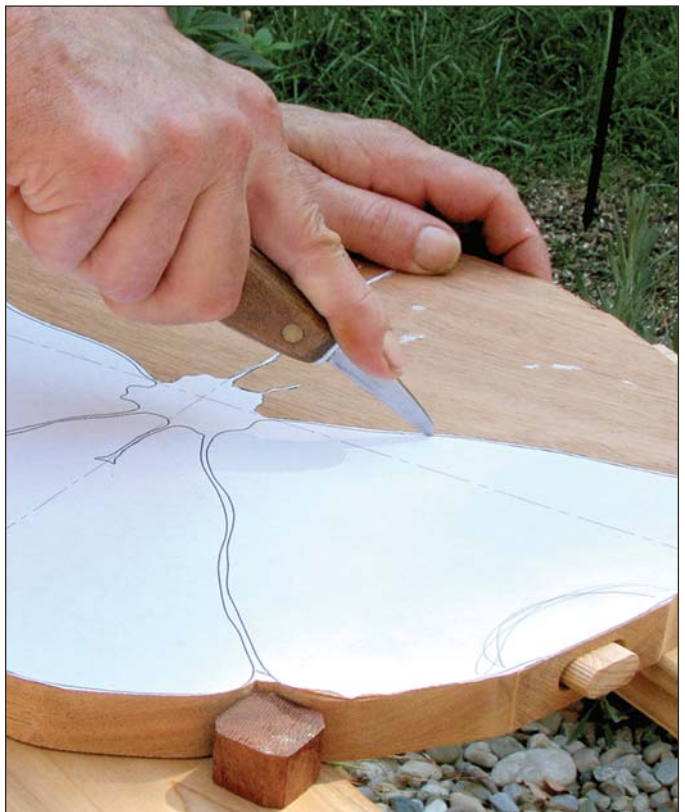
Taking a stab at marking. Cutting through the pattern with the point of a knife establishes the layout lines for the carving.
