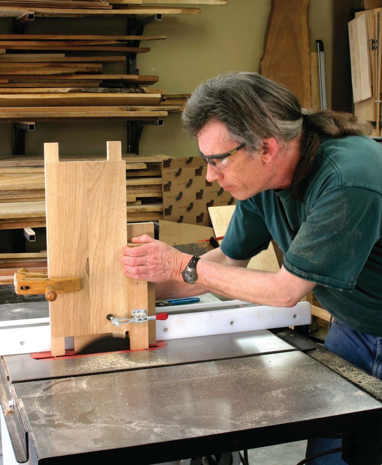
Cutting the shoulders. Use the tenoning jig to make the shoulder cuts on the through tenons. The clamp on the far end holds the workpiece to the jig.
