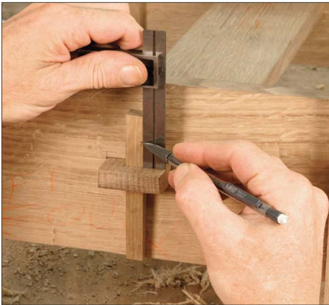
As the tenon key is fit, the length above and below the through tenon changes. I leave the key long and mark the length once I have a good fit.
