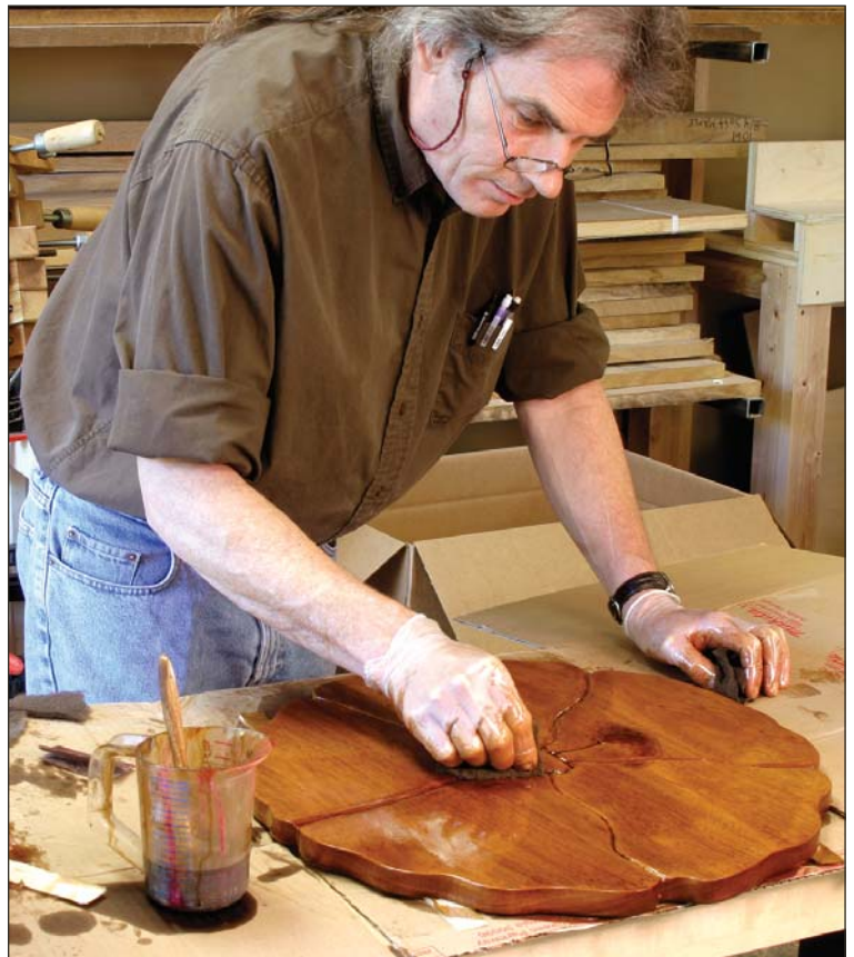
First coat. Dark walnut Danish oil helps to accentuate the grain of the mahogany. Two color coats were followed by three coats of natural Danish oil.
