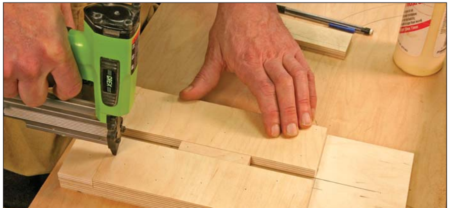
Built around the holes. This jig for the through-mortises is made by assembling small pieces to a backer. The openings are then cut with a router and a locating fence is added.
