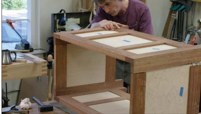
Assembling the front and back panels first simplifies the final assembly—putting the sides together results in a completed case.
