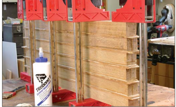
Thin veneers tend to buckle when clamped. Gluing them in a stack applies even pressure to keep them flat.
