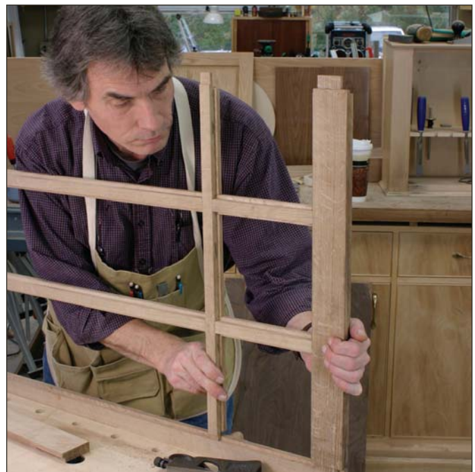
I assemble the door in stages. Here I'm placing a subassembly of the intermediate stiles and rail to one of the door stiles. The remaining stile will be placed on top and clamped.
