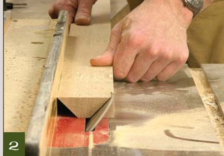
2 Be careful ripping the second bevel. After the leading edge clears the blade, use a push stick centered in the stock's width to move the material past the saw blade without tilting it.
