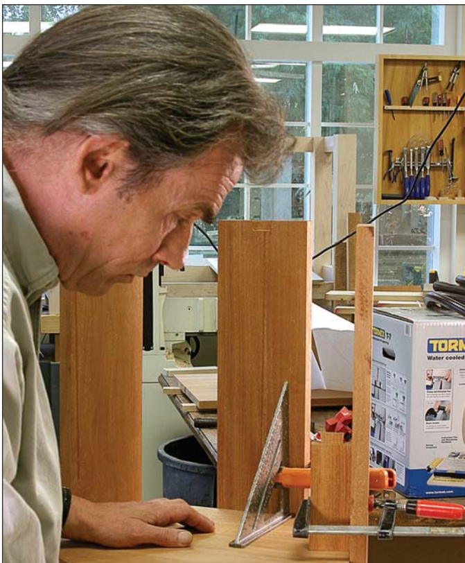
Straight fitting. All the joints were made and all parts dry-assembled before doing any of the shaping to the legs and shelf.
