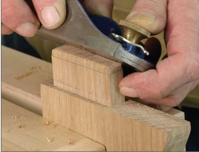
After the tenons are trimmed to fit with a shoulder plane and scraper, the exposed ends are rounded with a block plane.
