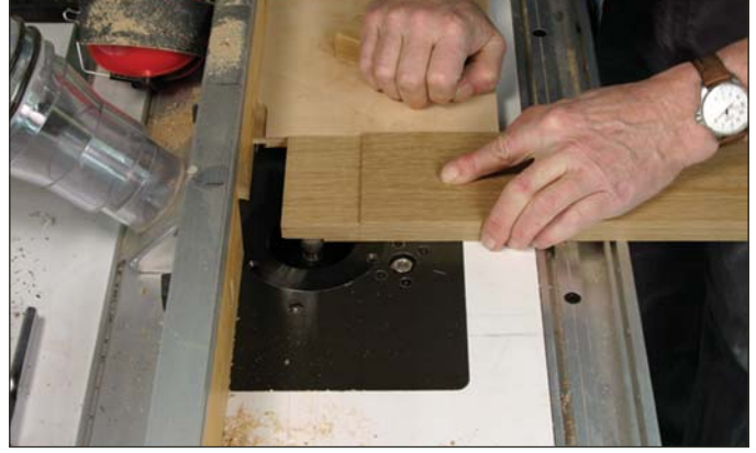
Got your back. Use a wide block to move the narrow shelves across the router bit.
