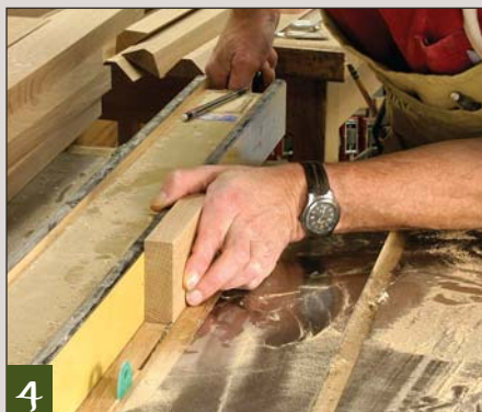
4 Set the distance from the blade to the fence by lining up the edge of a thin piece of stock to the left side of the blade. I use the saw cut in the table saw's zero-clearance insert as a guide.
