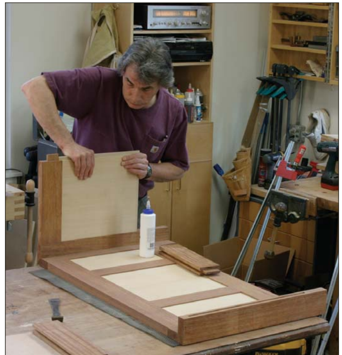
Rails and panels for the sides are slipped into the already-assembled back panel.
