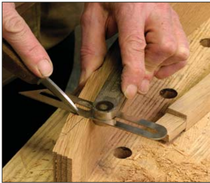
Around the bend. Mark the tenons all the way around the slat with a square and an adjustable bevel. Go over the lines with a knife before cutting the shoulders with a backsaw.
