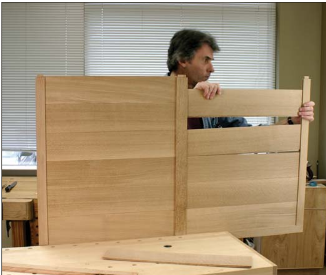
With the rails already glued to one stile, the shiplapped boards for the back panel are slipped into the groove in the rail. When they were all in place, I glued on the remaining stile.
