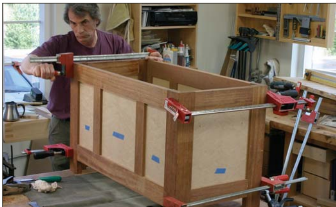
The assembled chest is flipped upright, the corners are checked for square and the case is clamped.
