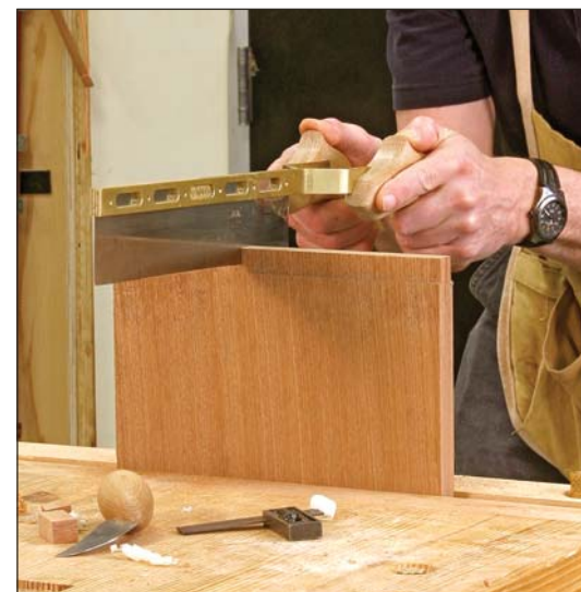
Ends second. The ends of the tenons are cut by hand, then the waste in between is removed.
