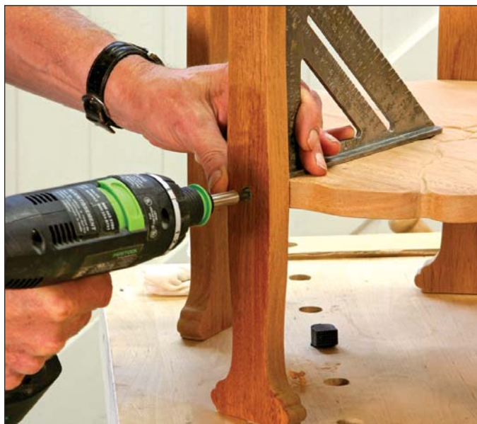
It isn't cheating. The original table had face-grain plugs in the faces of the legs. It is reasonable to assume that there are screws beneath the plugs. A Domino loose tenon reinforces these joints.
