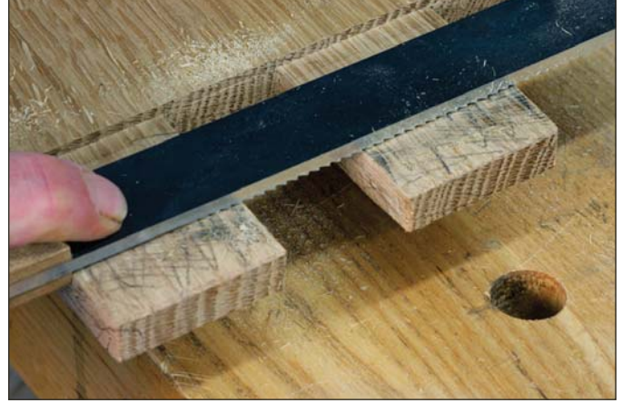
Off the top. The pencil marks indicate the high spots. Remove them with a float, then test the fit again.
