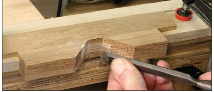
Double duty. This jig guides the bearing on a flush-trim router bit, then is used to guide a chisel to pare into the mitered corners.
