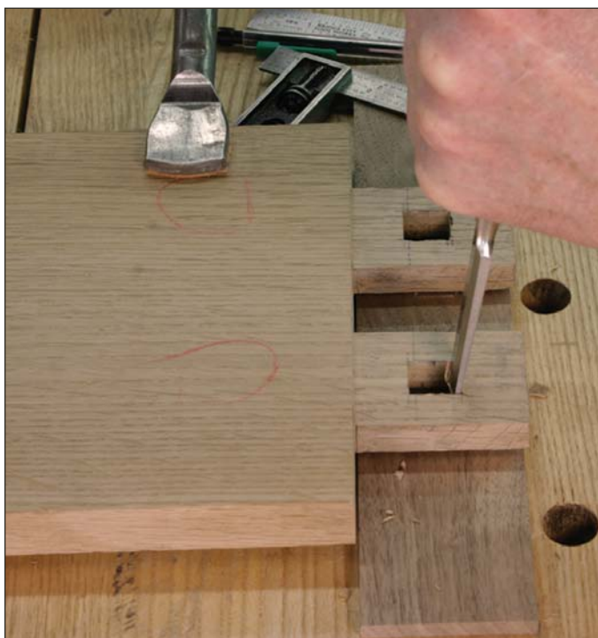
Angle by eye. Use a chisel to taper the end of the mortise for the wedge.
