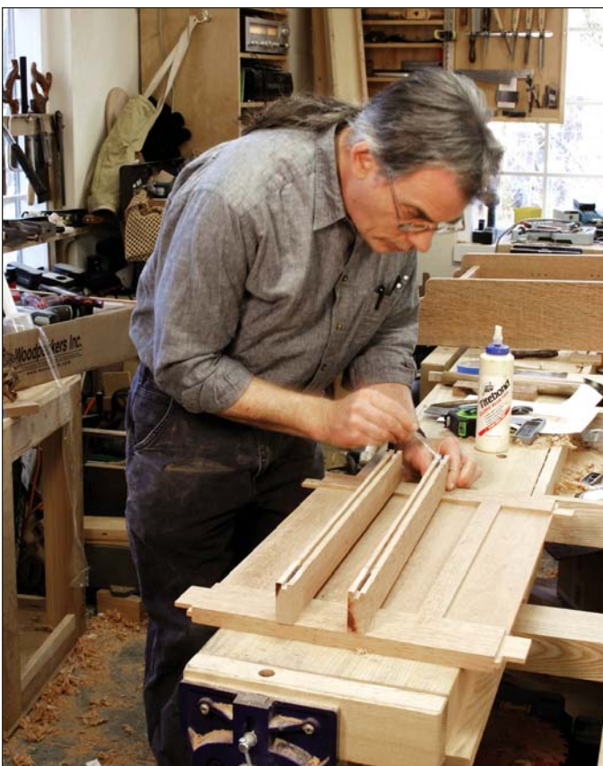
Two step glue-up. The center panel is put in place and the intermediate stiles glued between the top and bottom rails. After letting the glue cure, the outer panels are inserted, and the stiles are glued to the rail ends.
