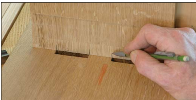
From the source. Mark the ends of the tenons directly from the mortises.
