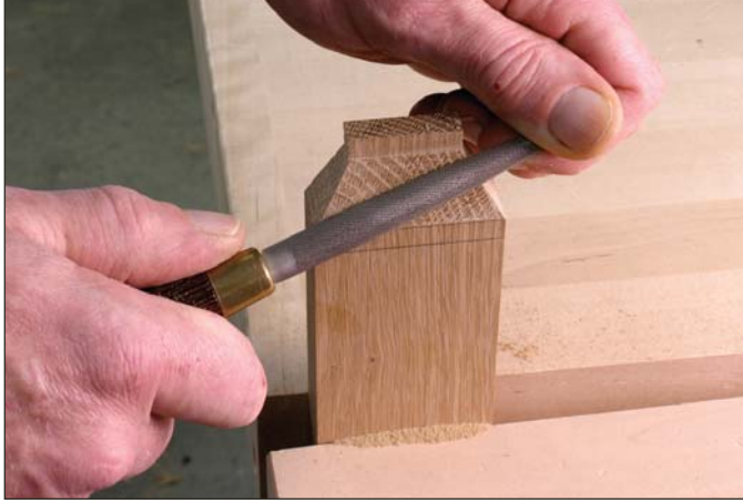
Leaving the block attached gives me plenty of material to clamp in the vise while I smooth out the saw marks with a rasp, followed by a file, and then #150-grit sandpaper.
