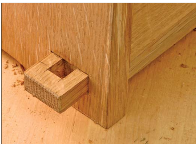
Just a bit behind. The back edge of the second through mortise is back from the face of the end \frac{1}{16} ". The tusk will then be able to pull the joint tight.
