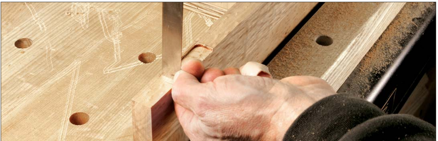
Final cuts. The router leaves a flat bottom and a straight back edge to the hinge mortise. The rounded corners, however, need to be removed with a chisel. Knifed-in layout lines provide a reference for the chisel.
