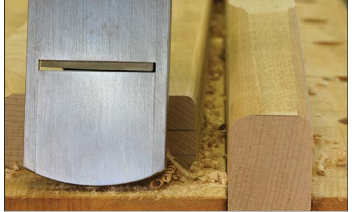
Why this slides. Opening the mouth of the block plane provides room to skew the iron.
