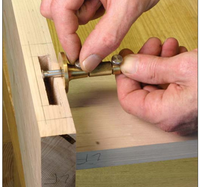
Better than numbers. Setting the marking gauge directly to the edge of the mortise ensures exact alignment of the rail and leg.
