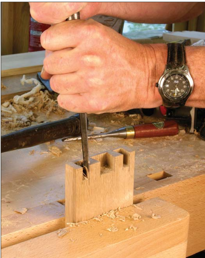
After routing most of the waste, I use a chisel to pare the pins down the rest of the way. The router quickly establishes a consistent depth.
