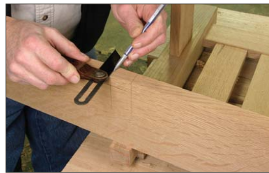
Follow around. An adjustable bevel transfers the layout lines for the angled mortise from the top of the arm to the bottom.
