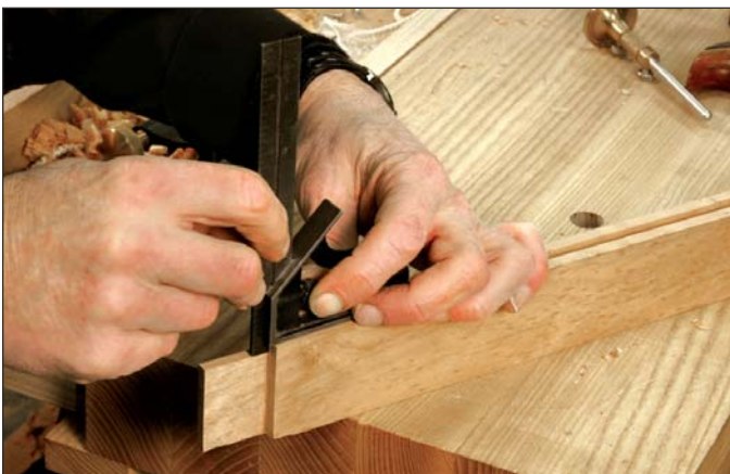
Drop-in measurement. With the adjustable square sitting on top of the groove in the stile, the blade is bottomed out to obtain the exact measurement for the depth of the groove.
