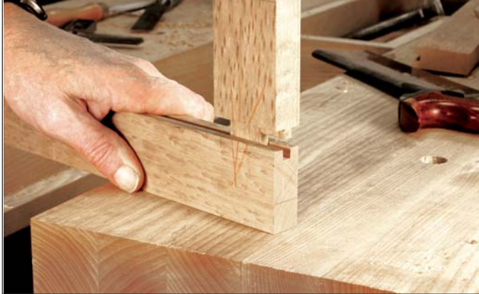
Double duty. The haunch fills the panel groove on the outer edges of the door. It also will keep the stile and rail faces aligned if the wood warps.
