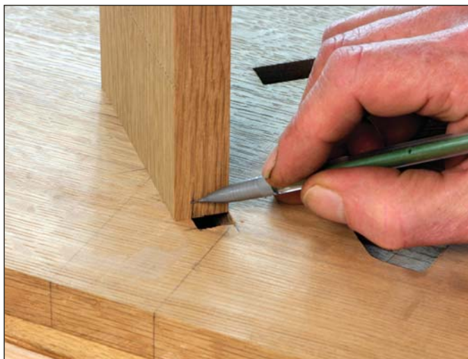
On your mark. Use the mortise to determine the exact thickness of the tenon.
