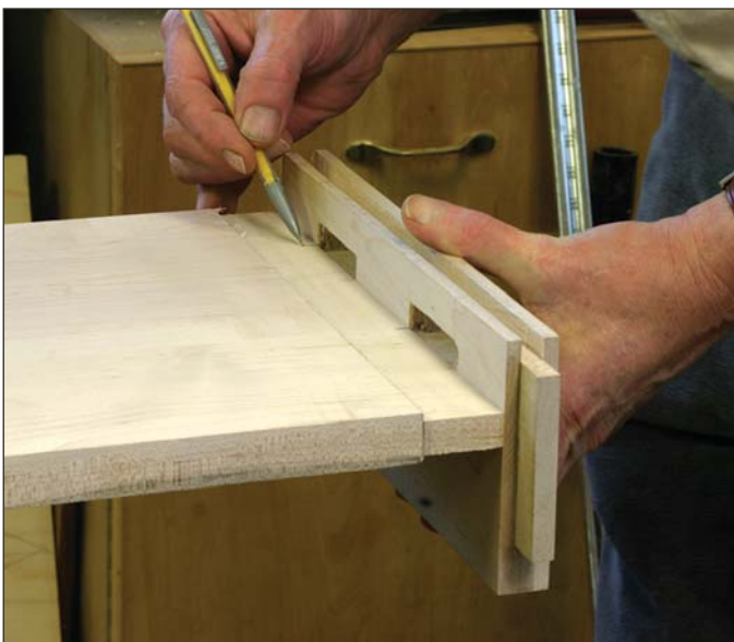
Where it belongs. Marking the tenons directly from the mortises is faster and far more accurate than measuring.
