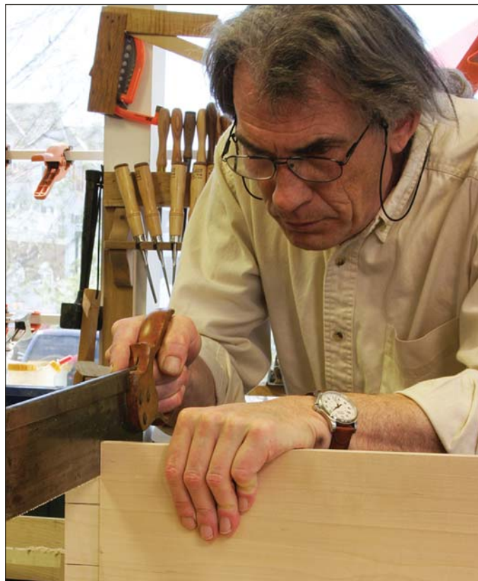
Easier by hand. These cuts could be made at the table saw, but that would be an awkward operation. Cutting the tenons by hand allows me to see what is going on.
