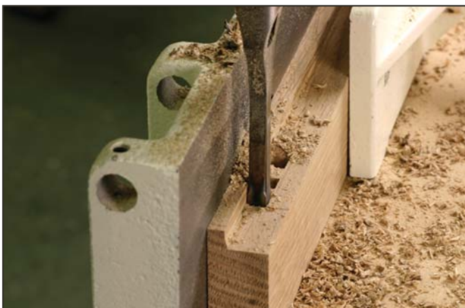
Simple setup. Set the fence on the mortiser by lining up the chisel with the back of the rabbet.
