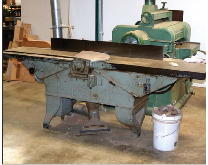
Not many one-man shops have a 20" jointer like this vintage machine, but then again, not many one-man shops produce work at the level of quality and detail that Jim Ipekjian does.
