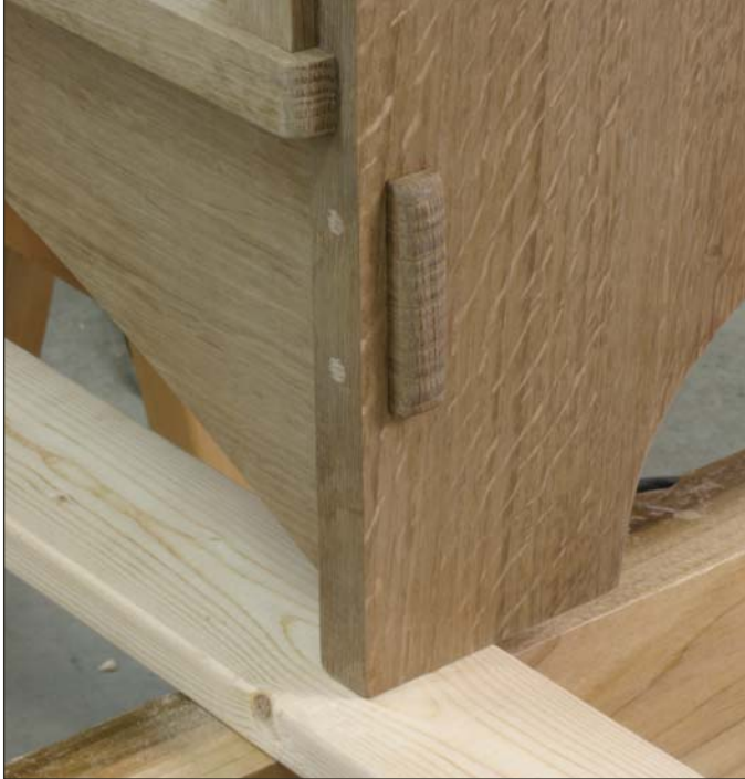
After exposure to ammonia fumes for 24 hours, the oak has turned a grayish brown color.
