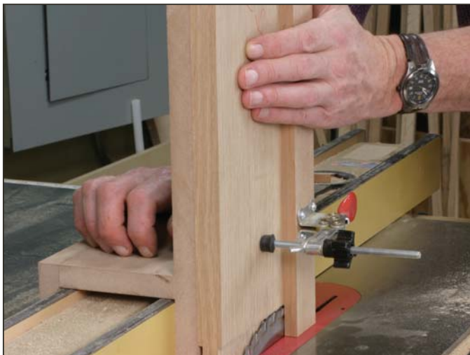
The long mortises on the ends of the rails are cut with this tenoning jig that rides along the table saw fence.
