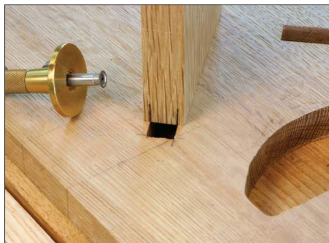
Check & go. Mark from both sides to center the tenon and adjust until the parts match.
