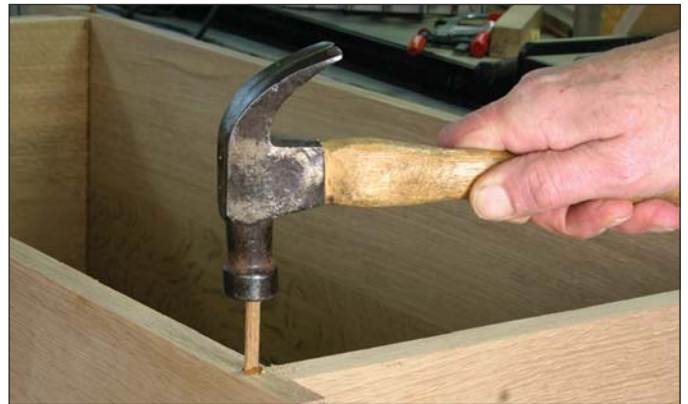
Overkill. The dowel reinforces the through mortise and tenon joint. It isn't needed, but it's a nice detail to include.
