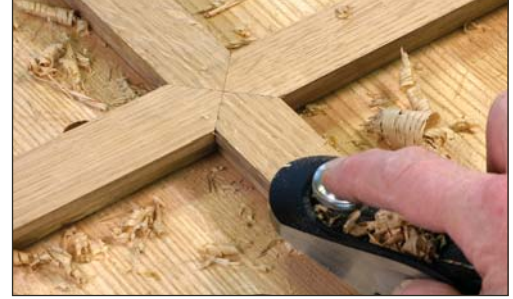
Payday. Flush the surfaces of the completed joints with a sharp block plane, and take a moment to feel proud. Then get back to work; there are a bunch of these.
