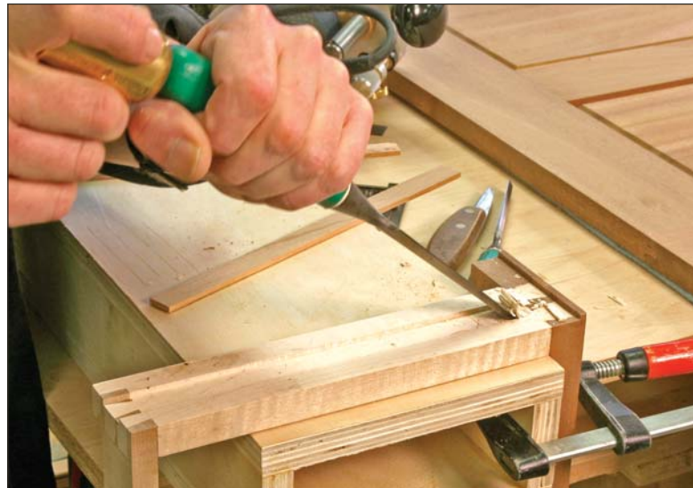
Hidden away. The hidden drawer rides on wooden slides attached to the carcass. The end of the groove will act as a stop for the runners, and needs to end in the right spot.
