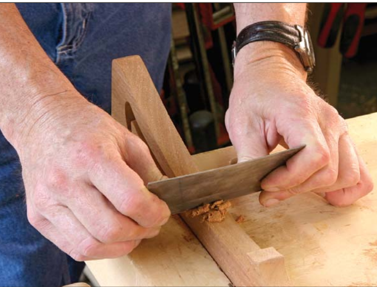
A close scrape. The hand-stitched rasp will leave shallow, narrow grooves. A cabinet scraper follows the rasp to remove the high spots between the grooves and leaves a fine surface.
