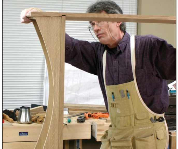
After spreading glue on the end of the bottom, and the cheeks of the tenons, the remaining cabinet side is carefully put in place.
