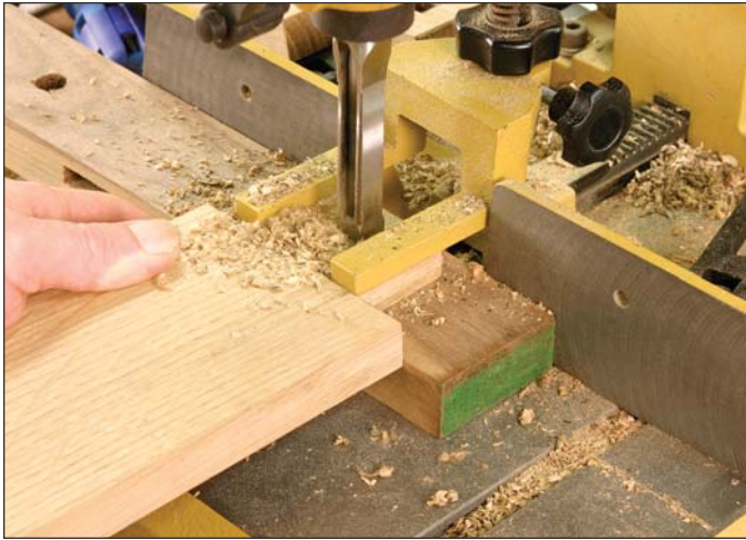
The mortise is cut with one plunge of the hollow-chisel mortiser. A piece of scrap below the cut supports the tenon, keeping the wood from breaking on the back side.
