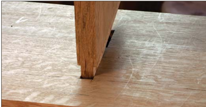
Now you know. Aim for a snug fit by testing a corner of the tenon in the mortise after routing the cheeks.
