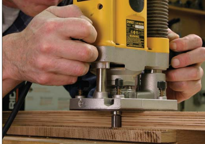
Under control. Cut the tenon shoulders first, using a straightedge and a bearing-guided router bit. Adjust the depth of cut in small increments to achieve the proper thickness.
