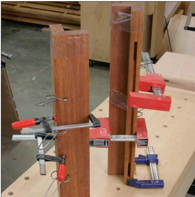
Strips of clear packing tape across the joint let the miters fold together. More tape and additional clamps provide a tight, strong joint.
