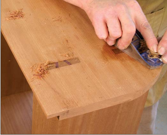
Soak then shave. After sawing off the wedges, the joints are soaked with paint thinner to make it easier to trim the end grain flush.
