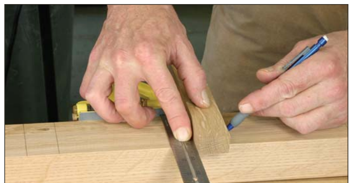
The real thing. A scrap of muntin stock is held against the square to mark the stiles. This speeds the process and ensures accuracy.
