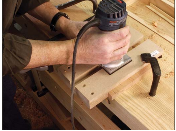
Stop action. A pencil mark indicates the end of the dado, and because the router will leave rounded ends, I stop just short of the mark.
