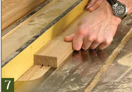
7 With the blade height and fence settings adjusted, cut two grooves in the back of the thicker leg parts.
