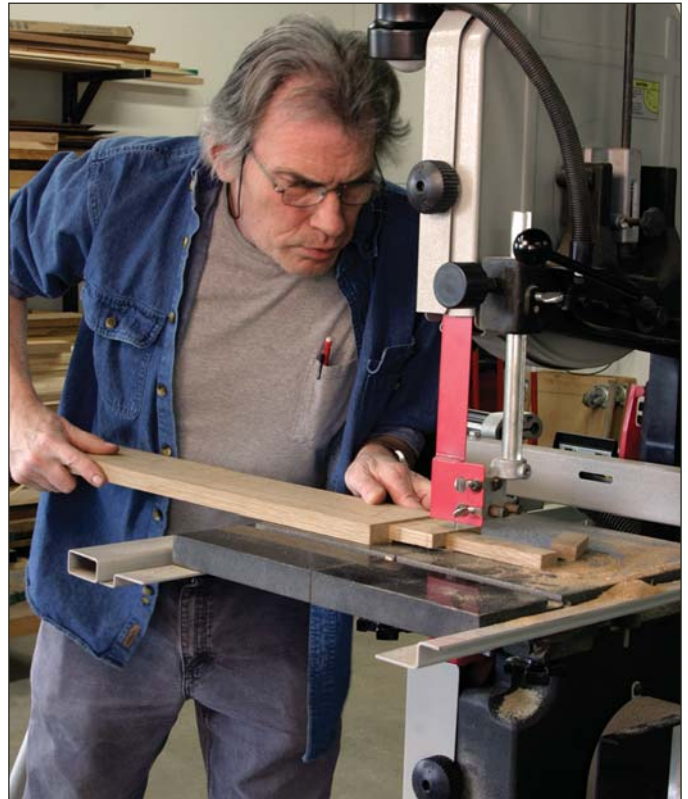
Stop in time. Cut the end of the tenon, but stop just short of your shoulder line.
