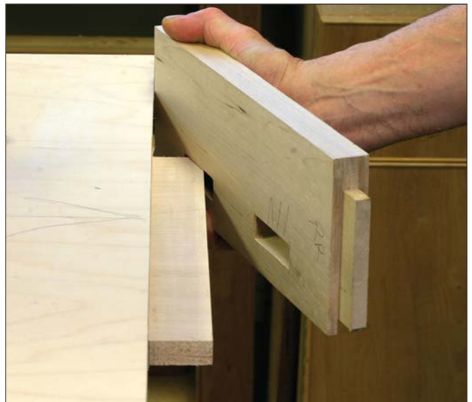
When to stop. When a corner can be forced into the mortise, the thickness is close. Then it's time to cut the edges of the tenons.
