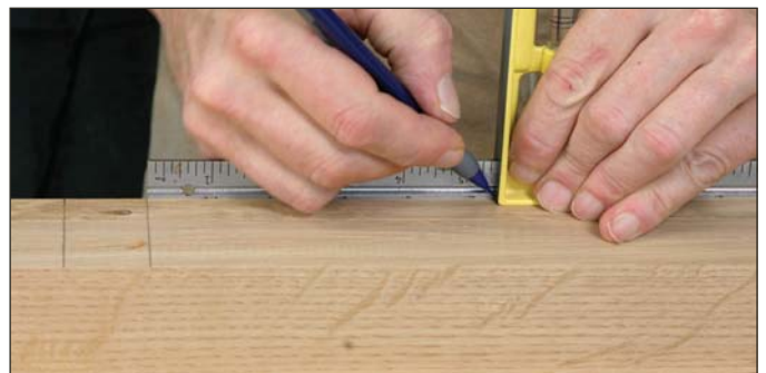
Better than numbers. A combination square does an excellent job of laying out repeating spaces, in this case the openings in the door.
