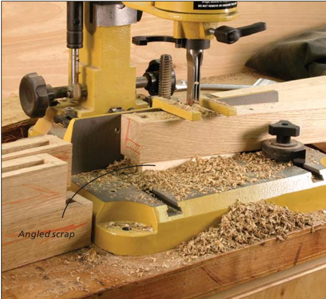
An angled block of scrap wood tilts the leg to cut an angled mortise parallel to the top of the leg.
