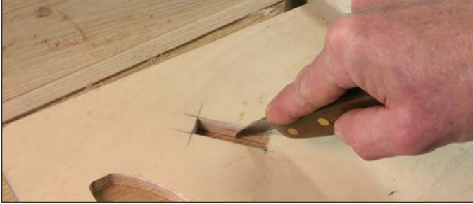
Score first. Prevent tear-out by scoring around the openings before cutting with the router.
