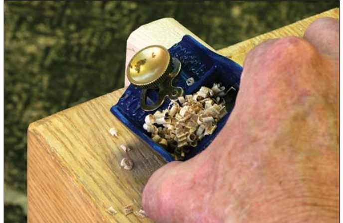
Big mouth, quick work. This side of the plane will take a coarse cut, removing a lot of material in a hurry.
