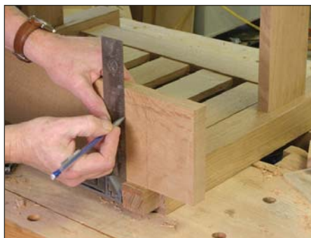
Can't miss. Balance the arm on the base assembly and mark the location of both the front and back tenons without moving the arm.
