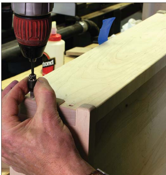
Waste removal: Follow with a drill through the hole in the punch body. This removes the waste within the square recess.
