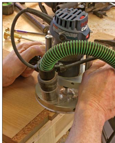
Shoulders first. A shallow rabbet is cut on each side of the shelves to start the making of the tenons.
