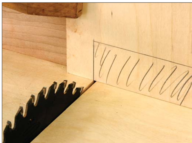
Nothing to chance. The saw kerf in the horizontal part of the jig shows exactly where the blade will cut. With the layout line at the kerf line, clamp the piece to the jig.
