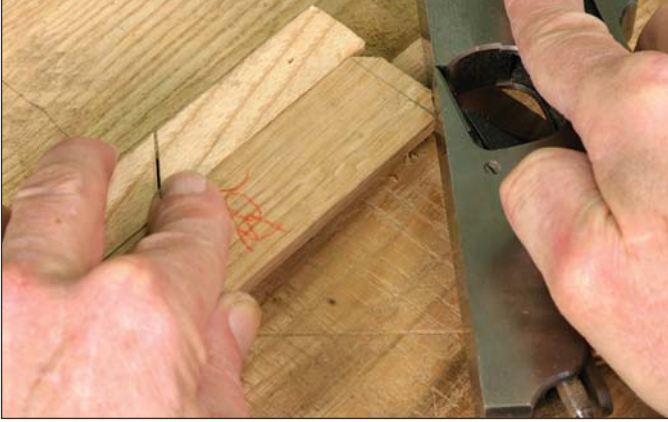
Complex geometry. Test the fit often while fitting the miters. Trimming one edge will lengthen or shorten an adjacent edge as well.
