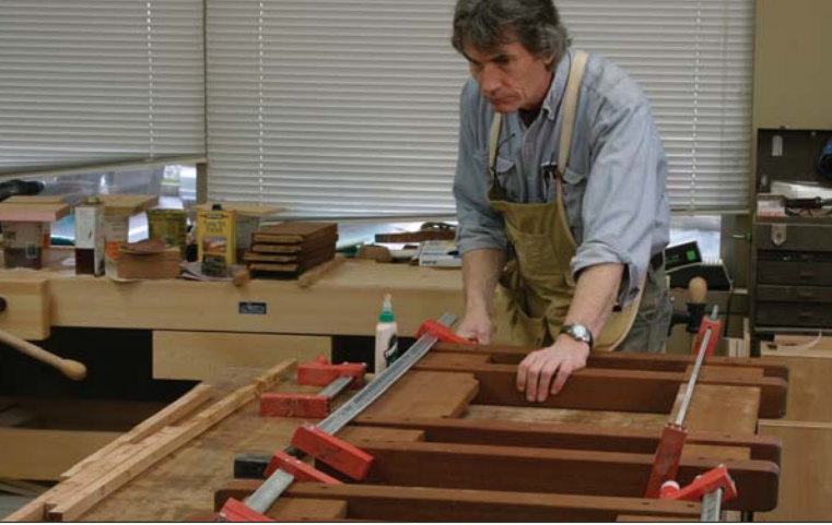
Once the coloring of the wood is complete, the table base is assembled in stages. Here I'm gluing the center rails between each subassembly.
