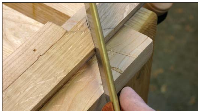
On the right side. For the points of the miters to meet, the saw cuts must be on opposite sides of the lines on each side of the mullion.
