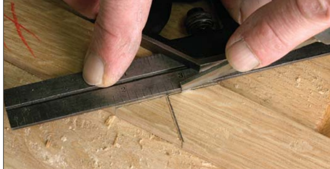
X marks the spot. The joints in the central mullion meet in the exact center. A knife cut along the lines will help to guide the saw.
