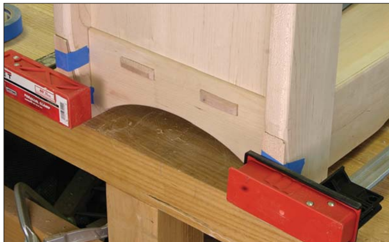
Tape for the tapers. Offcuts from tapering the legs are taped in place to provide a flat surface for the clamps.
