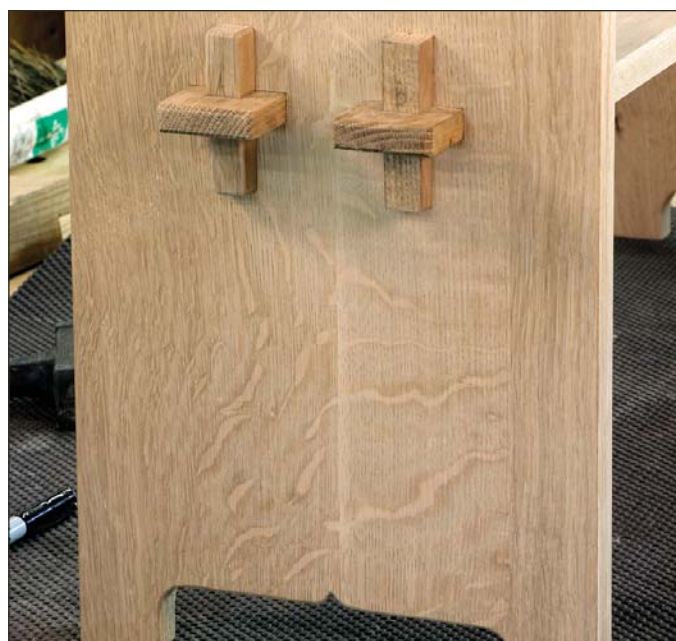
Hard & soft. Edges on the tenons and keys are beveled, but they fade away to leave clean lines at the joints.
