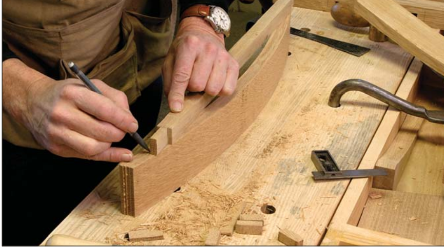
Stick with it. Make a pattern on scrap to lay out the tenon locations on the curved back rails. Hold the stick in place and mark both ends without moving the stick.
