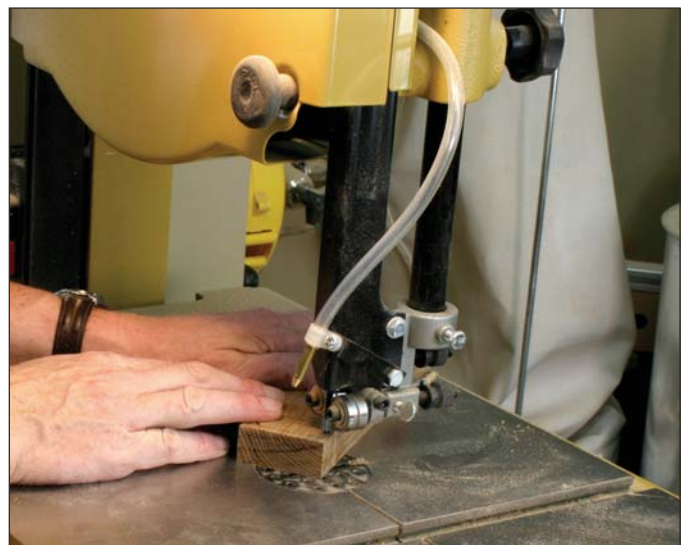
All of the cuts to form the capital block were made on the band saw, as shown here. The final cut will be made after the block is smooth.
