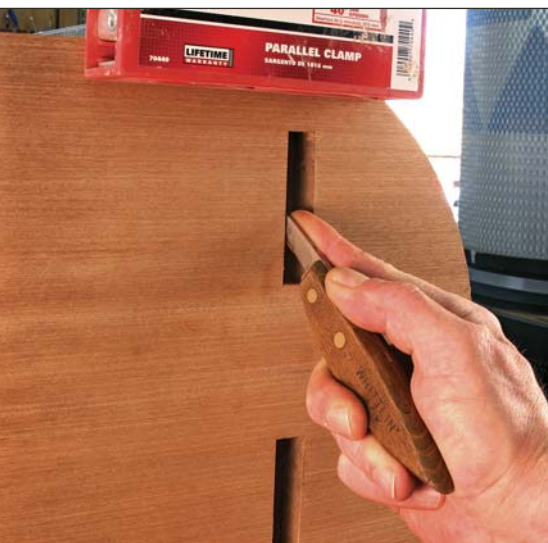
Marked in place. The tenons are marked directly from the mortises, ensuring that the locations match.
