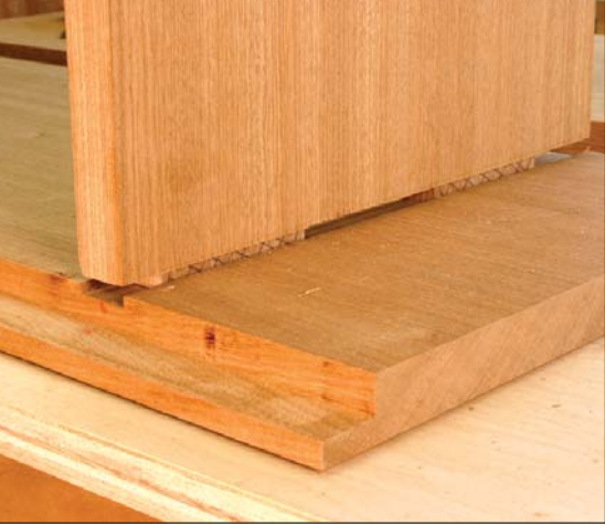
Test, don't guess. Pencil hatch marks on the tenons will smear and reveal tight spots within the joints during the test fitting.
