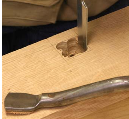
Pare to plumb. The same wedge is clamped between the arm and the bench to pare down the walls of the through-mortise.
