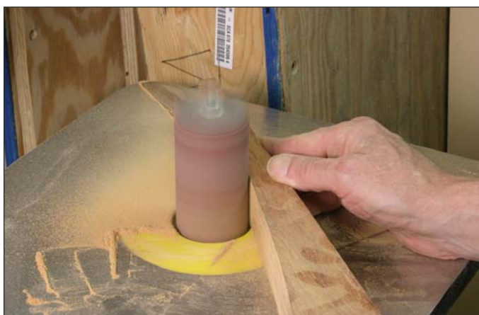
After cutting, the edges are sanded with the stack still stuck together.
