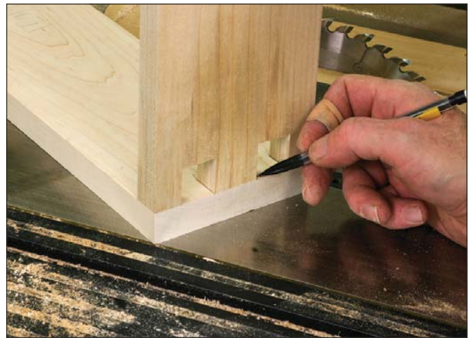
Balancing act. After cutting the first set of fingers, place the end of a side on the drawer front to mark the matching parts of the joint.
