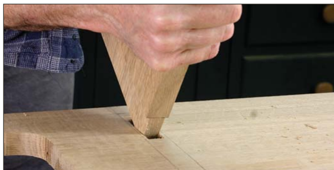
First things first. Test the thickness of the tenon by placing a corner of the shelf in the mortise. Aim for a tight fit at this point.
