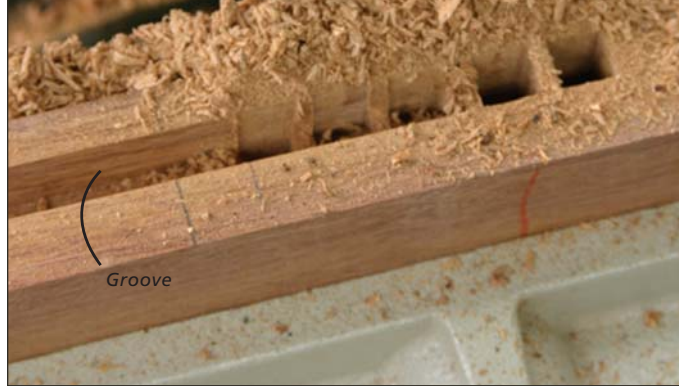
The mortiser is set with the chisel flush with the panel groove. Plunge the bit and chisel to make distinct holes, then come back and clean up the waste in between.
