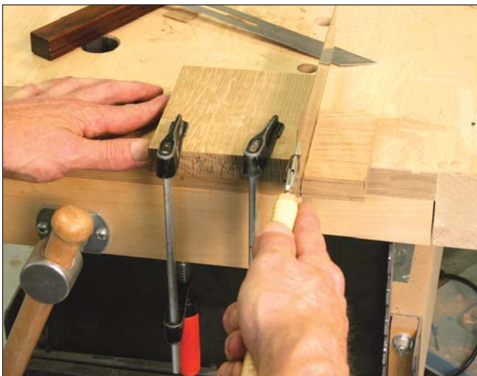
These angled shoulder cuts would be tricky to make with power tools.
