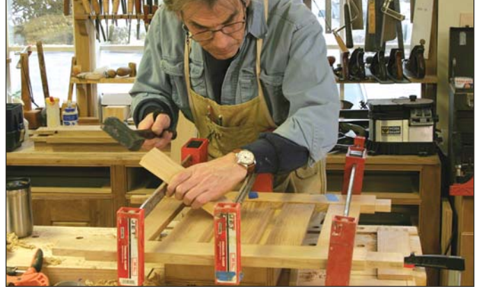
Only if you have to. Because the lower end of the vertical slats are angled, they only fit in one place. They can be adjusted with a tap or two.
