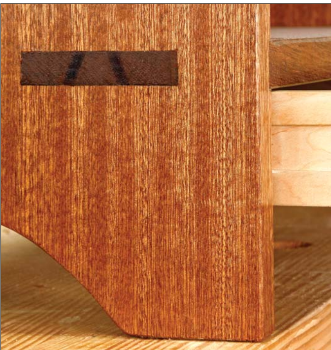
Now you see it. The rabbet in the end of the drawer front provides clearance for the sides, while allowing a narrow margin to be trimmed easily.
