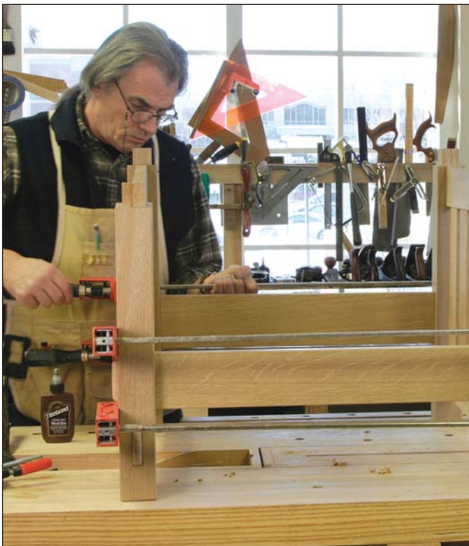
Stress management. With the sides glued into units, the last stage of the base assembly is a simple matter.
