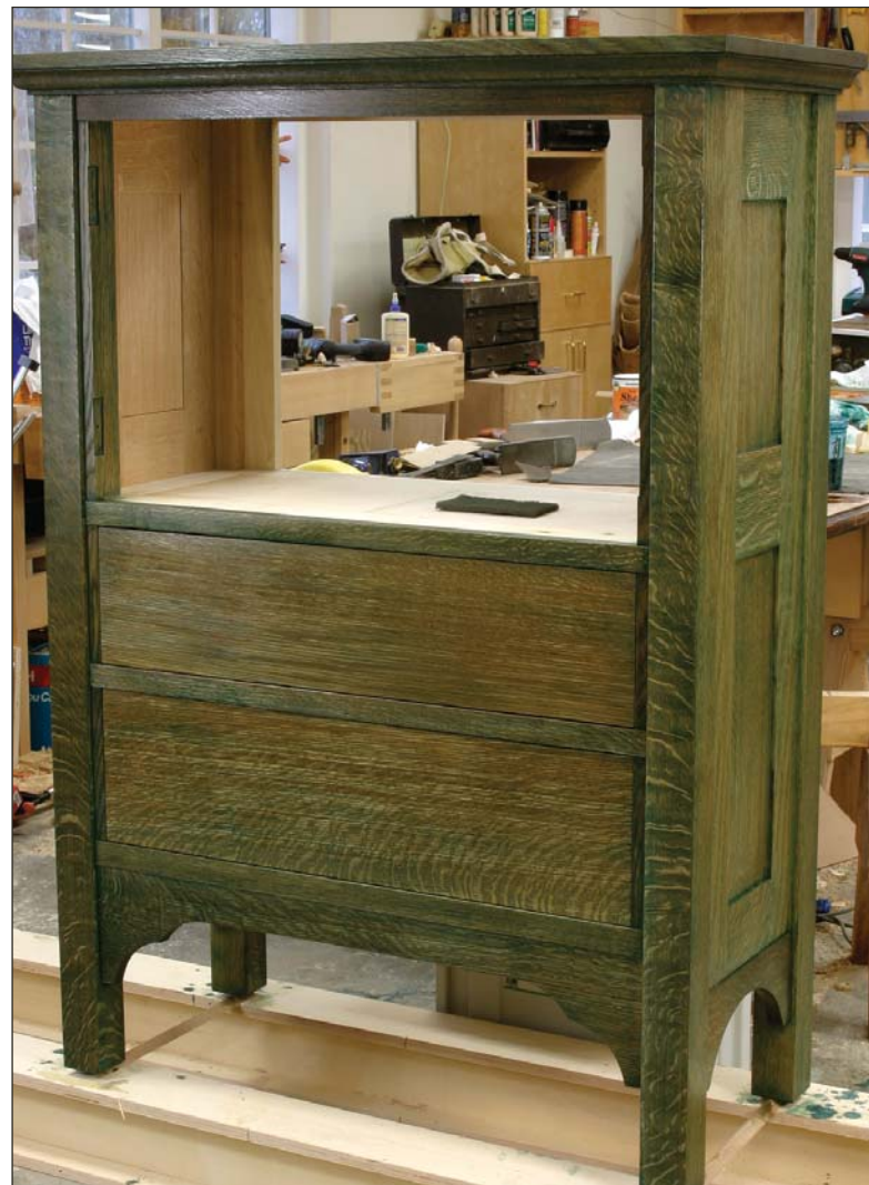
The stain is followed by a coat of natural color Watco, which lightens the color and highlights the figure of the quartersawn wood.
