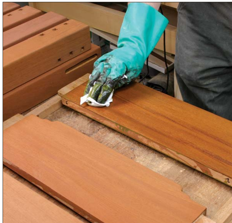
After wiping off the excess, the mahogany is left a rich, reddish brown color. This is the same technique used in original Greene and Greene furniture. After the stain dries, three additional coats of oil are applied.
