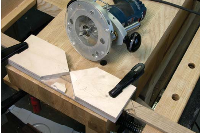
Step back and consider. The router jig is mainly to provide a flat bottom for the lap joint. Set the fence to keep the bit on the waste side of the saw cuts.
