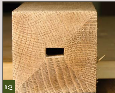
12 The completed legs have a small rectangular hollow in the center, and show quartersawn figure on all four sides. This is a stable assembly, relatively quick to make and easy to assemble.
