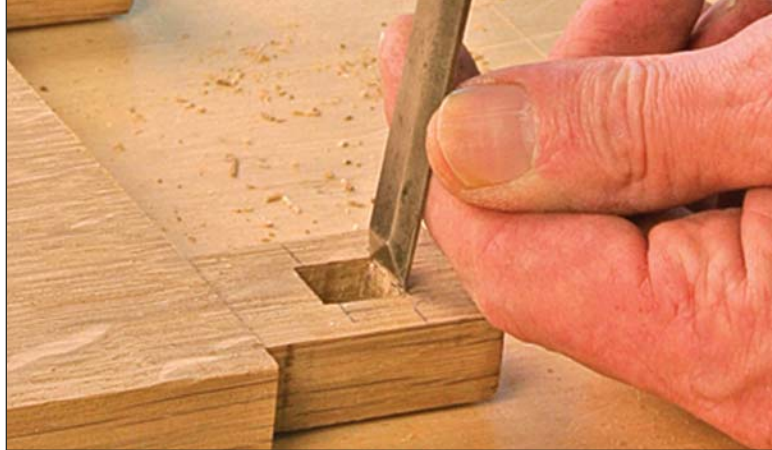
Eyeing the angle. Set the chisel on the line and lean the chisel back until the edge is in line with the bottom of the mortise. Strike the chisel with a mallet to complete the cut.
