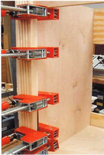
21 Glue and clamp the spacer strip in place.
