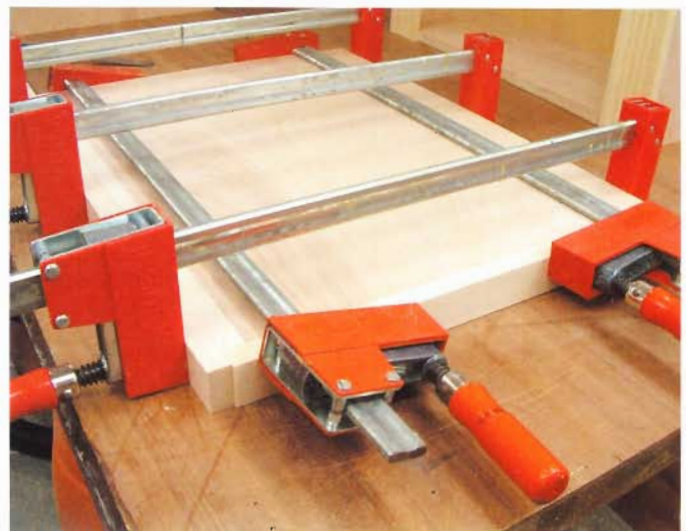
16 Cut the edge strips to fit the tops and glue them to the edges of the tops. See the illustration for top details.
