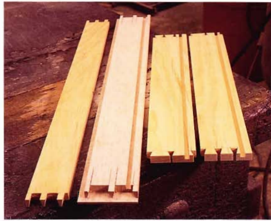
17 Now build the drawers for the lower section of the entertainment center.
