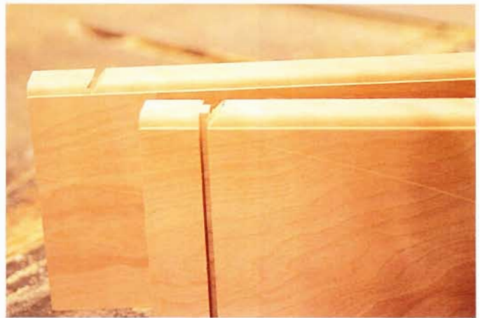
19 Set the blade to 45°. Cut just to the shoulder of the roundover cut on all rails (a single pass creates the tenon area) and stiles (nibble away for the mortises). Reset the blade to 90° and complete the tenons.
