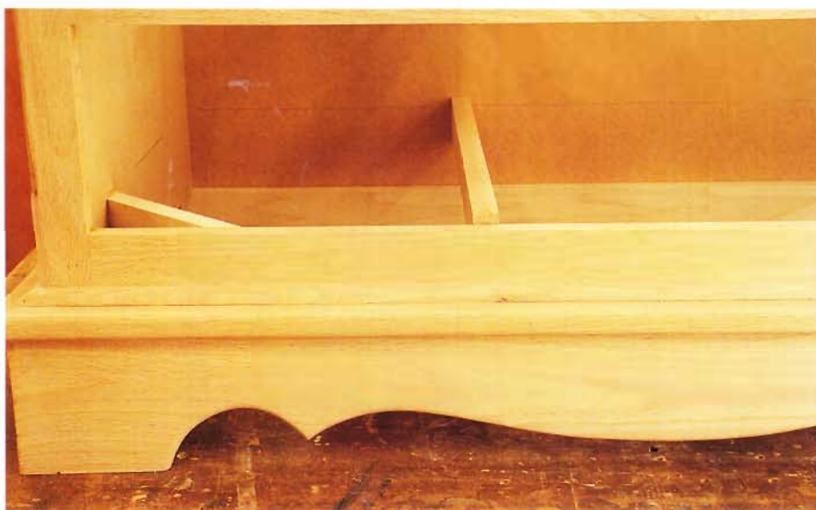
8 Using glue and nails, install two 8"-long 45° braces in the front lower left and right corners of the base cabinet, as shown.
