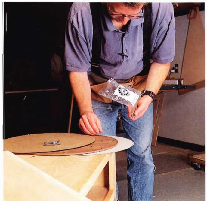
Put the ball bearings in the holes in the Masonite and place the top onto the assembly. Tie the whole unit together with a washer and wing nut. You should be able to rotate the lazy Susan and not see the bolt move.
