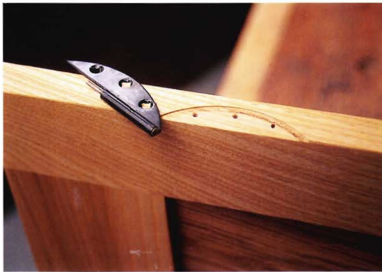
23 Above is a detail of the mortise and hinge.
