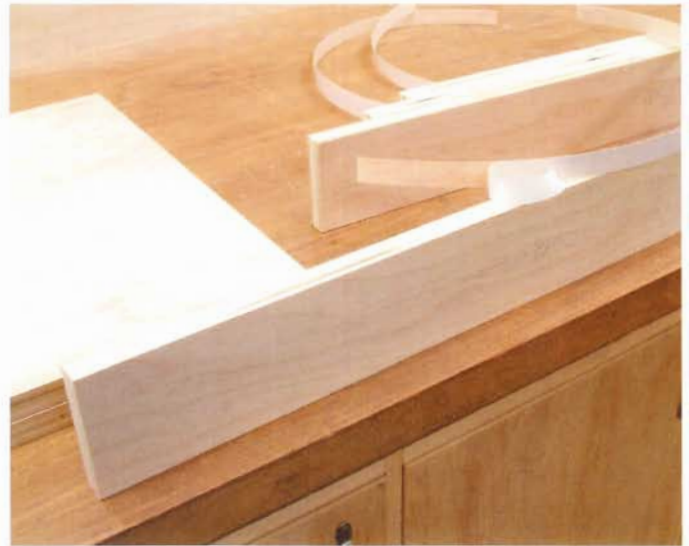
2 Edge-band all the parts that require it. Self-adhesive wood veneer edge tape is the best material to cover the edge grain of plywood.
