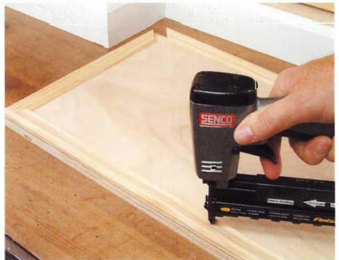
25 Reattach the cabinets to one another. Glue the dentil moulding assembly to the \frac{3}{4} "-wide front rail on the center cabinet. Double-check the measurements for the doors. Cut out the doors, then cut the plywood edge moulding to fit the faces of the doors. (The plywood edge moulding used on the doors has a lip on it. It is called plywood edge moulding at the home-improvement center. This lip is cut off before it is used on this project. See illustration for a detailed drawing.) Glue and staple or nail it in place. Hold the moulding flush to the edges of the doors.
