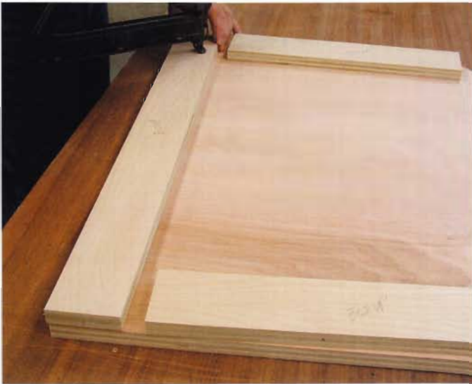
1 Lay out the top and cut it to shape. Glue and staple (or attach using screws) the buildup strips to the bottom of the top.
