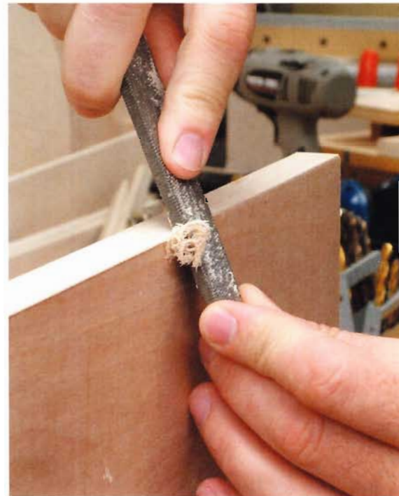
4 Trim the edges of the tape with a file and sand smooth.
