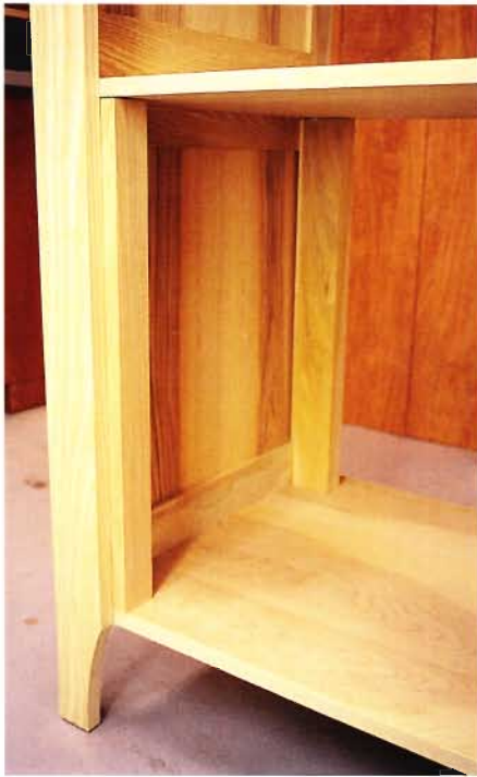
17 Install the front and rear drawer spacers on each side of the cabinet.
