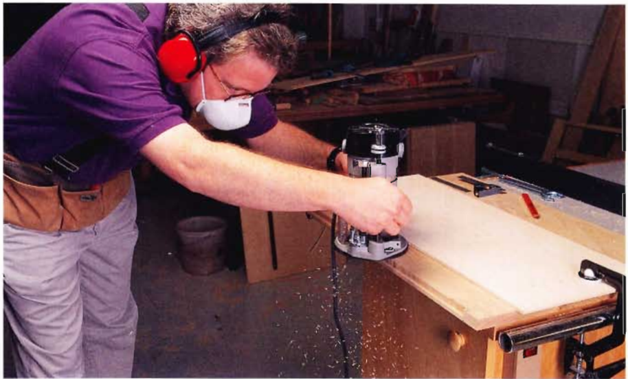
Cut a stopped rabbet in the rear edge of the top for the back. Then cut the \frac{1}{2} " \times \frac{1}{4} " rabbet in the rear edge of the sides for the back. Do this with a clamped-on straightedge and a router.
