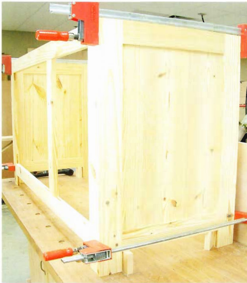
9 The end panels are assembled at the same time. When the legs are part of the framework, the cabinet casework comes together quickly.
