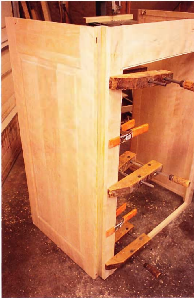
26 When set, glue the front face frame to the other leg of the L-corner, creating the quartered column area.
