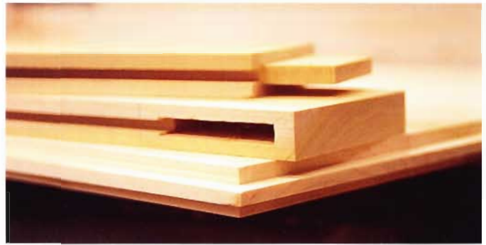
27 Mill, cut to size and assemble the top and bottom panels as well as the two shelves. All are made in the same fashion, with the front and back pieces being the stiles and the ends being the rails.
