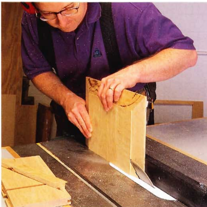
Set your table saw to about 12° to cut the bevel on the door panel. Leave a little less than \frac{1}{4} " thickness on the edge of the panel. The panel should be \frac{1}{16} " from bottoming out in the groove of the door frame.
