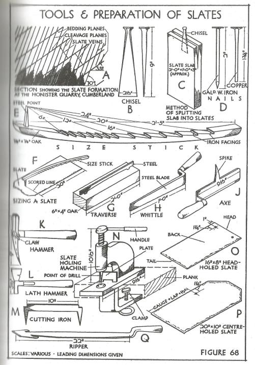
to give its maximum size with the minimum waste, and the slates are afterwards sorted into sizes.
