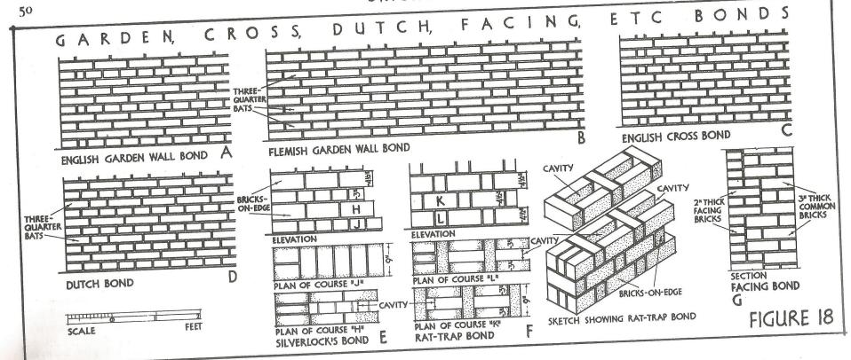
and occasionally for walls of cheap one-storied cottages. They can be employed effectively if their external faces are covered with vertical tiling (see p. 111, Vol. III). The best known brick-on-edge bonds are (a) rat-trap bond and (b) Silverlock's bond.
