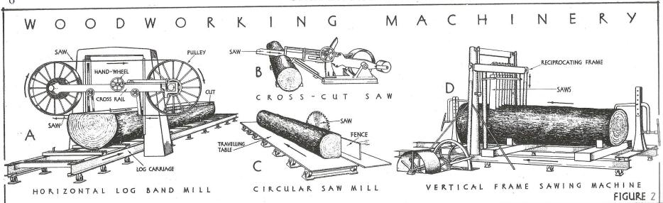
after they have been cut into suitable lengths. These include the (1) horizontal log band mill, (2) vertical log band mill, (3) circular saw mill, (4) horizontal log frame sawing machine, (5) vertical log frame sawing machine, (6) combined log and deal frame and (7) band re-sawing machine. The following is a brief description of these power-driven machines:—
