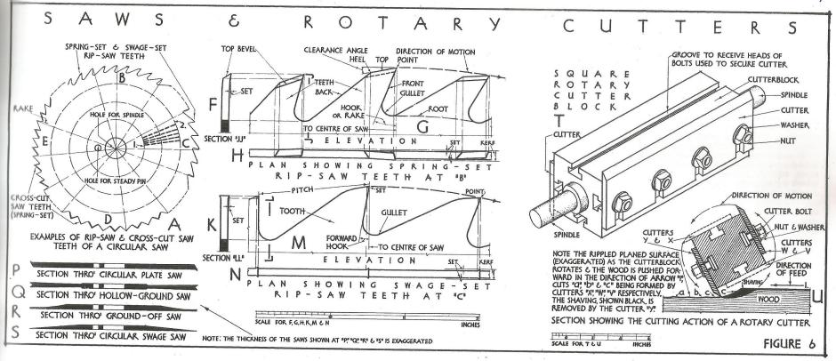
swage saw (see s) is tapered on one side from the rim towards the edge of the collar. They are either spring set or swage set. Both produce thin clean saw kerfs, and are used for cutting thin boards only, the ground-off saw being chiefly used for cutting boards from  $\frac{1}{16}$  to  $\frac{8}{3}$ -in. thick and the swage saw for sawing boards up to  $\frac{3}{4}$ -in. thick.
