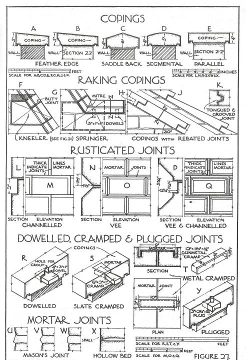
also be used (especially for securing quoin cornice stones) to resist any movement which tends to separate the joints (see p. 52).
