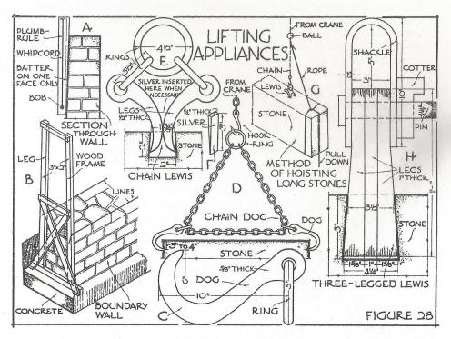
Chain Lewis.—This comprises three steel rings and two curved steel legs (see E, Fig. 28). The legs vary in size. The hole which is formed in the centre of the top bed of the stone is slightly dovetailed. If it is excessively dovetailed there is a tendency for the lewis to be pulled out owing to the legs bursting the stone during the lifting operation. The size of the hole varies from 2 to 3-in. deep; the 2-in. deep hole shown is about \(\frac{3}{4}\)-in. wide.
