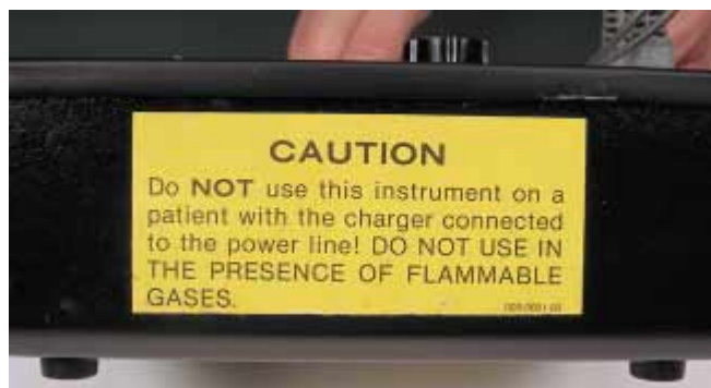
Figure 31-9 Warning Label on Electrical Equipment
