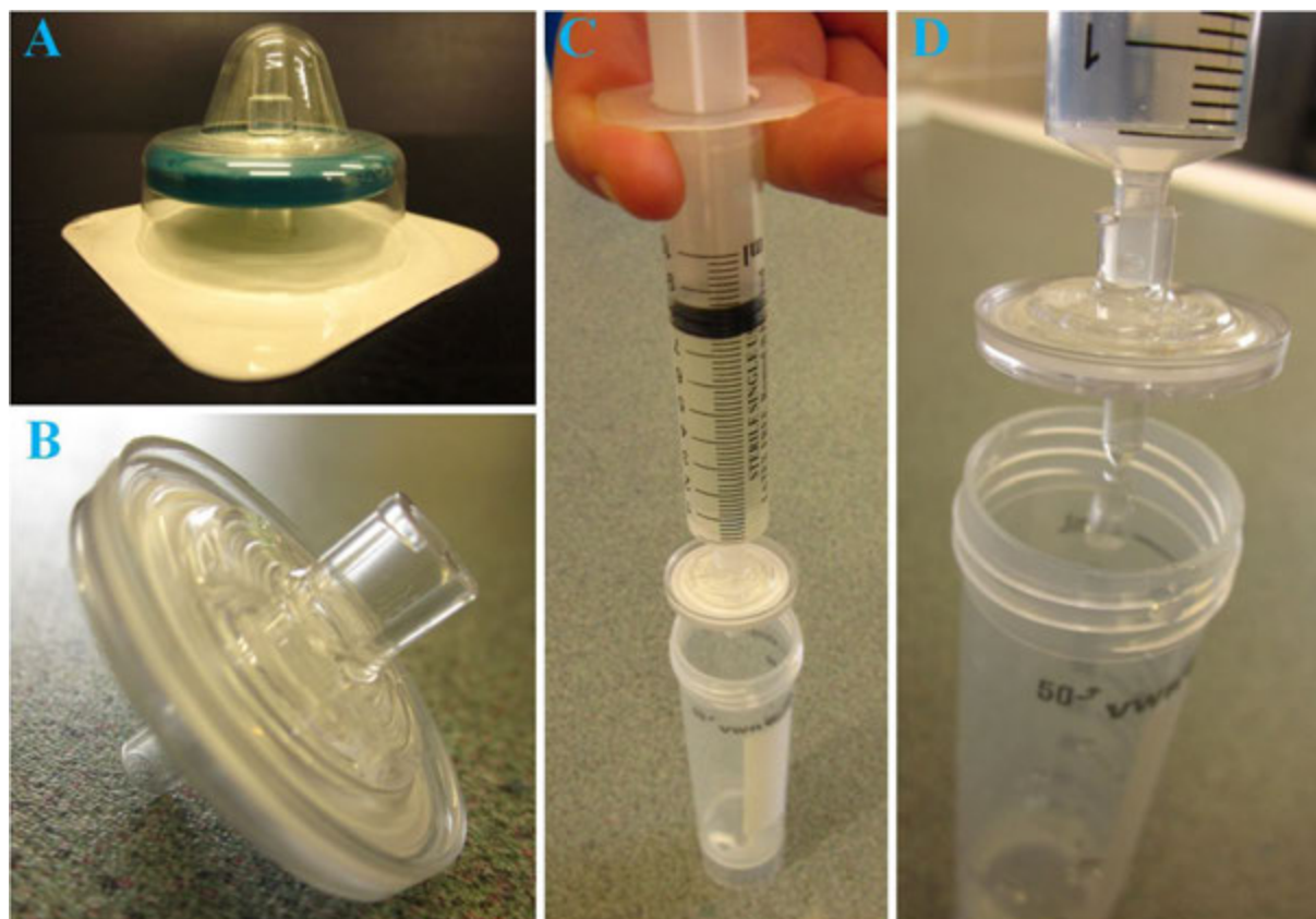
Figure 1.13. A, Sterile filter within its protective envelope. B, Close-up view of a sterile filter. C, Sterile filter fixed onto a syringe. D, Syringe-driven filtration.
