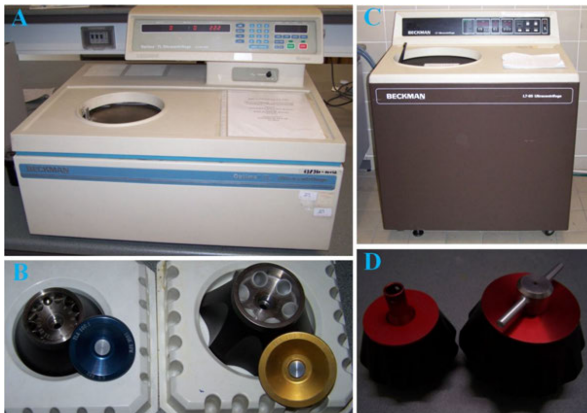
Figure 1.17. A, Micro-ultracentrifuge ( \text{RPM}_{\text{max}} = 100000 \text{ min}^{-1} , \text{RCF}_{\text{max}} = 300000 \text{ g} ). B, Rotors compatible with the micro-ultracentrifuge. C, Semi-preparative ultracentrifuge ( \text{RPM}_{\text{max}} = 70000 \text{ min}^{-1} , \text{RCF}_{\text{max}} = 350000 \text{ g} ). D, Rotors compatible with the semi-preparative ultracentrifuge.
