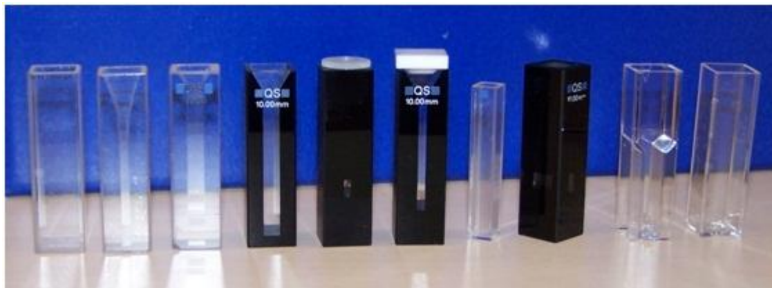
Figure 4.3. Cuvettes for holding samples. Cuvettes are generally made of glass, plastic or quartz. Quartz cuvettes are used when absorbance is measured at a wavelength under 320 nm, as glass and plastic absorb most of the light in this range. The path length is 1 cm in most cuvettes whose typical volume is around 1.5 mL. There are narrowed cuvettes for measuring smaller volumes. It is recommended to use narrowed cuvettes with darkened sides when measuring absorbance.
