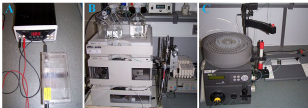
Figure 1.19. A, Power supply and buffer tank for gel electrophoresis. Gels are placed into the buffer tank. B, High-Performance Liquid Chromatography (HPLC) system. C, Fast Protein Liquid Chromatography (FPLC) system.
