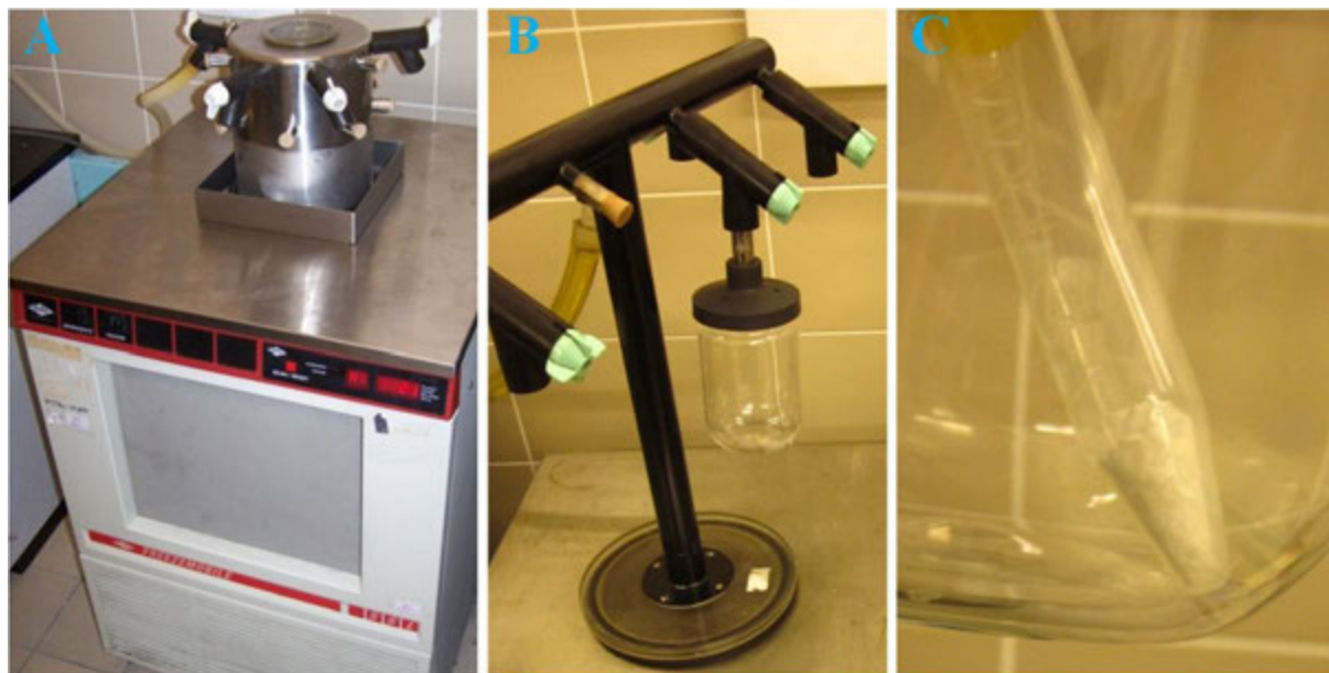
Figure 1.20. A, Freeze-dryer with a central vacuum chamber on the top. B, The central vacuum chamber can be expanded by tubes in order to enable the simultaneous handling of multiple samples. C, Freeze-drying of a sample within a Falcon tube.
