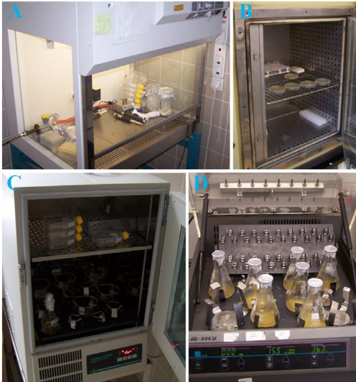
Figure 1.14. A, Laminar flow cabinet. B, Incubator (37°C) with bacterial cultures on agar plates. C, Incubator (37°C) with cultures of eukaryotic cells. D, Incubator (37°C) with a shaking platform for liquid cultures of E. coli bacteria (in Erlenmeyer flasks).
