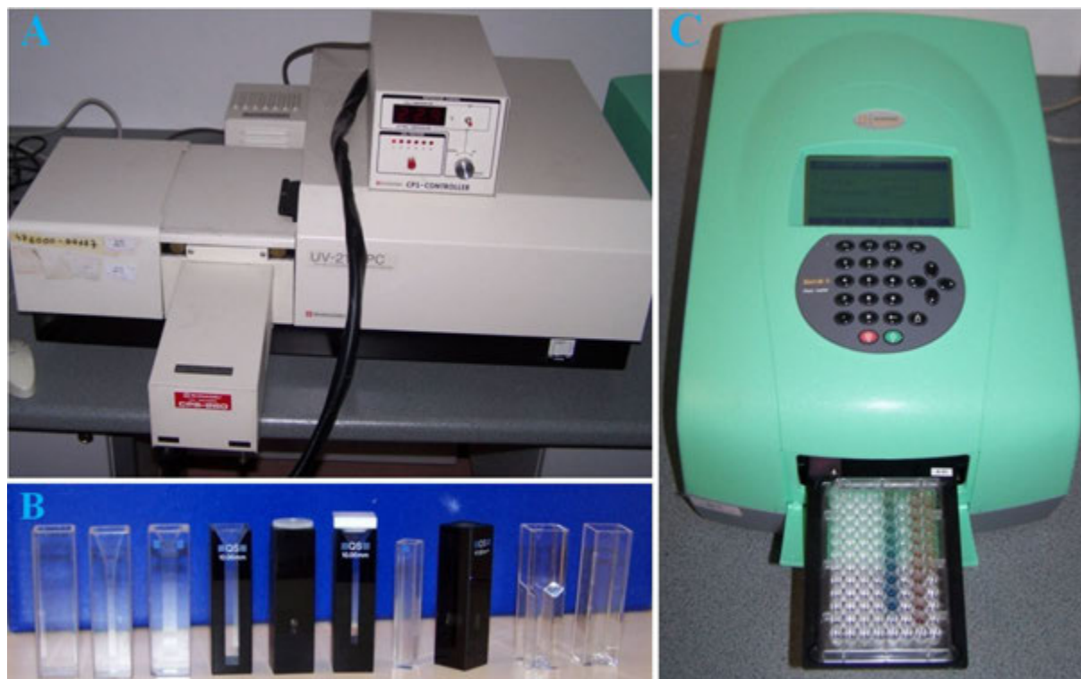
Figure 1.18. A, Spectrophotometer. B, Different types of cuvettes: photometric sample holders made of plastic, glass or quartz. C, Plate reader with samples loaded onto a 96-well microplate.
