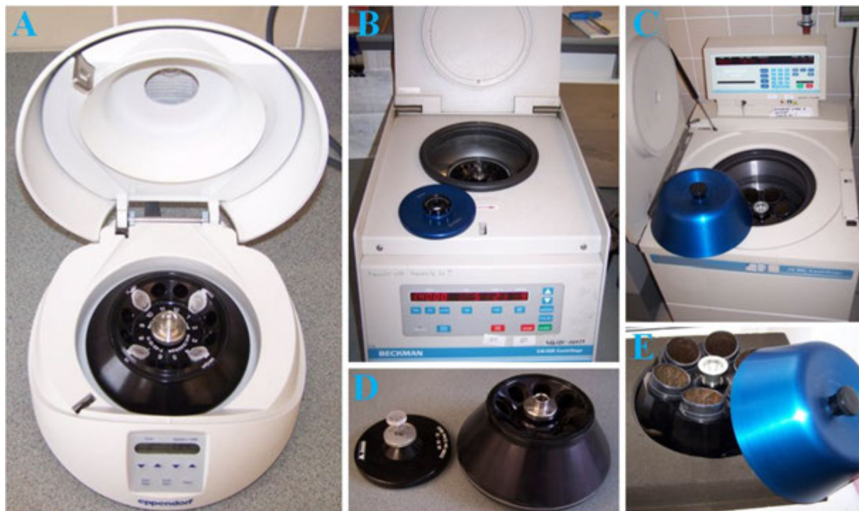
Figure 1.15. A, Bench-top Eppendorf centrifuge with samples arranged symmetrically around the axis of the rotor. B, Semi-preparative, refrigerated centrifuge with a rotor for Eppendorf tubes. C, Preparative, refrigerated centrifuge with a rotor for the handling of volumes up to 6 litres. D, Semi-preparative rotor with lid. E, Preparative rotor with lid.
