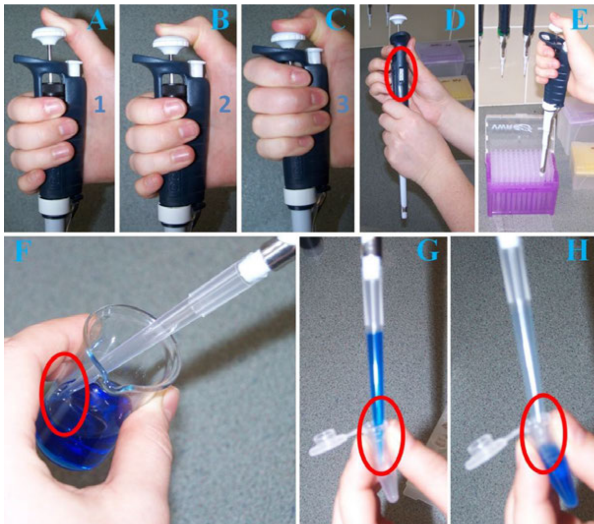
Figure 1.9. A-C, Three positions of the button of the pipette. D-H, Liquid handling with pipettes. D, Adjusting the volume. E, Fastening an appropriate tip. F, Drawing of the liquid. G, Transferring the liquid into an Eppendorf tube. H, Dispensing the liquid.
