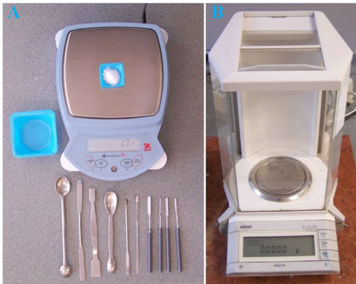
Figure 1.11. A, Top loading balance with disposable weighing dishes, laboratory spatulas and spoons. B, Analytical balance on a vibration-free surface.
