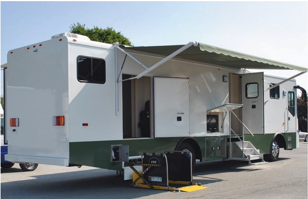
Fig. 21.5 Mobile health unit with wheelchair-accessible entrance. (Image from Matthews Specialty Vehicles. Reprinted with permission from RAD-AID International)
