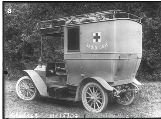
Fig. 21.1 Early use of mobile radiology during World War I, including mobile units with x-ray capability developed by Marie Curie to find bullets and shrapnel in wounded soldiers (a) and vehicles built to provide imaging access to various military medical installations (b)
