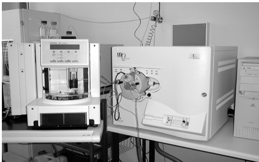
FIGURE 9 A Prince Technologies CE (Groton Biosystems, Boxborough, MA) interfaced to a Thermo Finnigan mass spectrometer.
