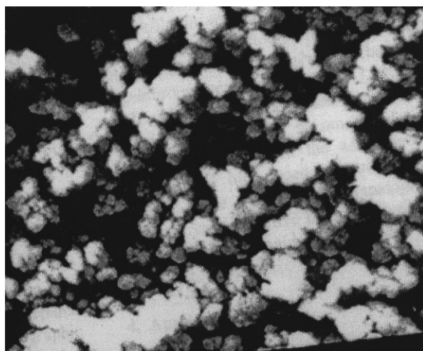
FIGURE 10 Scanning electron micrograph of the inner part of a methacrylate-based monolith. (Reproduced with permission from reference 59.)
