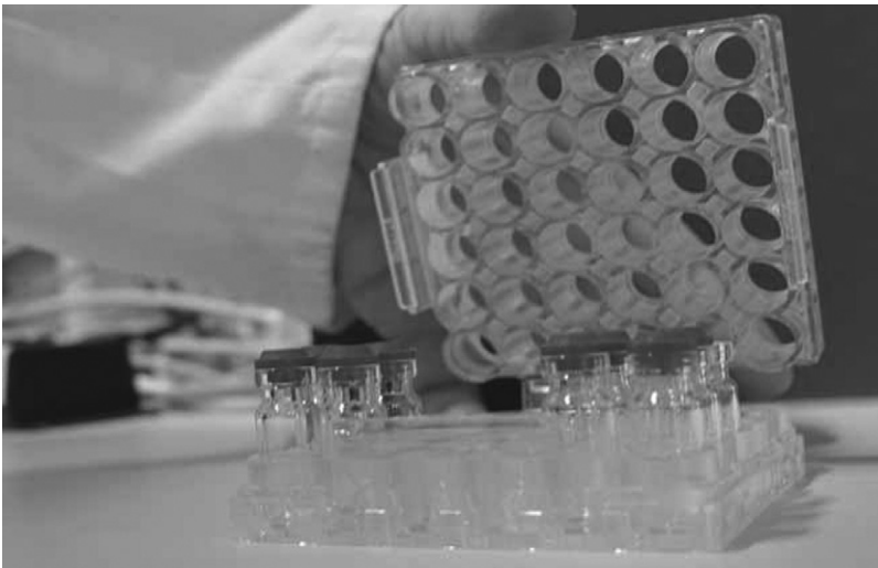
FIGURE 20 A way to prevent frequent system failure caused by punching of the electrode in the vial closure septum due to sticking of vials at the capillary interface block of the most frequently used QC performance Beckman MDQ CE system is the use of sandwich racks. The cover of these racks avoids vials coming out of the racks.
