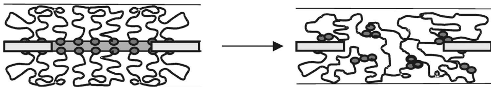
Fig. 6: Scheme of physical cross-linking of a suspended membrane of polymer chains with multiple head groups. Upon drying of the water core, which is initially present in the transferred membrane, the head groups aggregate and form physical cross linking sites.
