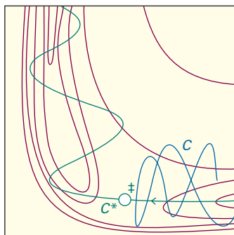
Fig. 24.21 An attractive potential energy surface. A successful encounter ( C^* ) involves high translational kinetic energy and results in a vibrationally excited product.
