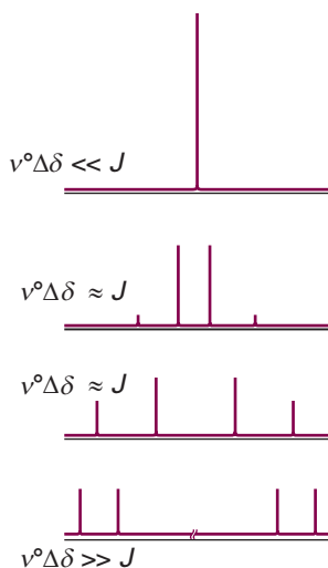
Fig. 15.25 The NMR spectra of an A_2 system (top) and an AX system (bottom) are simple ‘first-order’ spectra. At intermediate relative values of the chemical shift difference and the spin–spin coupling, complex ‘strongly coupled’ spectra are obtained. Note how the inner two lines of the bottom spectrum move together, grow in intensity, and form the single central line of the top spectrum. The two outer lines diminish in intensity and are absent in the top spectrum.
