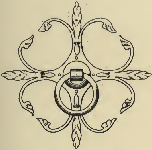
Closing Ring from Eye Church, Suffolk. 1/2 full size with details full size.
