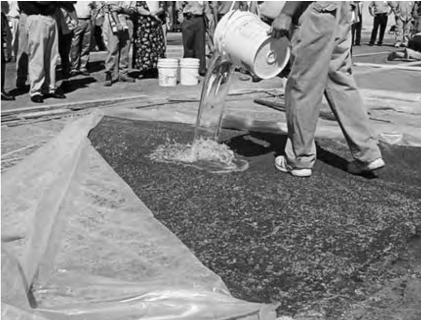
*Figure 2.11* Permeability of a pervious pavement demonstration project – Cleveland, Ohio (photo by author).
