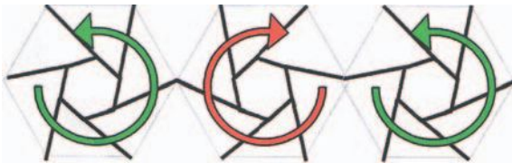
▲ 3.4 Single RF units with clockwise and anticlockwise beams.
