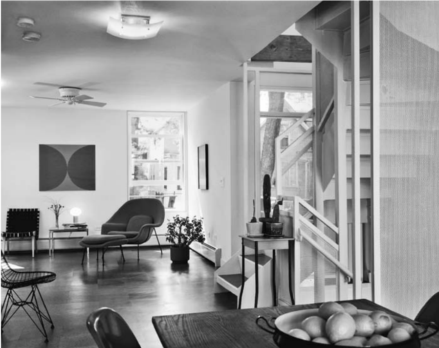
Window placement at F10 maximizes reflected light; the solar chimney includes a south-facing clerestory window that brings natural light to the house's core.
