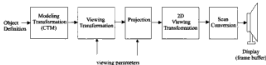
Fig. 8-11 A 3D graphics pipeline
