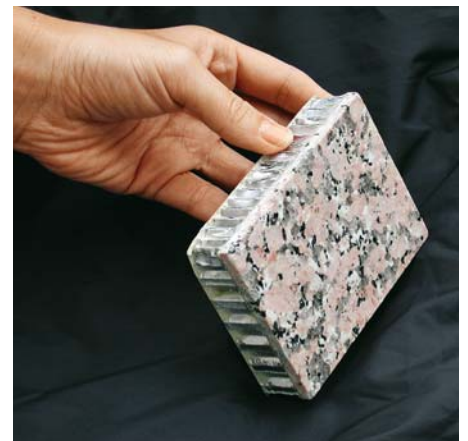
Stone faced composite panels with a thin layer of stone adhered to a honeycombed aluminum core has proven to be resistant to flexure, even after frost treatment in an aggressive environment.
