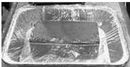
Testing of brick for efflorescence.
