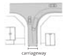
If footway edge follows the wide swept path of refuse vehicles and buildings are set back to maximise sight lines, a vehicle - oriented layout will result
