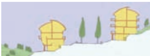
Orientate according to site contours
