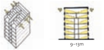
Cellular plan daylit (sidelit): Accommodates maximum variety of uses
