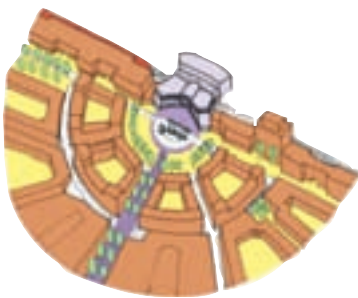
Public transport orientated development ensures that a mixed use community has a railway station or bus stop within walking distance at its heart
