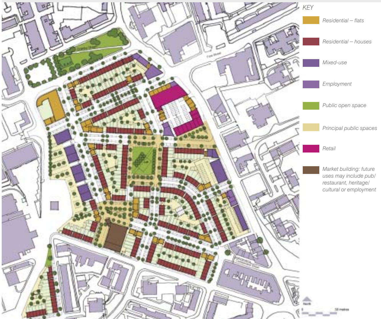
The masterplan for South Yard Enclave in Devonport, successfully combines over 450 high-quality homes, a community healthcare centre, new supermarket and shops, public open space, offices, managed workspace and the retention of the historic Market Hall.
