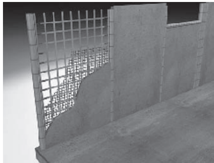
Figure 3. Grid wall system (Courtesy: Arch Daniel Romero).
