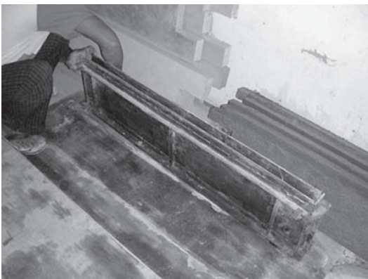
Figure 8. Steel moulding equipment for dry casting.
