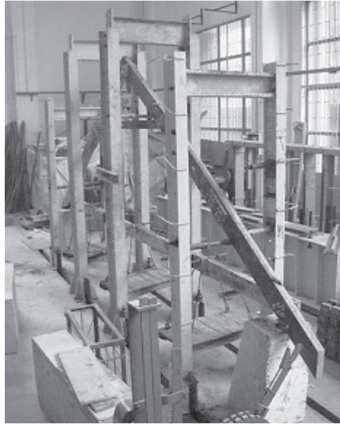
Figure 2. Laminated bamboo truss test at IBTCS.
