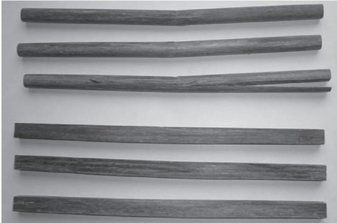
Figure 3. Failure mode of drift pin under bending stress. (upper: Round type, bottom: Square type)
