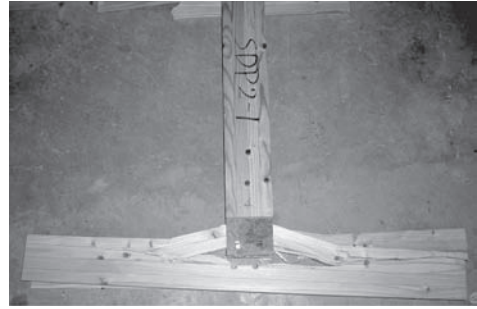
Figure 13. Failure mode of the double-board type.
