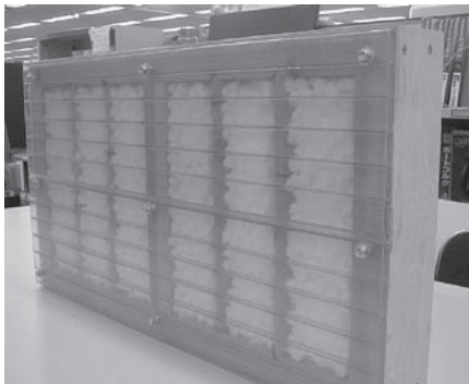
Photo 10. Bio plastic Insulation wall.
