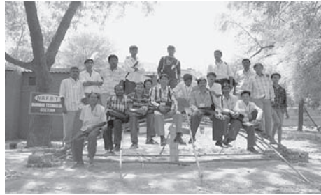
Figure 9. Bow arches (2 No.) before ferro-cementing, carrying human load of about 1 ton in a workshop.
