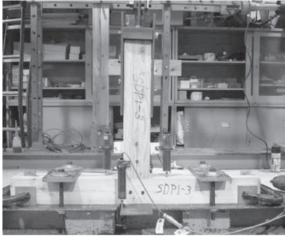
Figure 10. Set-up of the tensile test specimen.
