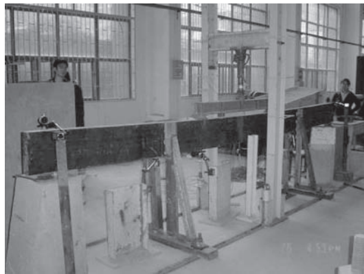
Figure 7. Full-scale bamboo girder beam test.
