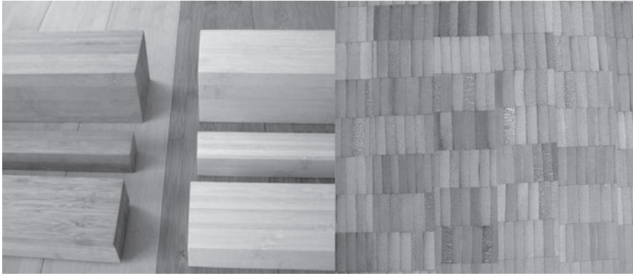
Figure 3. (left) Laminated Bamboo Lumber from one of the manufacturers in China and shipped to the US for many building finishing products (image courtesy of 4windsbamboo.com); (right) close up look of the bamboo lumber section that is a makeup of many strips laminated together.
