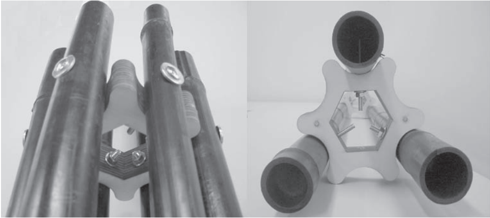
Figure 1. Research of utilizing bamboo in raw-form by developing bamboo bundling connections for stronger structural properties.
