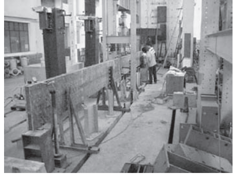
Figure 3. Setup for full-scale glulam girder testing.
