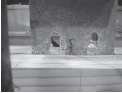
Figure 12. Failure mode of the single-board type.
