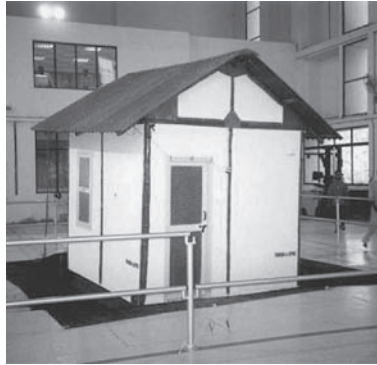
Figure 6. Bamboo House under shake table testing at CPRI, Bangalore.
