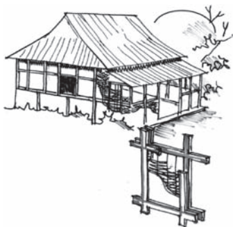
Figure 4. Typical Assam House (Wattle & daub, bamboo lath infill walls).
