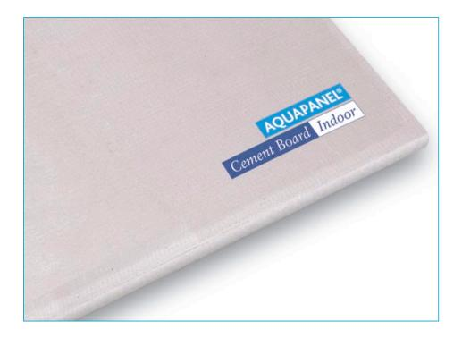
AQUAPANEL® Cement Board Indoor is a solid, durable tile backing board for interior use. It is made of aggregated Portland cement with coated glass fibre mesh embedded in back and front surfaces. The ends are cut square and edges are reinforced for extra strength (the EasyEdge<sup>™</sup>). The panel is 100% water-resistant and resistant to mould and mildew. It is non-combustible and has low installation costs.
