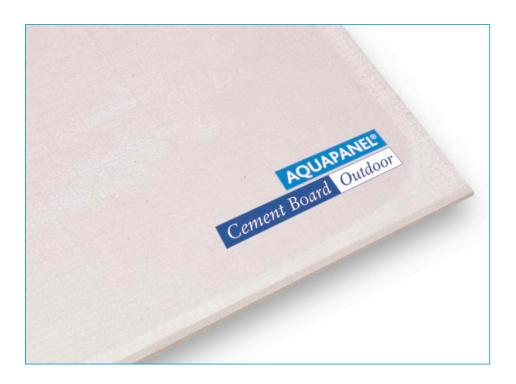
AQUAPANEL® Cement Board Outdoor is a robust, non-combustible building panel made of aggregated Portland cement with coated glass fibre mesh embedded in back and front surfaces. It offers all the benefits of a dry panel system with the strength of brick and block.
