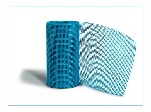
AQUAPANEL® Exterior Reinforcing Tape (33cm) is used to reinforce joints in exterior areas where a coat of paint is to be applied on the AQUAPANEL® Exterior Basecoat.
