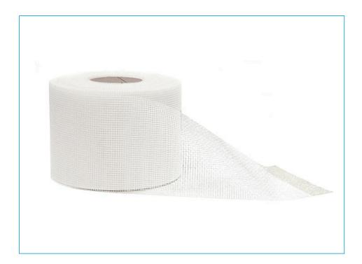
AQUAPANEL® Tape (10cm) is a glass fibre tape with an alkaliresistant coating. AQUAPANEL® Tape is used to reinforce joints on ceilings in interior areas and on walls and ceilings in exterior areas. It is embedded in the AQUAPANEL® Joint Filler – Grey.
